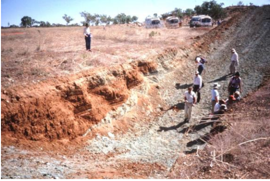
Figure 2. (a) Ellendale 9 lamproite in Western Australia is located within a field of more resistant lamproites that are barren of olivine. This commercial deposit, exposed in the bottom of the trench, was discovered by its magnetic signature as it lay hidden within a prominent field of lamproites much similar to the Leucite Hills in Wyoming. (b) A parcel of peridot gems from anthills near the Black Rock lamproite in the Leucite Hills. These are part of the >13,000 carat group collected from just two anthills. Note the excellent clarity of the faceted gems.
