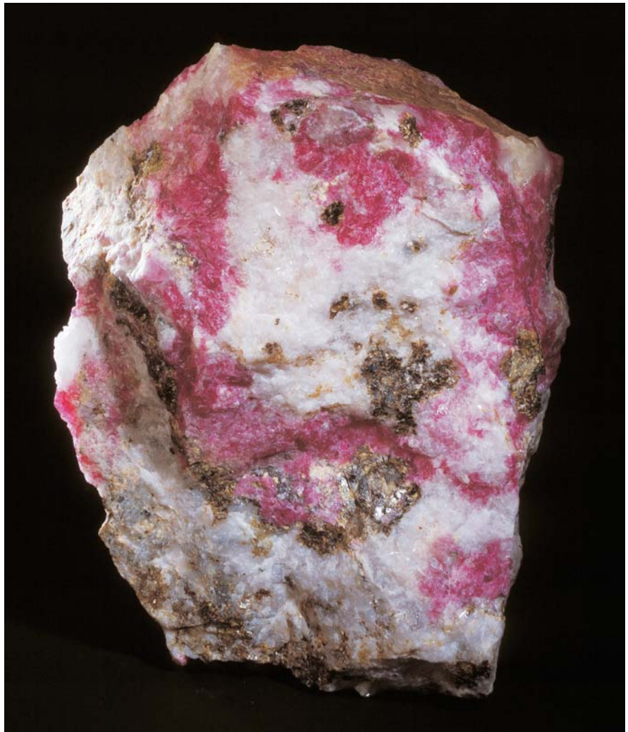
Below: Rough sample of tugtupite in vein with white albite and brown spahlerite from the Narsaq area. Size of sample: 8 x 10 cm.
