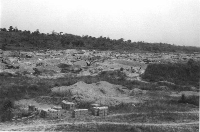
Plate 3.5 Overview of dug out pits where overburden can be haphazardly thrown on top of virgin land, Kono District, 2003
