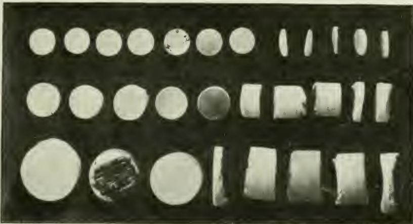
FIG. 2.—Blanks of various sizes and thicknesses as cut from the shell and before submission to the "backing" process. (See p. 74.)
