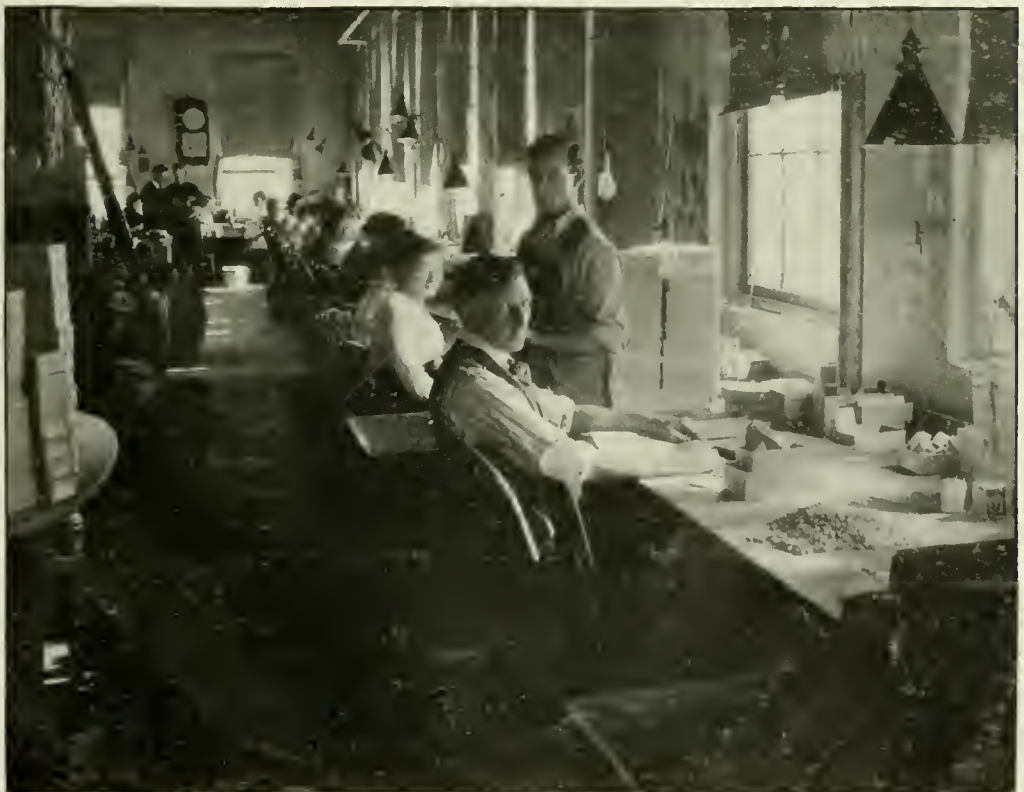
FIG. 2.—The sorting room, in which skillful operators classify buttons into 40 grades. (See p. 77.)
