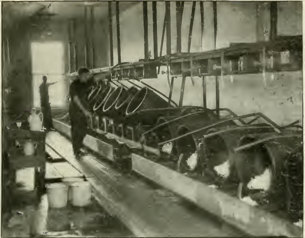
FIG. 1.—The churns, with buttons receiving polish by the use of acid and steam. Note the funnels from which acid solution drips into the churns. (See p. 77.)
