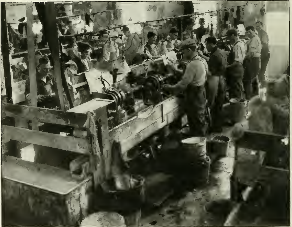
FIG. 2.—The cutting room, where blanks are cut from the raw shells. (See p. 72.)
