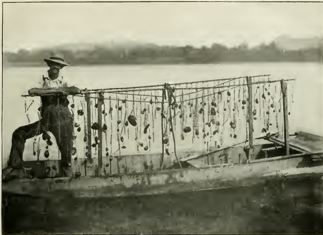
FIG. 1.—Bar and crowfoot outfit for taking mussels, consisting of john boat, two bars with crowfoot hooks, and the "mule" (lying on stern of boat). (See p. 46.)
