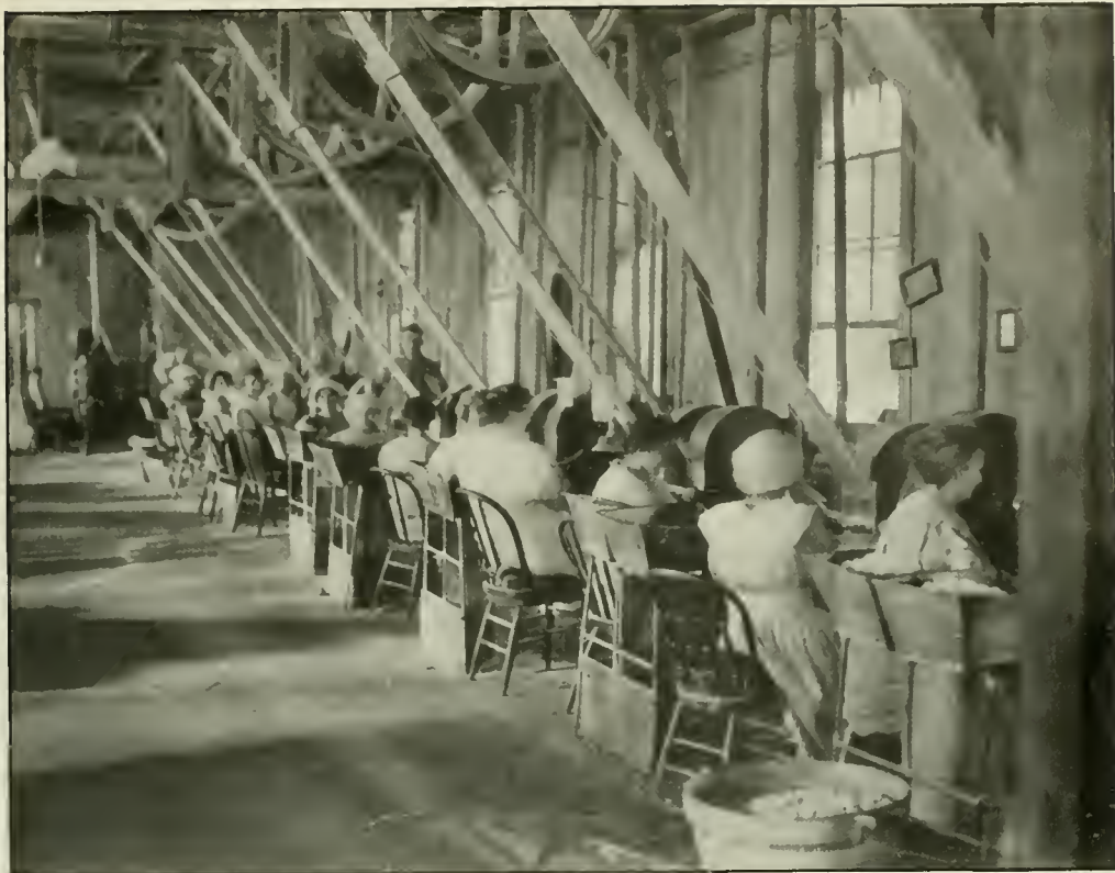
FIG. 1.—The belt grinders, where blanks are brought to uniform thickness. (See p. 75.)
