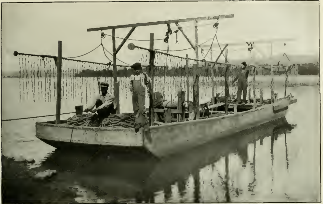
FIG. 1.—Barge with long crowfoot bars, employed on the Ohio River. Note rollers set on ends of bars to facilitate movement over the bottom. (See p. 51.)
