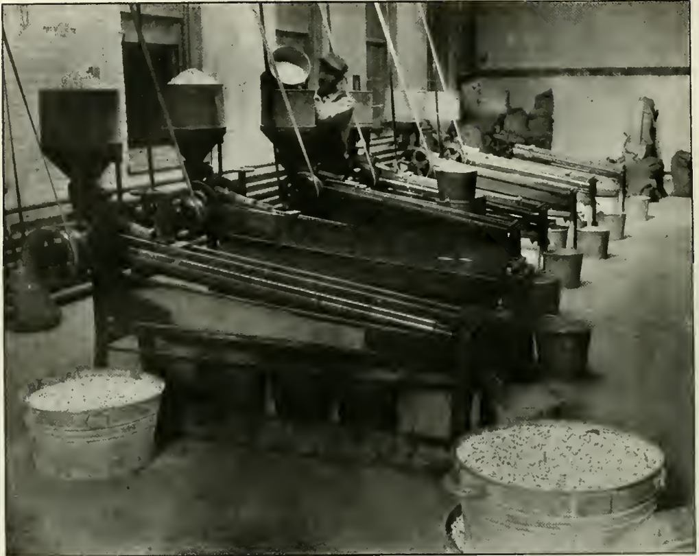
FIG. 1.—Blank classifiers for separation of blanks according to thickness. (See p. 74.)
