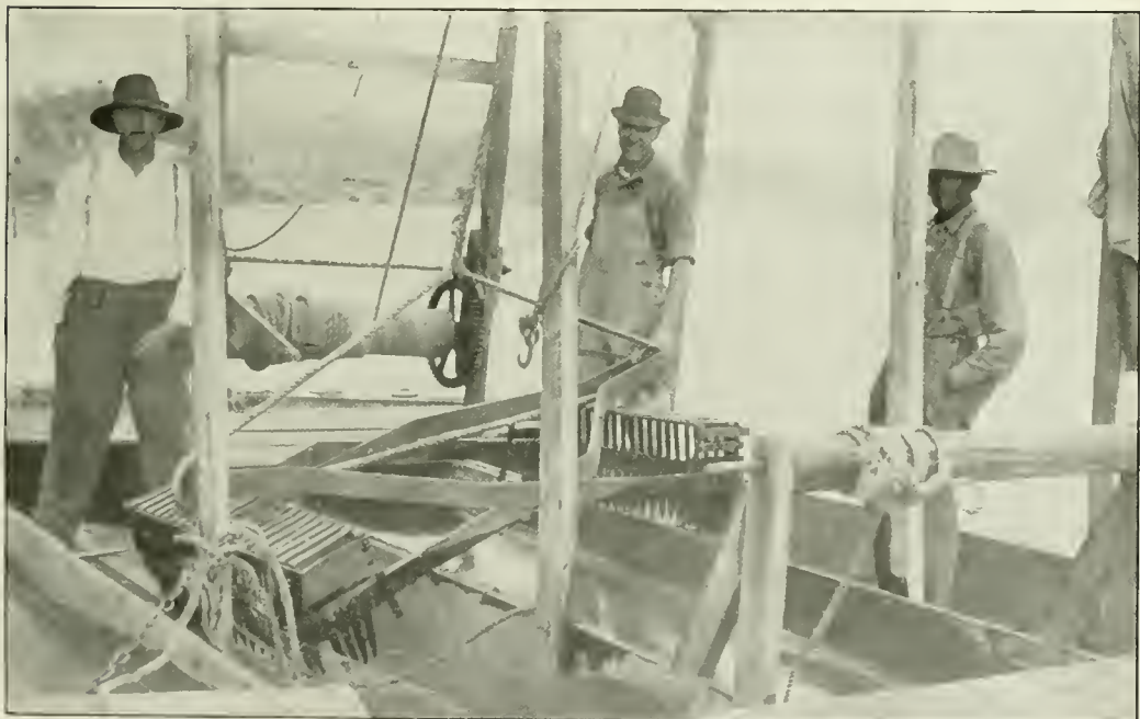
FIG. 2.—The dredge resting on gunwales of two boats forming the catamaran from which it is operated. (See p. 57.)
