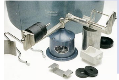
In centrifugal casting the mechanism spins, throwing the molten metal into openings in the plaster.
