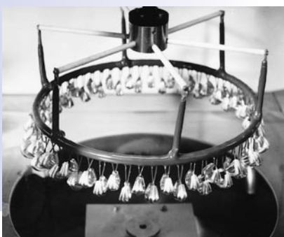
During electroforming, precious metal is deposited on wax forms suspended in a solution. Later the item is drilled and the wax melted and removed.
