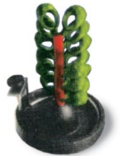
In centrifugal casting the mechanism spins, throwing the molten metal into openings in the plaster.
