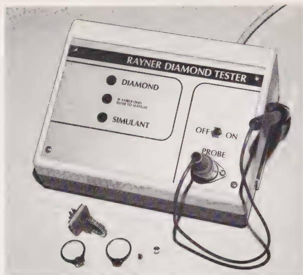
Figure T.3 The Rayner Diamond Tester distinguishes diamond from diamond simulants by detecting its high thermal conductivity. (Gemmological Instruments Ltd.)
