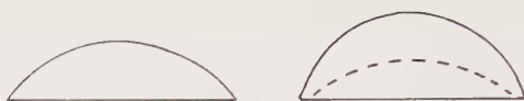
Figure C.1 Profile of the cabochon cut. Stones are sometimes hollow-cut (as shown on the right) to lighten their colour.
