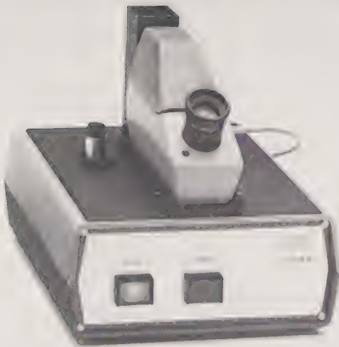
Figure R.3 The Rayner Dialdex critical-angle refractometer (top) is fitted with a calibrated control in place of a calibrated internal scale. (Gemmological Instruments Ltd.) The Kruss ER602 extended-range refractometer (bottom) uses a heated strontium titanate measuring prism. The bottle of thermo-plastic contact paste is heated to liquid temperature (40 °C) in a special socket on the control plinth. A sodium light source is fitted at the rear of the plinth. R.L. of the contact paste is 2.22, and the range of the refractometer is 1.79-2.21.
