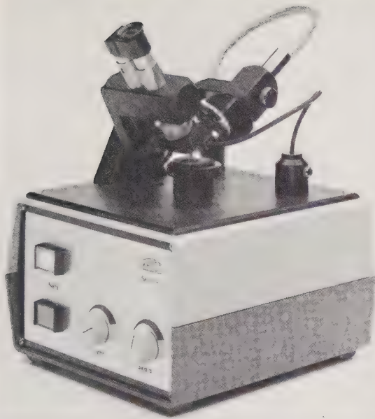
Figure S.4 A unit combining a variable-intensity self-contained light source, a colour filter disc and a prism-type wavelength spectroscope. (Krüss)
