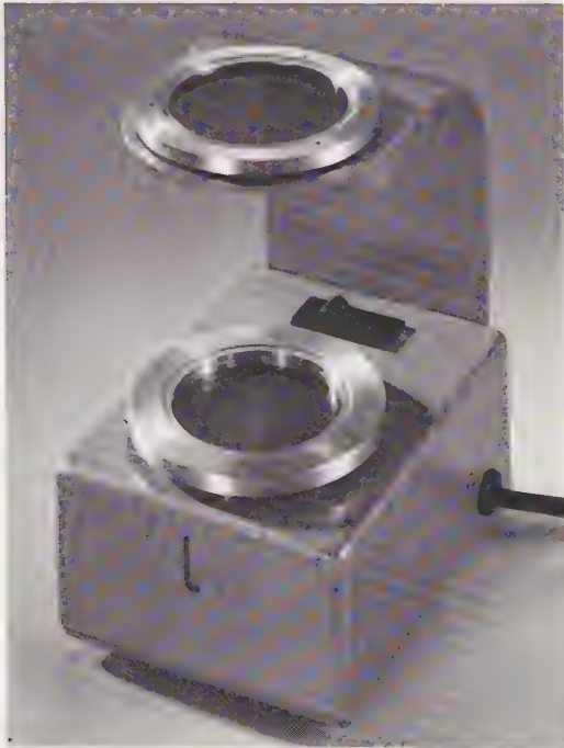
Figure P.3 The Rayner polariscope. (Gemmological Instruments Ltd.)
