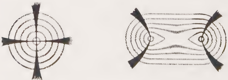
Figure 1.3 The interference figures seen (left) in a uniaxial stone, and (right) in a biaxial stone.
