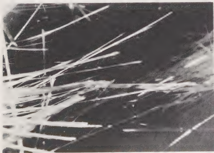
Figure A.2 Acicular rutile inclusions in quartz.
