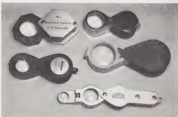
Figure H.1 A range of hand lenses.
