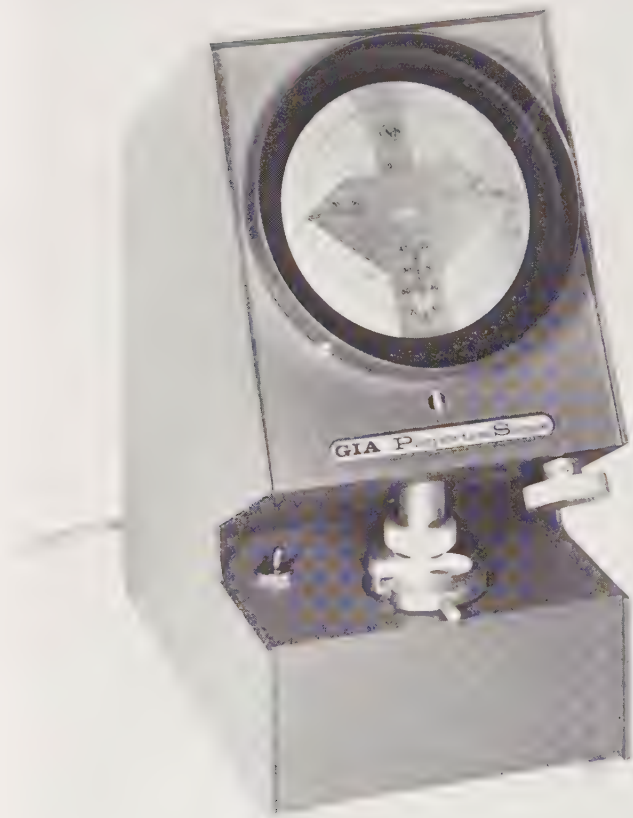
Figure D.3 The GIA ProportionScope is used to check the proportions and angles of a brilliant-cut diamond's crown and pavilion.
