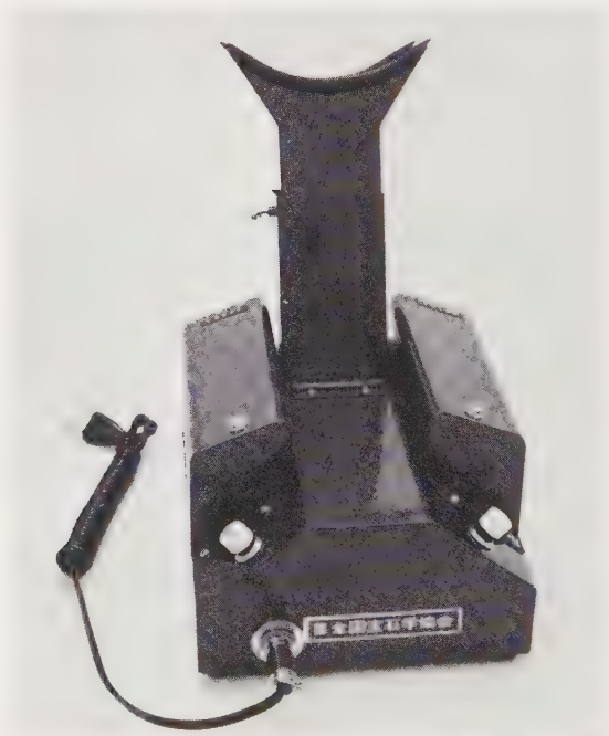
Figure U.3 A dual-range (LW, SW) combined ultra-violet lamp and viewing cabinet. (GAAJ/Gemmological Instruments Ltd.)
