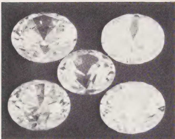
Figure L.4 Five diamond simulants photographed at an angle to illustrate the 'light spill' test. The centre stone is a YAG, and shows the greatest light leakage from its pavilion facets due to its relatively low R.I. (1.83). The top left stone is a GGG (1.97), top right is a lithium niobate (2.25), bottom left is a cubic zirconia (2.16) and bottom right is a strontium titanate (2.41) which, like diamond (2.42) shows no light leakage.
