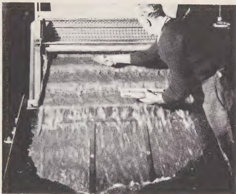
Figure G.4 Removing individual diamonds from a grease table in Kimberley, South Africa. (De Beers)
