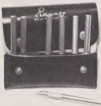
Figure H.2 A set of seven hardness pencils. (Rayner/Gemmological Instruments Ltd.)
