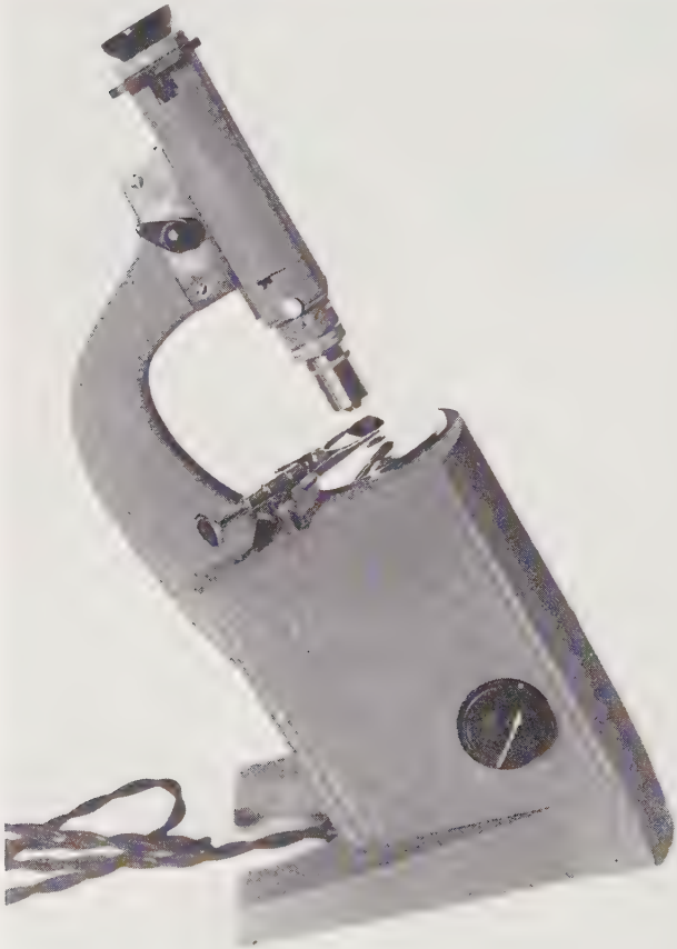
Figure G.5 The Gübelin jewellers' spectroscope with built-in wavelength and specimen light sources. (Gübelin)
