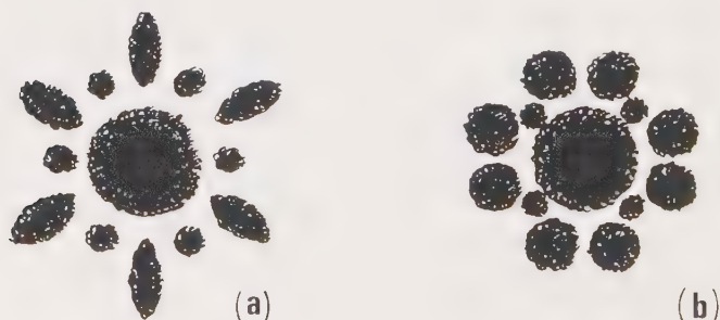
Figure L.2 The hexagonal Laue diffraction pattern produced when a narrow beam of X-rays penetrates a natural pearl is shown at (a). With a cultured nucleated pearl, both the hexagonal and the four-point pattern, as shown at (b), can occur, depending on the orientation of the bead.
