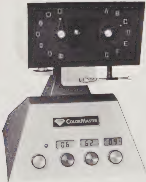
Figure V.2 The GIA ColourMaster is a visual colorimeter which can be used to match and code coloured stones for hue, brightness and colour saturation. (Gem Instruments Corp.)
