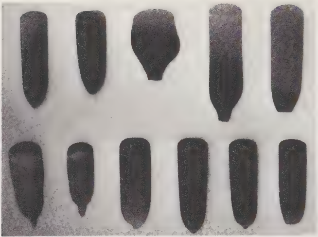
Figure B.4 Synthetic corundum and spinel boules grown in a Verneuil furnace.
