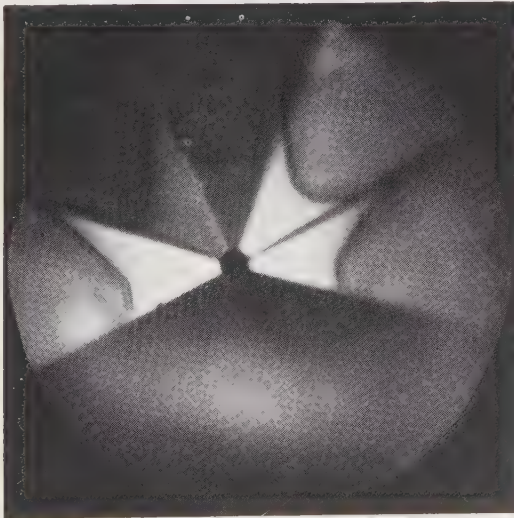
Figure U.2 The 'umbrella' effect as seen round the culet of a cyclotron-treated diamond.
