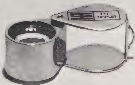
Figure T.7 The components of a triplet hand lens.
