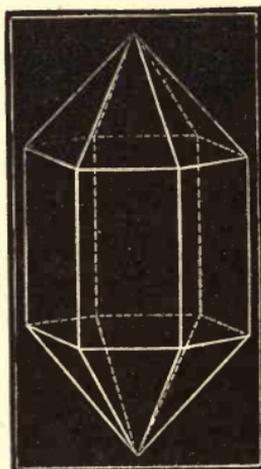
Fig. 68.—Most ordinary form of Quartz Crystals.
