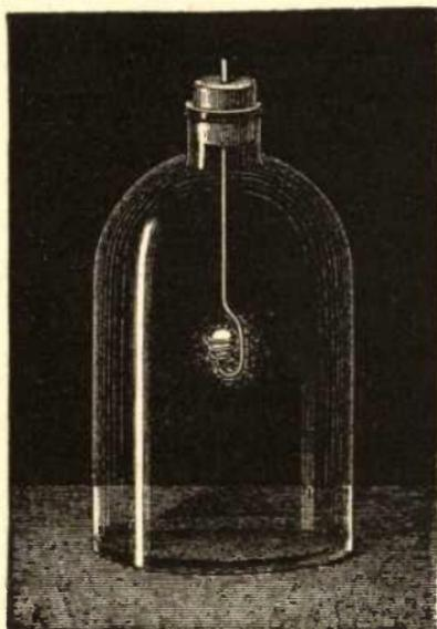
Fig. 33.—Combustion of the Diamond in Oxygen.
