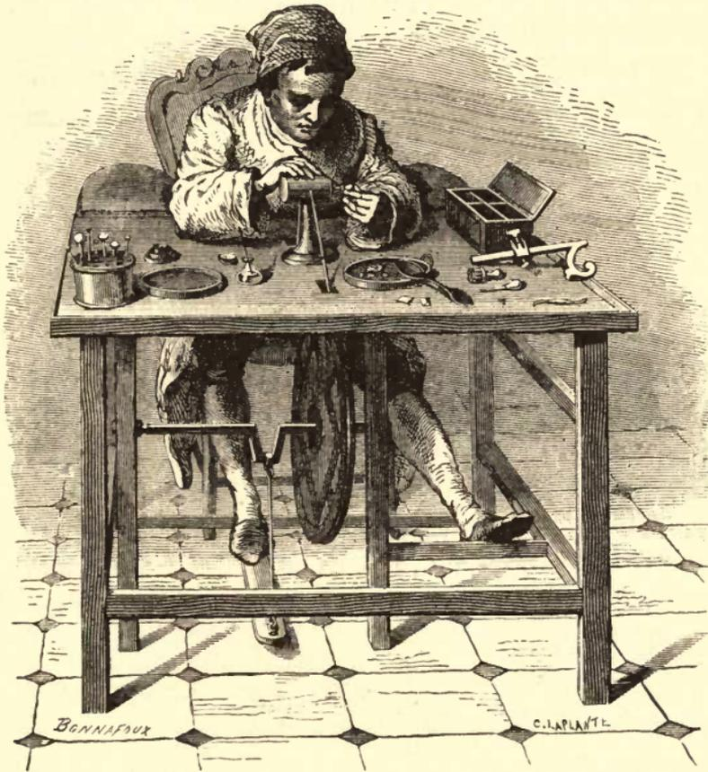
Fig. 123.—The Lathe at work.
