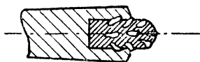
FIG. 162.—Diamond chips embedded in a tungsten or tungsten carbide matrix; tool used for truing purposes
