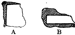
FIG. 148.—A and B. Cutting industrial diamonds according to the shape of the rough stone is not a satisfactory method
