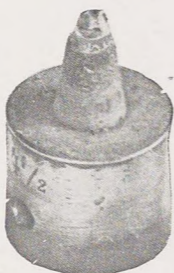
Diamond cemented on spindle for cutting.
