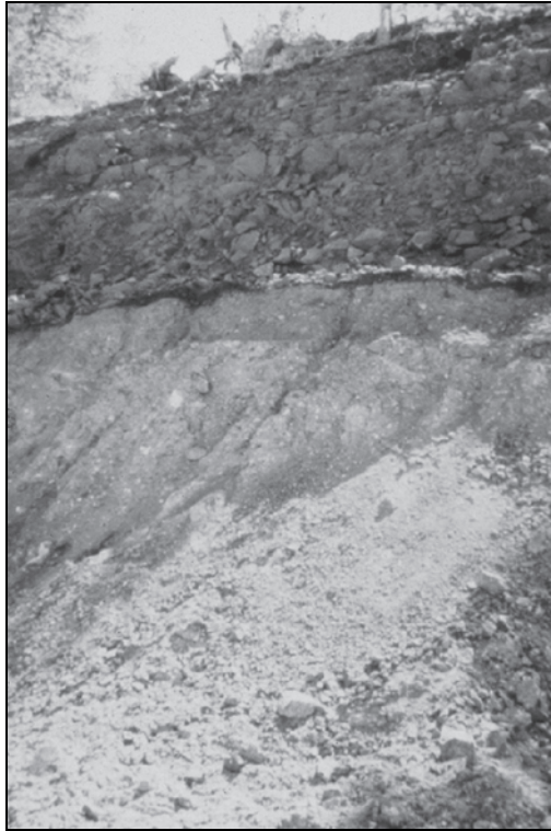
FIGURE 6.7 High wall at Kelsey Lake mine in Colorado with kimberlite breccia lying under a thin crust of granite
