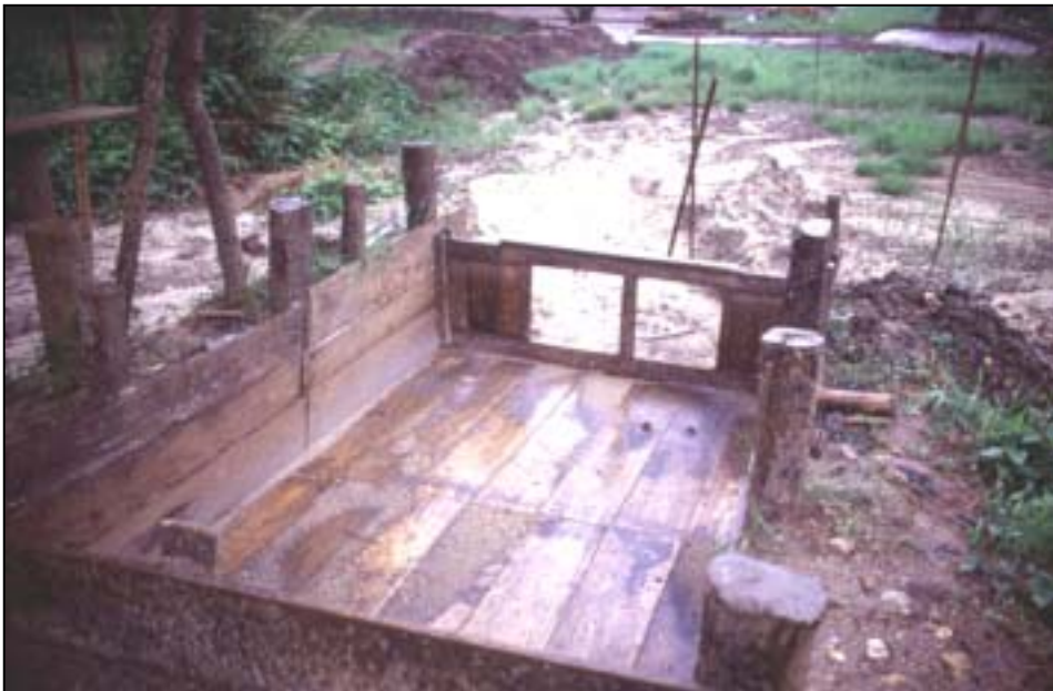
Plate 8: Sluice box used for processing clay rich sediments
