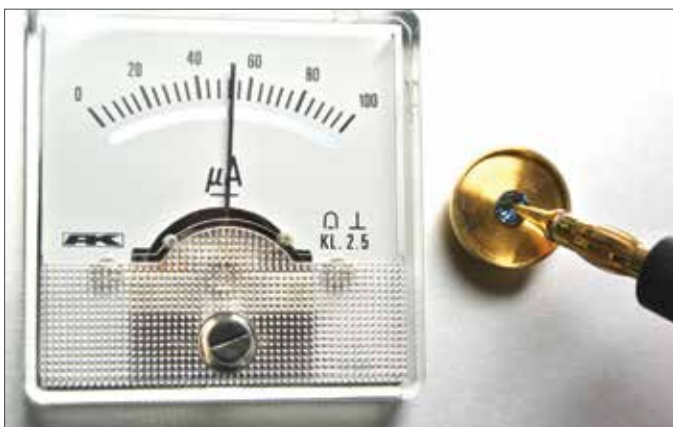
Fig. 4: This HPHT synthetic blue diamond tested by an electrical conductance meter reveals considerable electrical conductance. Natural blue diamonds would show similar behaviour. The new blue CVD diamonds have been found to be non-conductive.
