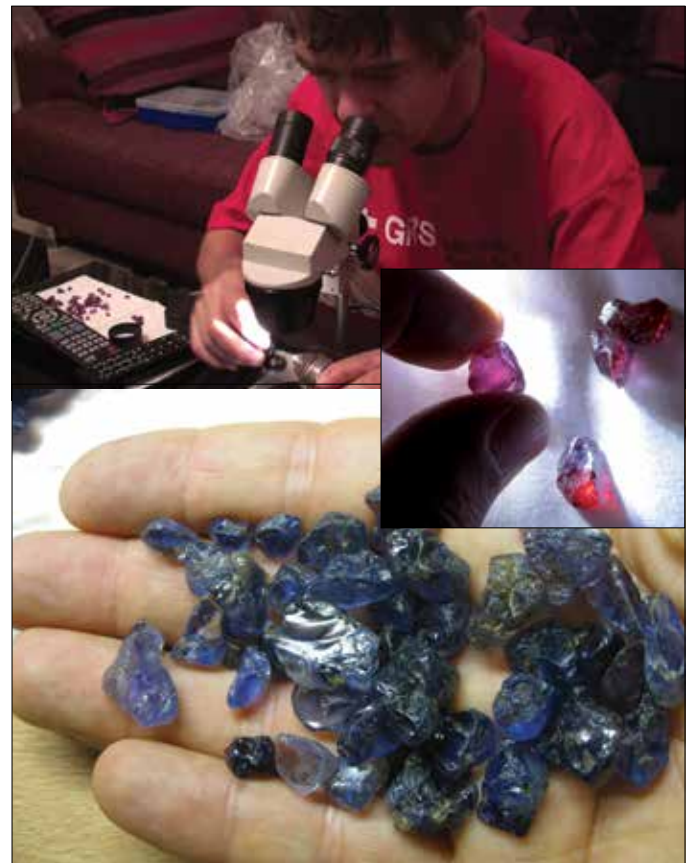
Fig. 24: Peretti works with a portable microscope to search through lots of rubies and sapphires of dealers in Ambatondrazaka. The presence of illmenite, zircon clusters, blue color zones and absence of silk make these rubies very easily distinguishable through microscopical examination from all other ruby localities, even from the counterparts found in Winza (Tanzania). The same is true for the sapphires that contain large negative crystals accompanied by secondary fluid feathers, isolated zircon crystals, black illmenite inclusions, oriented pargasite needles and the general absence of silk (Lit. 2).
