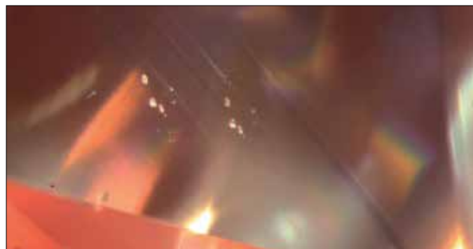
Fig. 5c: A blackish layer in a PDC CVD-grown pink diamond is accompanied by whitish particles and transparent crystals (HRef-0172, 0.50ct, 100x, fiberoptic, L.H.)
