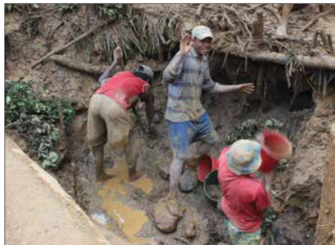
Fig. 12: Miners are digging under the trees to reach a secondary alluvial mining deposit with boulders of gneiss, amphibolite, gabbro and quartzite.
