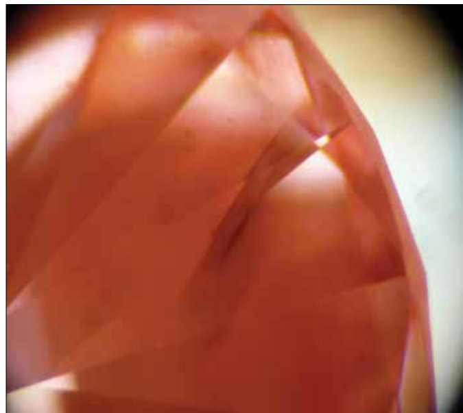
Fig. 5a: Blackish irregular clouds are found in this CVD-grown pink diamond from PDC (HRef0161-2)
