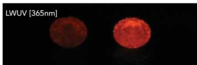
Fig. 9a-b: Synthetic HPHT-grown pink diamond and a brownish-pink CVD-grown diamond in day light and their fluorescence colors in Long Wave Ultraviolet (LWUV) light. Note the very strong pinkish orange fluorescence of the CVD-grown PDC diamond and strong orangy red fluorescence of HPHT-grown pink diamond caused by irradiation.
