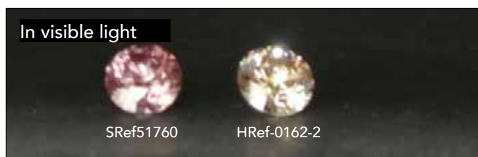
Fig. 9a-b: Synthetic HPHT-grown pink diamond and a brownish-pink CVD-grown diamond in day light and their fluorescence colors in Long Wave Ultraviolet (LWUV) light. Note the very strong pinkish orange fluorescence of the CVD-grown PDC diamond and strong orangy red fluorescence of HPHT-grown pink diamond caused by irradiation.
