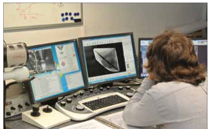
Fig. 5: A CVD blue diamond was exposed to an electron beam at low vacuum conditions in an Environmental Scanning Electron Microscope (Zeiss Evo 50 SEM) and a variable pressure secondary electron detector (VPSE) was able to produce images of differences in the charges located within the diamond (SEM-CC image), revealing details of the growth features. Operator PD Dr. Alfons Berger (in the picture). Results see Fig. 10-12.
