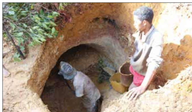
Fig. 15: Miners digging deeper into the alluvial bed to reach the gem-bearing layers. These layers are carried away with baskets to the washing place.
