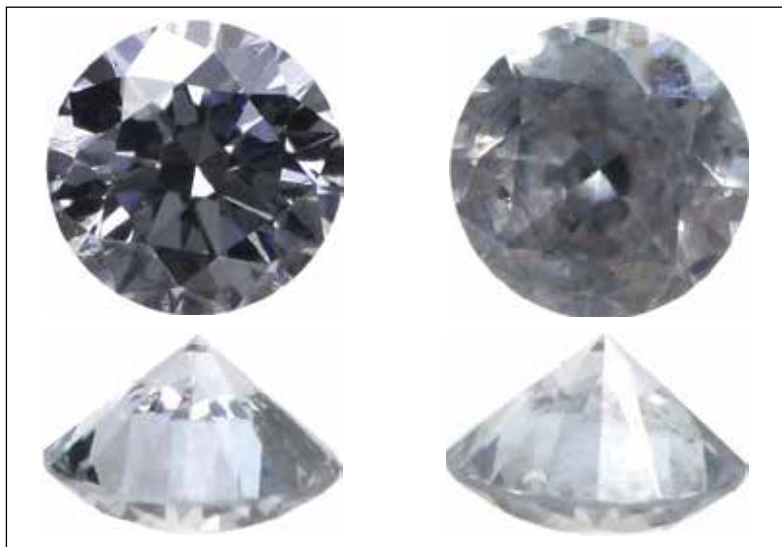
Fig. 19: 0.11ct Fancy grey-blue CVD grown diamond before (left) and after heating in air (right)
