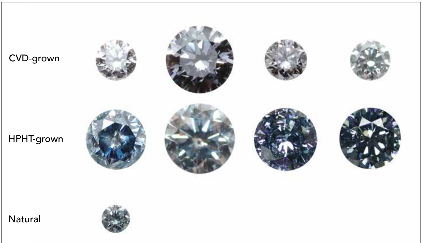
Fig. 3: These faceted synthetic blue diamonds were tested for this report: four CVD diamonds grown by Orion PDC (on top), four synthetic HPHT-grown diamonds from Chatham, AOTC, Tairus (middle), and one natural blue diamond (bottom). One HPHT crystal is not shown. Color and carat weights of these stones range from light blue to intense blue, and from 0.30 to 0.65 carats respectively.
