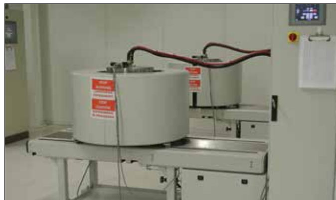
Fig. 2a: This HPHT-diamond laboratory of Ziemer Swiss Diamond Art AG (Port, Switzerland) shows a recent example of an upcoming factory producing lab-grown diamonds by BARS split sphere technology. Compare with CVD-diamond factory (Part A, Fig. 1[12])
