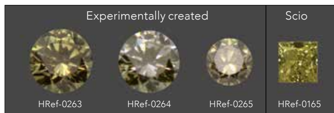
Fig. 13: Overview of all tested samples from left to right. The first three samples are the experimentally created, multistep treated CVD-grown yellow diamonds.
