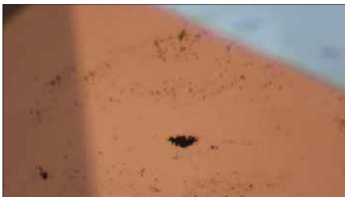
Fig. 6a-b: Black inclusion in a CVD synthetic diamond from Scio Diamond is assumed to be non-diamond carbon.
