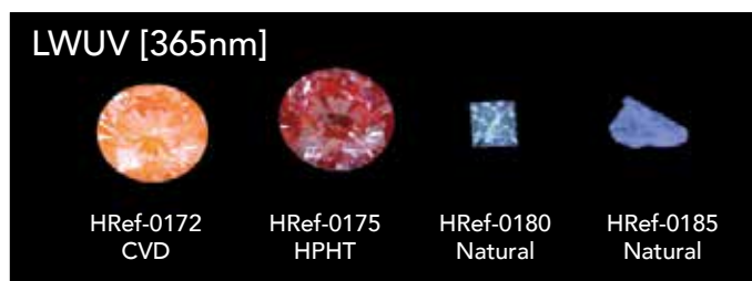
Fig. 8a-b: Comparison of fluorescence of synthetic and natural pink diamonds in Long Wave (LWUV) and Short Wave (SWUV) ultraviolet light. Note that a huge variety of color can be seen in fluorescence, blue typical for natural pinks, LW being stronger than SW. Synthetic pink diamonds show the same fluorescence in LWUV and SWUV in comparison to their natural counterparts.
