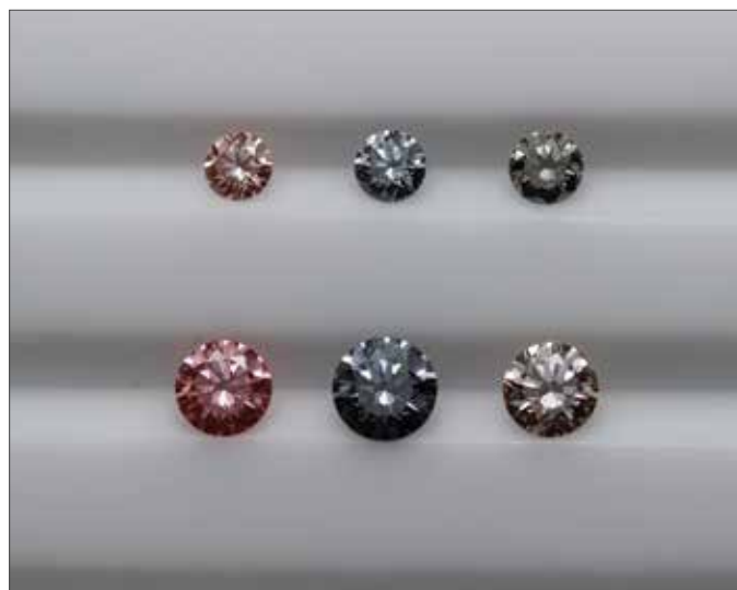
Fig. 2a: These CVD-grown diamonds produced by Orion PDC exhibit various tones of pink and blue color. CVD diamonds produced by Scio Diamond Technology USA, are yellowish brown.
