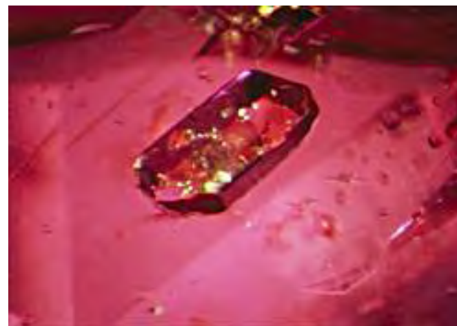
Light yellow apatite crystals in a corundum from Umba Valley, Tanzania; 25x.
