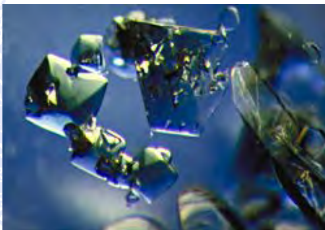
Spinel octahedra in a blue sapphire from Sri Lanka; 25x.
