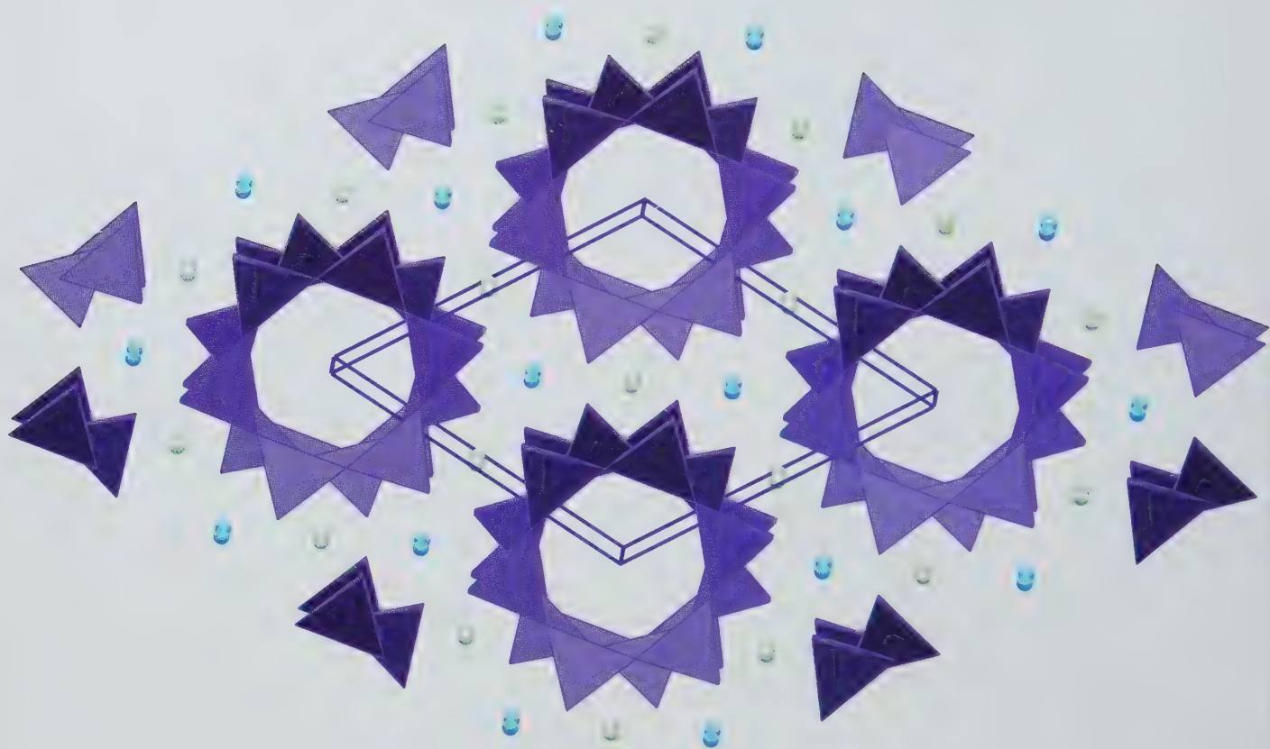
Figure 6. Crystal structure of beryl, viewed just off the z-axis or [0001], emphasizing the rings of \text{SiO}_4 tetrahedra enclosing hollow channels, octahedrally coordinated Al (pale blue balls) and tetrahedrally coordinated Be (pale green balls with wire bonds). Blue lines indicate the unit cell.
