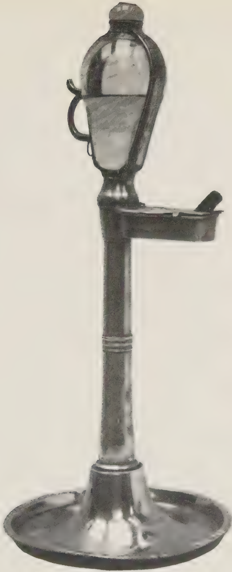
18th century north German oil clock. The glass reservoir is graduated from 8 pm to 7 am to show the hours of the night by the quantity of unburnt oil
