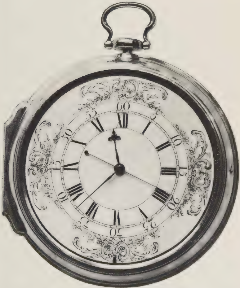
Harrison's number 4 chronometer. Only 5 inches in diameter, it has a single balance wheel and the escapement used is a much improved modification of the verge
