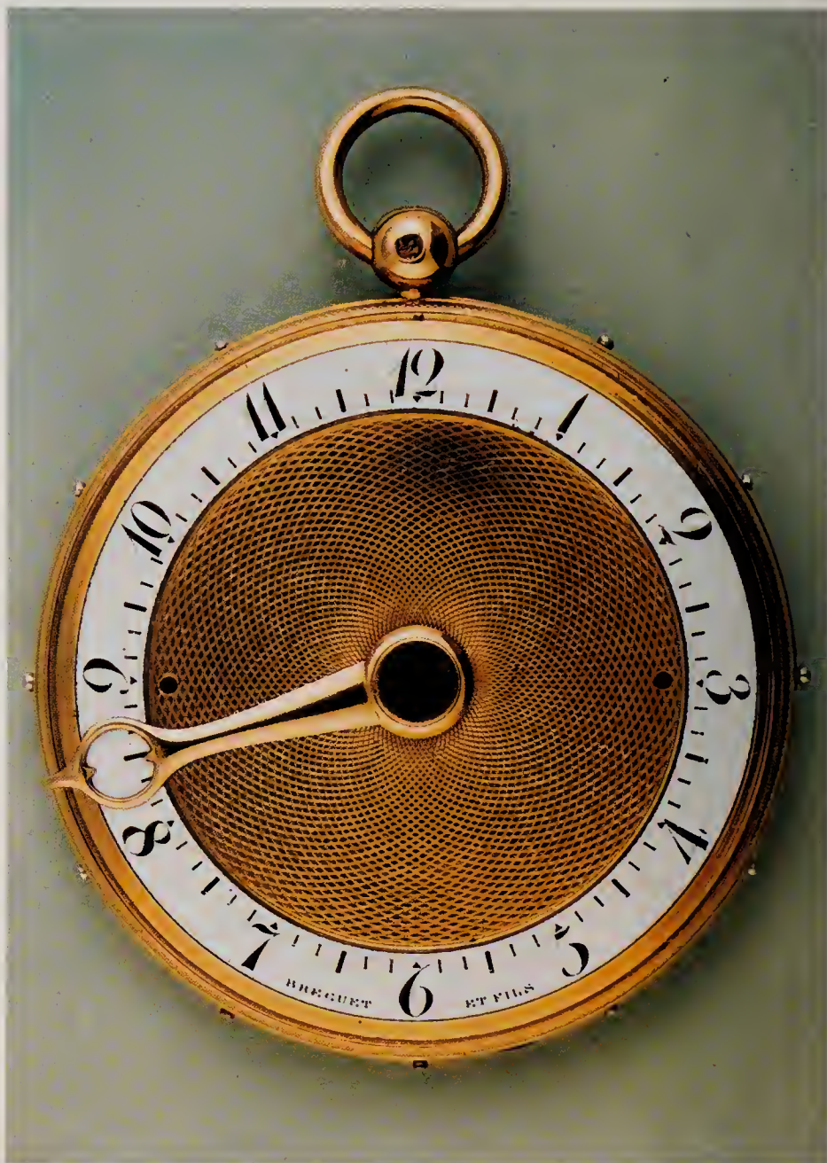
Above: A Breguet montre à tact with a cylinder escapement in a gold case. Turning the hand until it stopped indicated the time in the dark or to a blind person.
