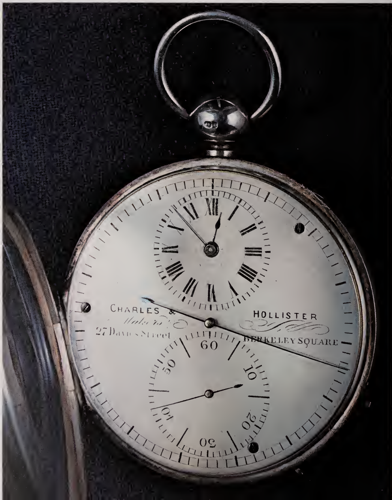
Right: Wider distribution of watches encouraged experiment. This English watch of 1850, by Charles and Hollister, has two trains, one with a stop lever operating the independent seconds hand, and the other with a stop lever for the going train.
