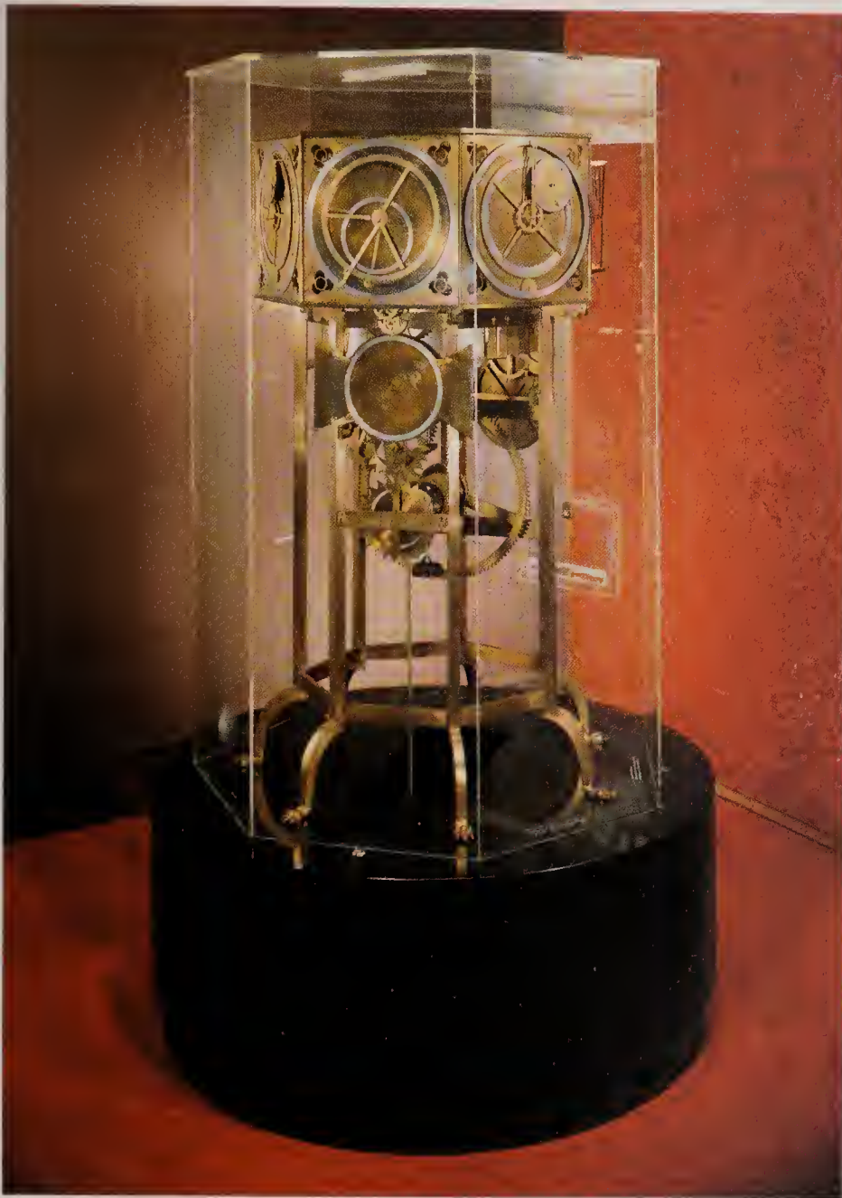
Above: The first reconstruction of Dondi's clock, made by Peter Hayward in 1961 for the Smithsonian Institution, Washington from the original instructions. It is seven-sided and stands about one metre high. The winged central dial is for mean time and the rising and setting of the sun. Above this is the Primum Mobile (sidereal time), with dials for Mars on the left and Venus on the right.
