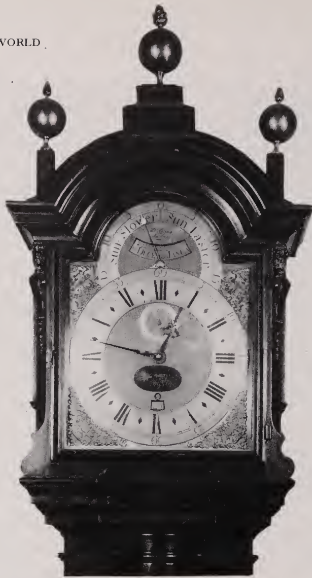
Right : The equation dial shows a plus or minus figure of minutes and seconds to be subtracted from or added to sundial time.
