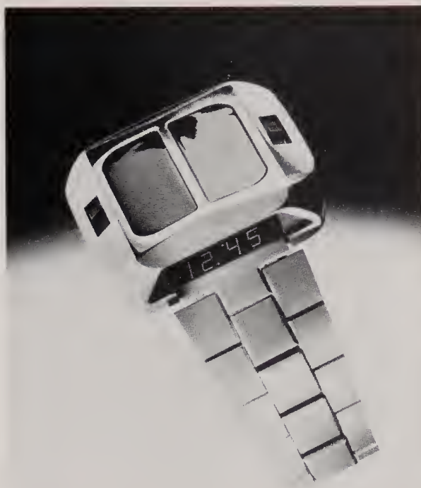
Left: The quartz module has been miniaturized to watch size and can be powered by a solar cell to give indefinite operation. This version is the Synchronar.
