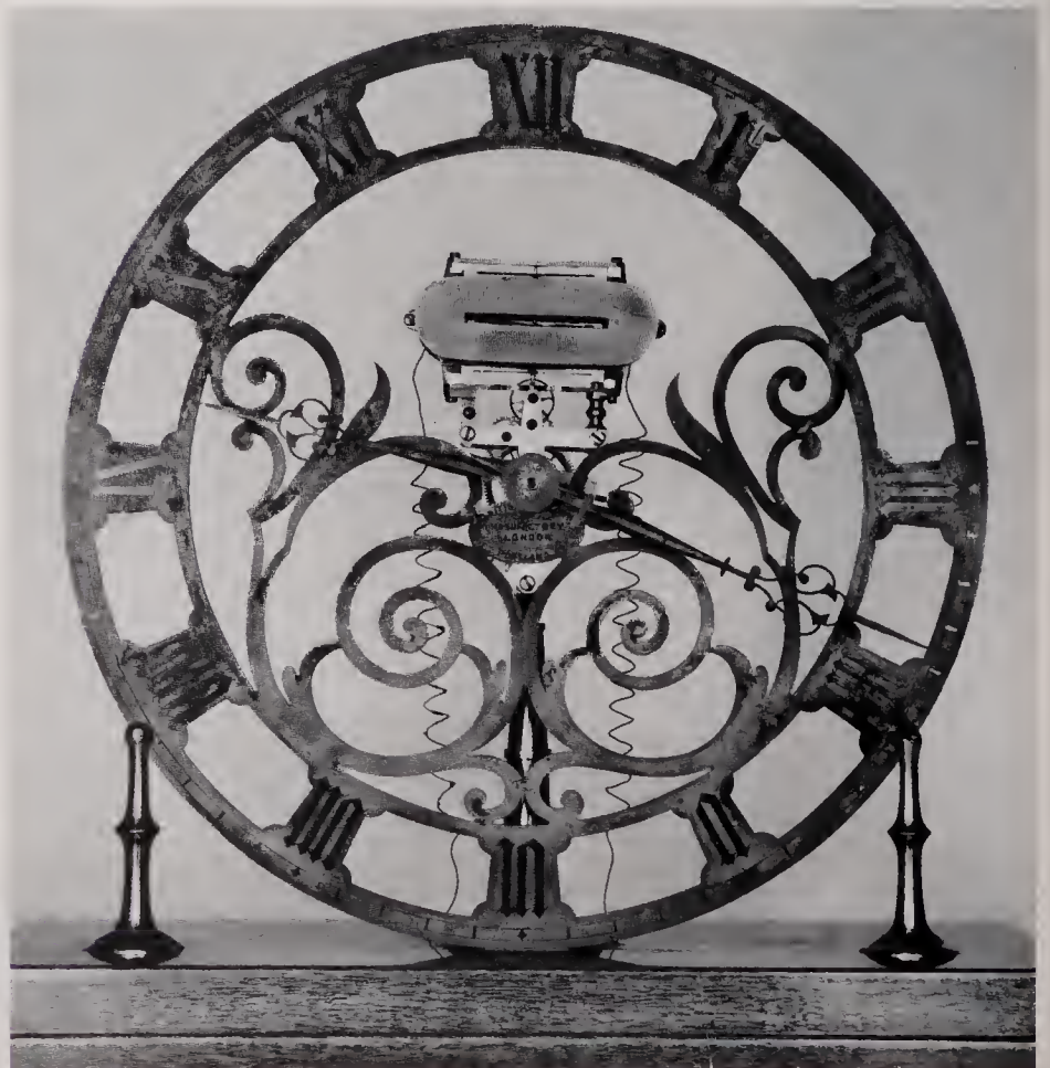
Below, left and right: The electric master clock and slave dial made by Wheatstone's company, the British Telegraph Manufacturing Co., in about 1870. A pendulum with a coil for a bob behaves like a generator of alternating current to drive the slave.
