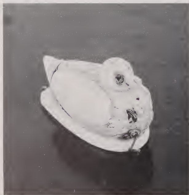
Below: A miniature portable compass dial in the shape of a duck. The compass helps to align it north-south to read the shadow.
