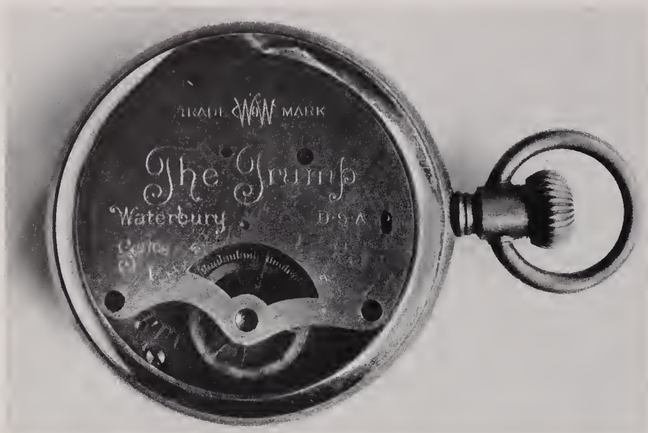
Above: One of the Waterbury short-wind models. The twin teeth of the duplex escape wheel can be seen above the plain balance. On the right is the same watch, in a style that became classic for pocket watches of all qualities.
