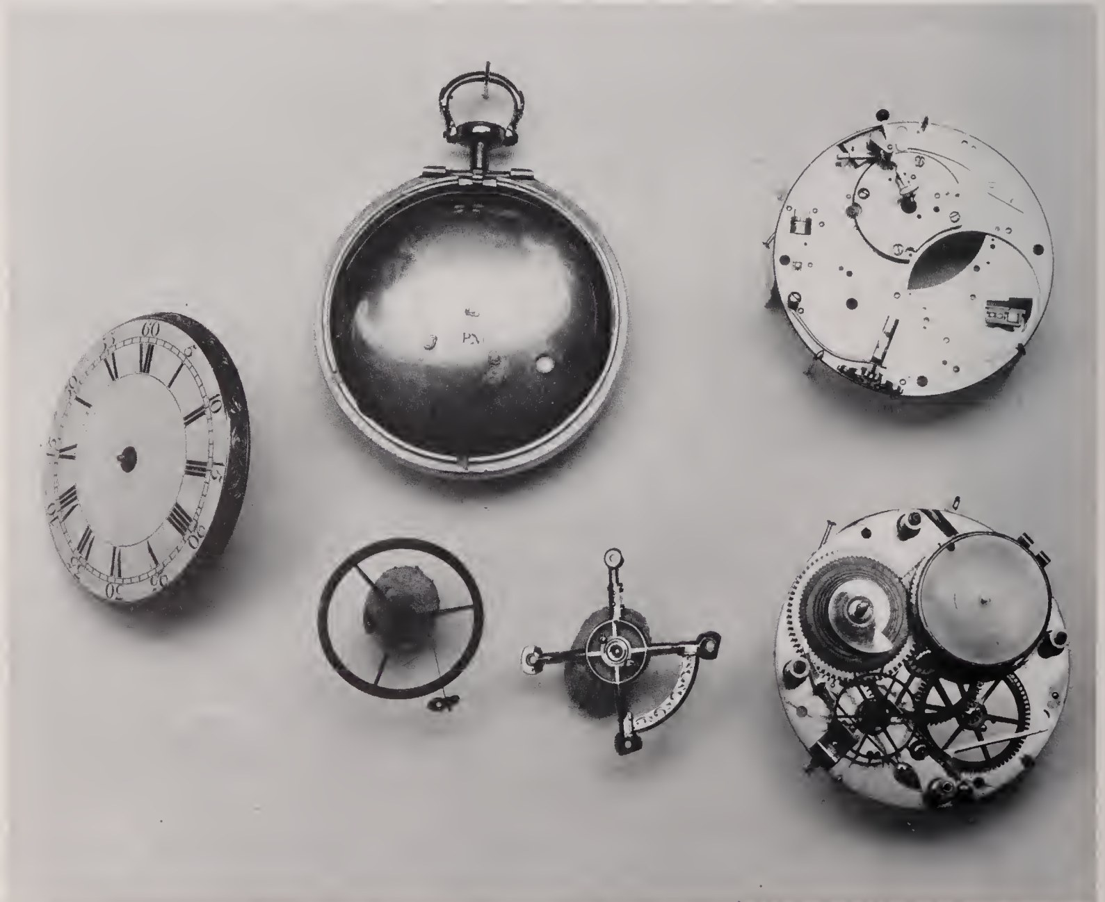
Below : Parts of the Mudge lever watch. The balance and the cross-shaped balance cock (mounted on corks for photography) are at bottom centre. The movement was jewelled with rubies for the balance, sapphires for the train wheels, and milky sapphire for the pallets and notch stones.
