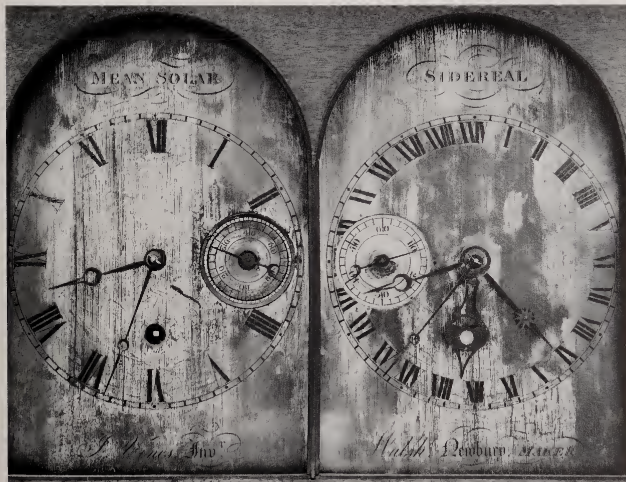
Left : Sidereal and mean time dials designed by Joseph Vines in 1836 and made by Walsh of Newbury. There is only one escapement beating sidereal seconds. The small seconds dial on the mean time clock revolves slowly backwards so that the hand can show mean time seconds and sidereal seconds.
