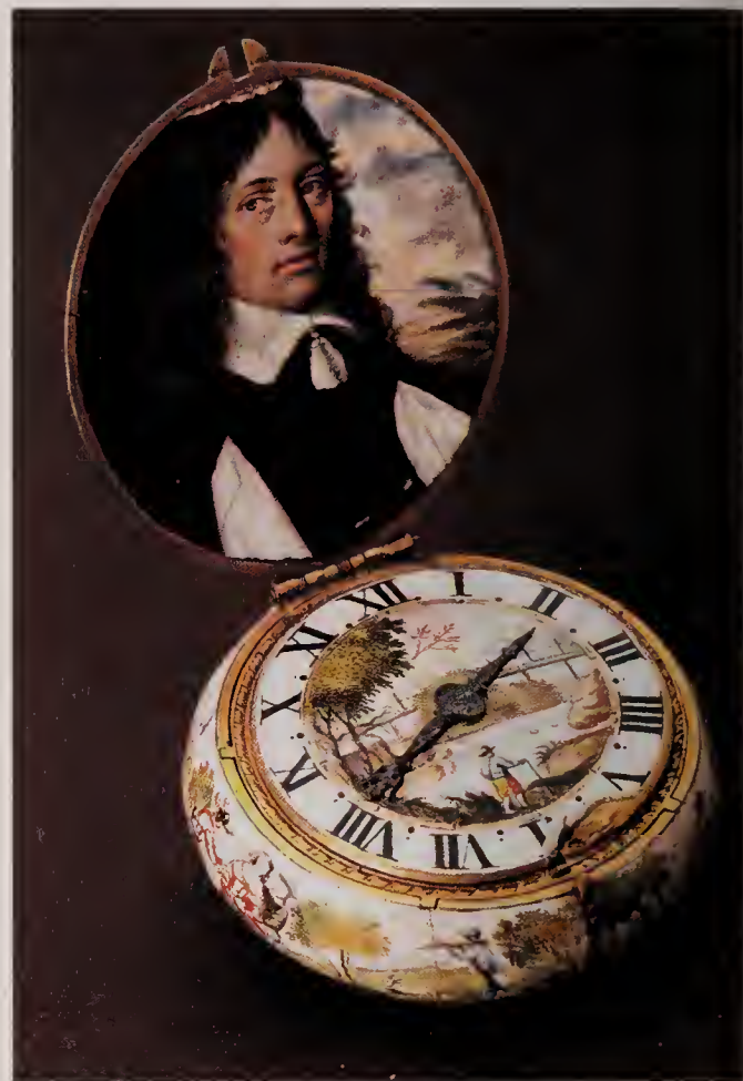
Left: A late Renaissance travelling alarm clock made in Lübeck by Nicolaus Siebenhaer. The small knobs on the outer double-XII chapter ring are touch knobs for finding the time in the dark. Inside is a 1-24 ring of Arabic numerals, then a double-XII ring. There is a moon dial in the zone.
