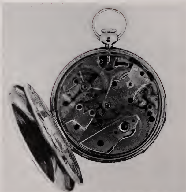
Above: A Breguet montre à tact with a cylinder escapement in a gold case. Turning the hand until it stopped indicated the time in the dark or to a blind person.
