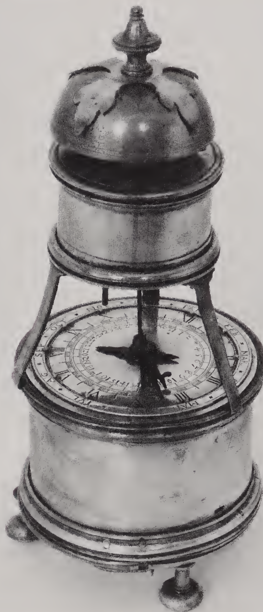
Above: A drum timepiece (i.e. not striking) to which a separate alarm mechanism has been attached. The single hour hand trips the pre-set lever below the alarm. The central hand on the timepiece shows the month. It is spring-driven and dated about 1600. A spiral spring was added to the circular balance some time after 1670.
