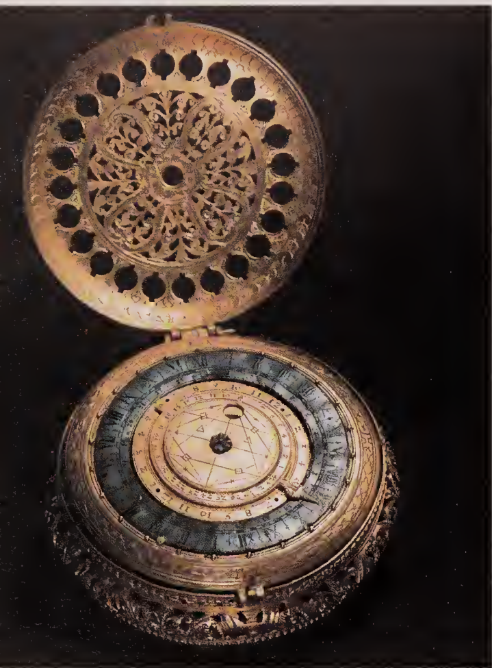
Left: A late Renaissance travelling alarm clock made in Lübeck by Nicolaus Siebenhaer. The small knobs on the outer double-XII chapter ring are touch knobs for finding the time in the dark. Inside is a 1-24 ring of Arabic numerals, then a double-XII ring. There is a moon dial in the zone.
