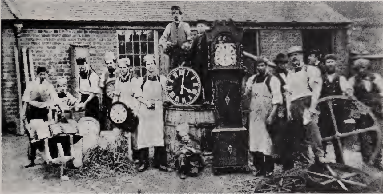
Left : The staff of Ashbourne, Derby, England, packing clocks into a crate in about 1865. The firm made longcase and skeleton clocks on a batch programme which, as in other small factories of the time, had some unrecognized elements of mass production.
