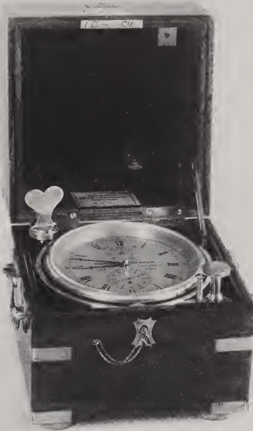
Left: A two-day box chronometer by Charles Frodsham, London. Two-day chronometers were normally for use at sea. The key, in a hole near the top hinge, was removed and the chronometer turned over in its gimbals for winding through a covered hole in the back. An up-and-down dial showed the number of hours in reserve.
