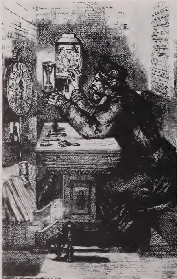
Above : A clockmaker's workshop c. 1740, in a print by Martin Engelbrecht, Augsburg. The frame of a watchman's clock and a foliot are propped up against the anvil base in a way reminiscent of the Stradanus print on page 62. Again, the bench work, such an essential part, is very much in the background.
