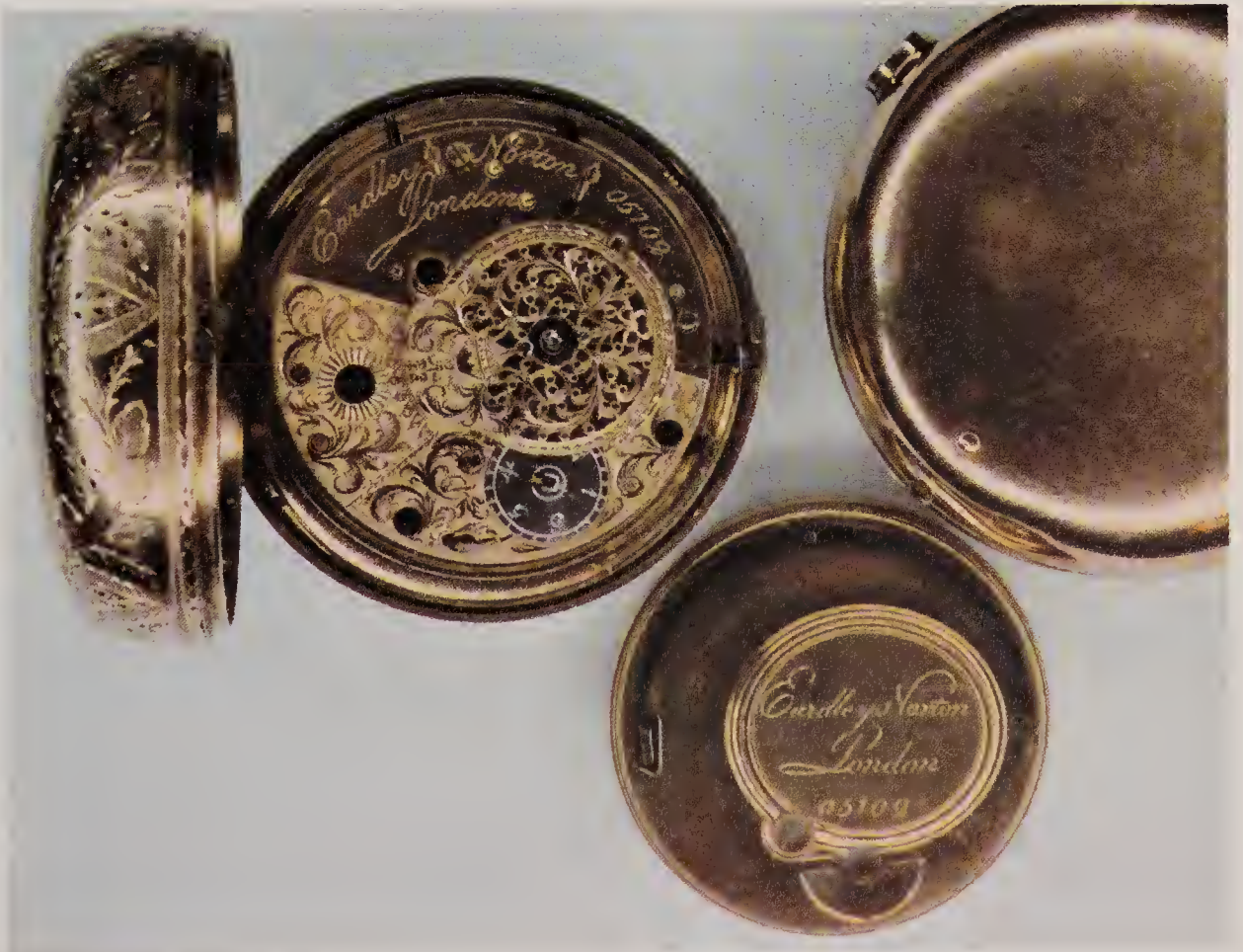
Right : A late eighteenth-century quarter repeater watch with diamond endstone by Eardley Norton, in an 18-carat gold case. The dust cap is shown below and the outer case on the right.
