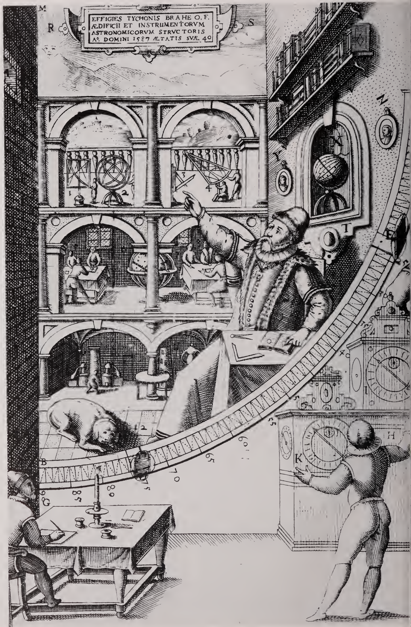
Right : Tycho Brahe's mural quadrant and two clocks, shown in his Astronomiae Instauratae Mechanica of 1602.
