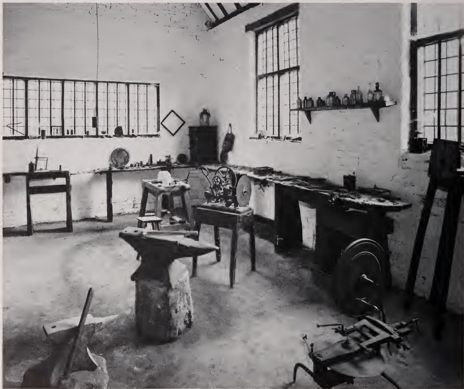
Above : A reconstruction of Samuel Deakin's workshop of 1771 at the Newarkes Houses Museum, Leicester. The forge and anvil are in evidence, as in many earlier prints. The wheel tooth cutting engine in the foreground is a forerunner of production tools.
