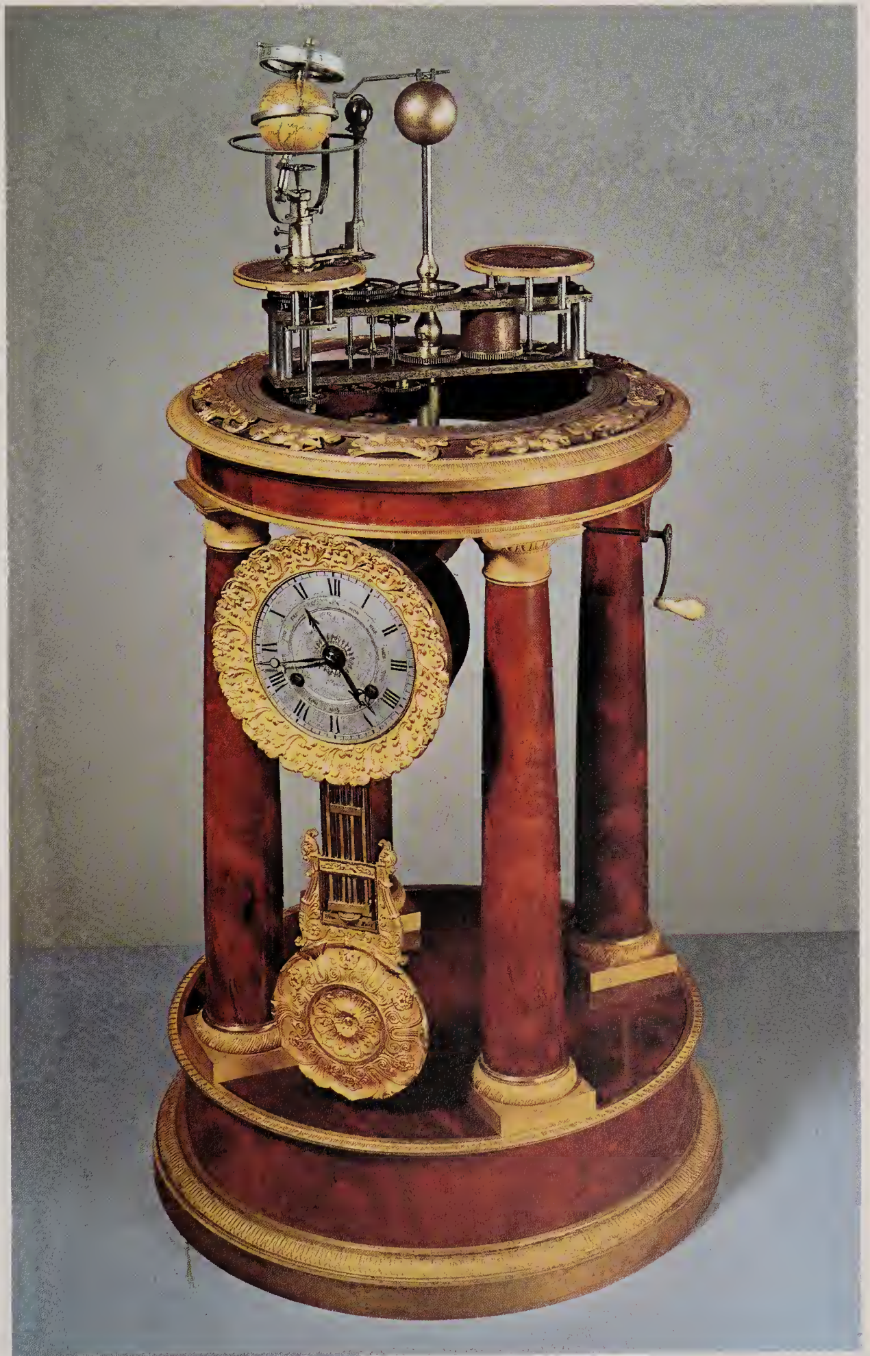
Right : An orrery clock by the French maker, Raingo, who made a number of them. The orrery on top is wound separately and can be set off by the clock or operated by hand for demonstration.
