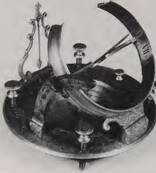
Left : A universal ring sundial made in the eighteenth century in Germany. It has a pin gnomon, the shadow of which indicates the time. The hour circle with gnomon can be angled to the local latitude, but is not suitable for use at sea, as it has to be levelled and orientated, for which a plummet and compass are provided.
