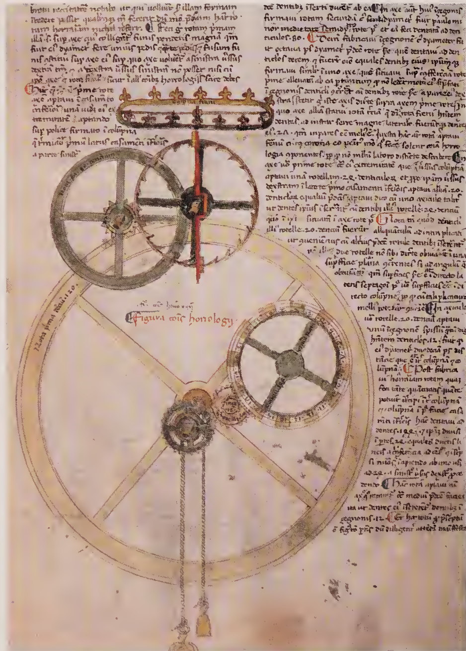
Below: A fourteenth-century copy of 'Il Tractus Astarii', in which Giovanni da Dondi described in detail the construction of his planetary clock of 1348–64. The central drawing is by far the earliest of a clock escapement, showing the crown wheel and the balance, which is also like a crown.
