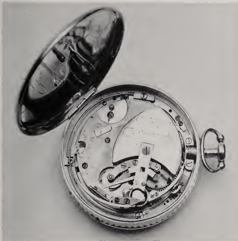
Above : The oscillating weight which bounces to wind a Breguet montre perpetuelle. The pendant is at the top when the watch is in a pocket so that the pedometer weight can bounce as the wearer moves.
