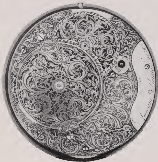
Left: The back plate of Larcum Kendall's first duplicate, K.1, of H.4. Captain Cook used it for navigation in his second voyage to the Pacific in 1772.
