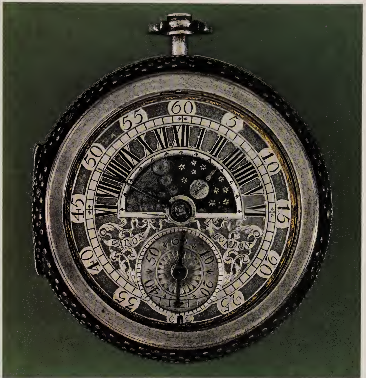
Right : A sun and moon dial is a feature of this late seventeenth-century watch by Peter Garon, London. The moon shows the hour in the semi-circular aperture at night and the sun by day. The large hand indicates minutes and the small one at the bottom, seconds. The time shown is just after 02.49 a.m.
