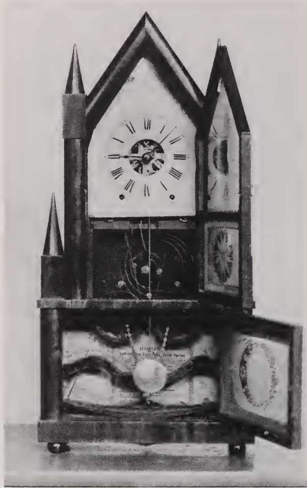
Left: A wagon spring clock, invented by Joseph Ives, and made by Birge and Fuller. A leaf spring, like that used in a cart, drives the clock through a lever and chain driving a fusee on each side.
