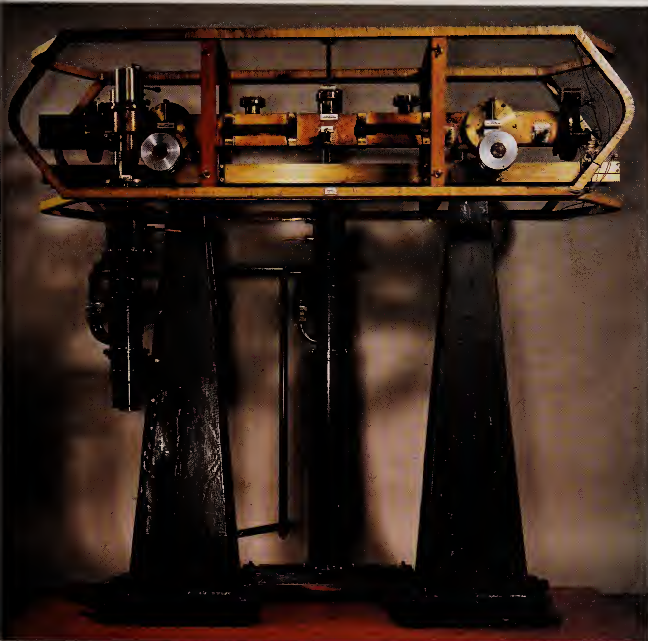
Left : The original atomic clock at the National Physical Laboratory. It kept time to the equivalent of one second in three hundred years. The latest version is more than ten times more accurate.
