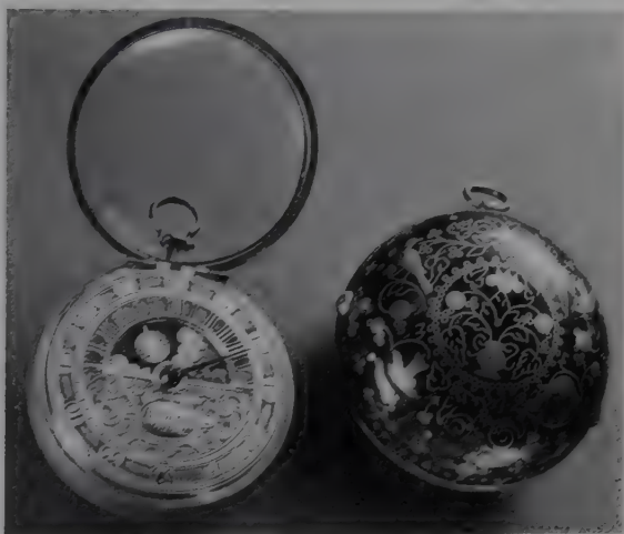
A pair-cased watch by Bushman of London c.1720 the outer case of tortoise shell inlaid with silver.
