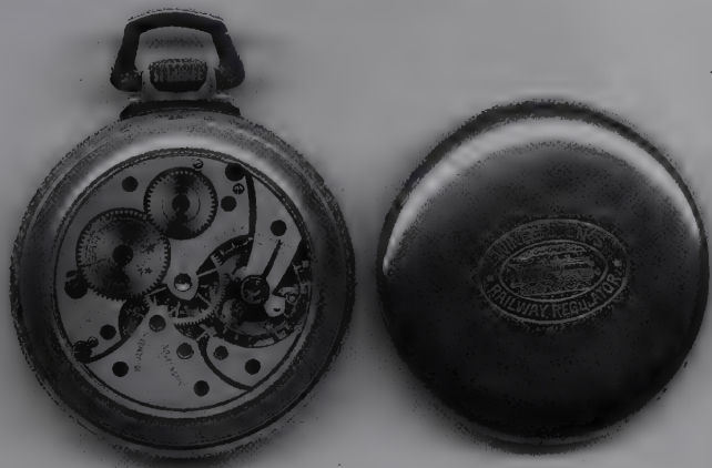
A classic Swiss 15 jewelled movement which was made in many sizes for pocket or wrist watches.
