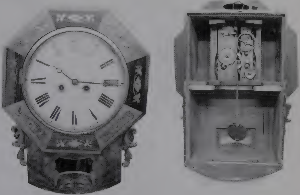
A Black Forest drop dial clock, the octagonal dial surround veneered in mahogany and rosewood with brass inlay and a 9 inch wooden dial. The 30 hour striking movement is a spring driven version of their traditional wooden framed weight driven clock. c.1870.
