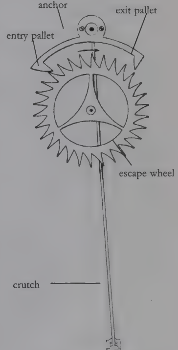
The anchor or recoil escapement
