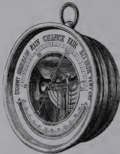
An aneroid barometer, note the corrugated drum used as the pressure sensing element
