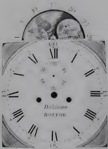
12 inch dial with fan corners and rolling moon for Thomas Dickinson of Boston c.1815.
