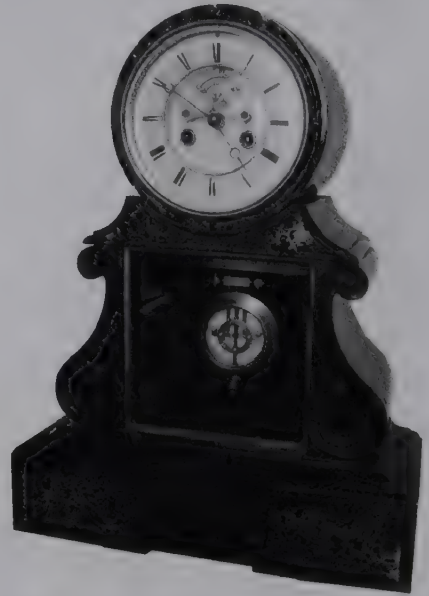
French black marble clock with visible escapement and compensated pendulum c.1880. (Courtesy Barrie Fitton)
