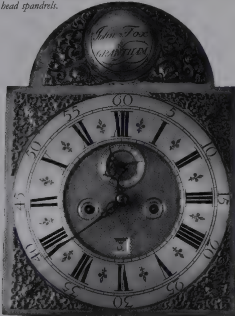
A 12 inch break-arch dial of c.1725. Note the minute numbering has become more prominent and the maker's name engraved on a domed roundel in the arch supported by 'dolphin' spandrels.
