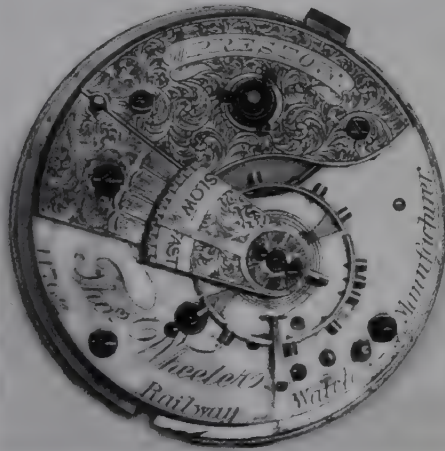
A 'Railway watch' movement with cut bi-metallic balance by Thos. Wheeler of Preston c.1870.
