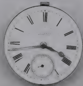
The lever watch was accurate enough to warrant a seconds dial.
