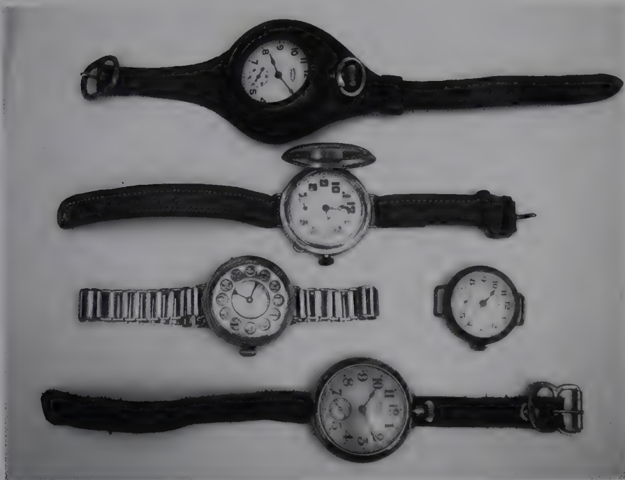
Some early wrist watches, the upper one is a small pocket type watch in a leather pouch, the one below is a silver cased full hunter style case to protect the glass h.m. 1907, the one below has a protective cover and the other two are purpose-made wrist watches by the Ingersoll company.
