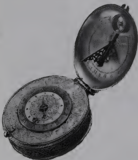
This watch incorporates a sundial and compass to enable it to be set to time. German made c. 1590
