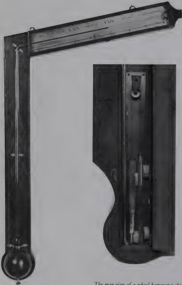
The rear view of a wheel barometer showing the arrangement of the pulley and counter-balanced glass weight resting on the mercury in the U tube
