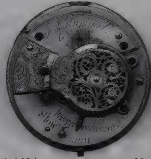
A typical 19th century verge movement. Note that the plate with the makers name secured by two screws and enables the spring barrel to be removed to replace the main-spring without having to dismantle the complete watch.
