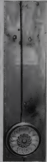
The pendulum of this clock is a little unusual in that it is cast with a sun flower decoration.
