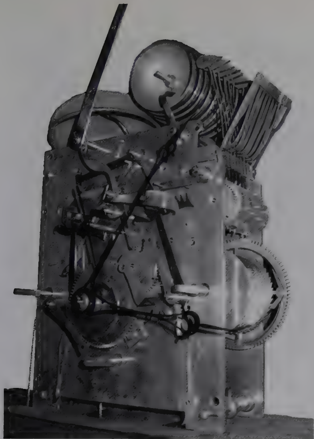
Three train movement by Hanley and Moore of the William Hall clock. (Front plate 7X8ins).
