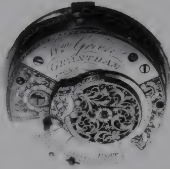
Watch movement no.57283 with verge escapement by William Green.
