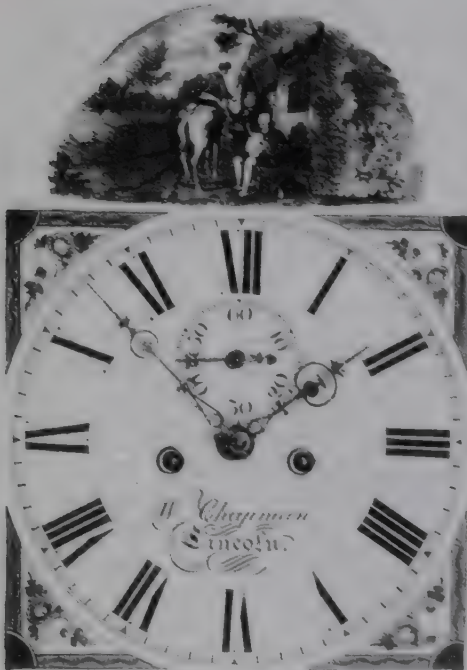
12 inch arch dial for Wm. Chapman of Lincoln with transfer printed design c.1840. Photo courtesy Brian Loomes
