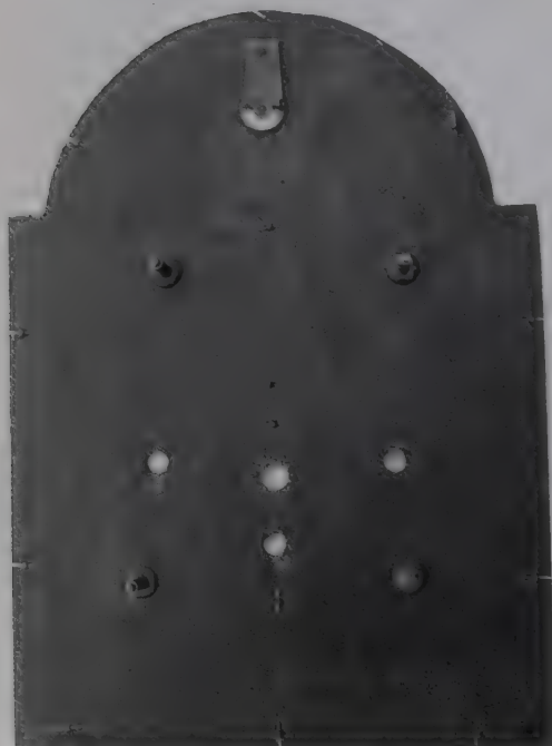
The rear of the Hall dial showing how the two dial plates are fastened together by many small pinned pillars.
