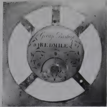
The dial plate of one of George Bishop's 30 hr. clocks. Note the cut away segments behind the chapter ring a feature used by many northern clockmakers to reduce the weight of brass.
