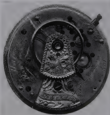
A lever movement with full Liverpool jewelling. Note that the balance cock is now much smaller and has a diamond end stone.
