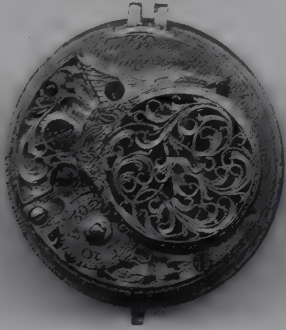
A typical mid 18th century watch movement. The pierced broad foot of the balance cock is typical of the period.
