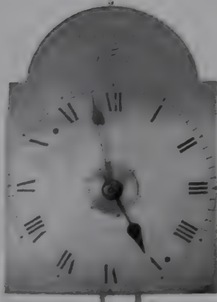
A miniature lantern clock with verge escapement and 6 in. silvered brass dial by Geo. Gudgeon of Bury c.1810
