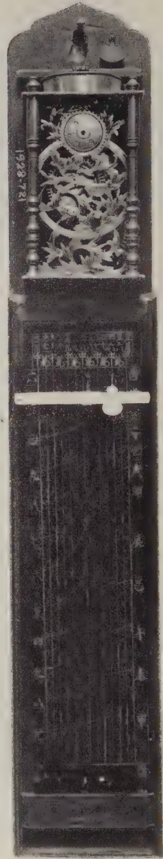
Japanese Pillar Clock, Weight-driven, with Balance and Spring.
