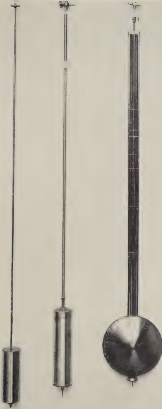
Three Clock Pendulums : (Left) Uncompensated. (Centre) With Graham's Mercurial Compensation. (Right) With Harrison's Gridiron Compensation.
