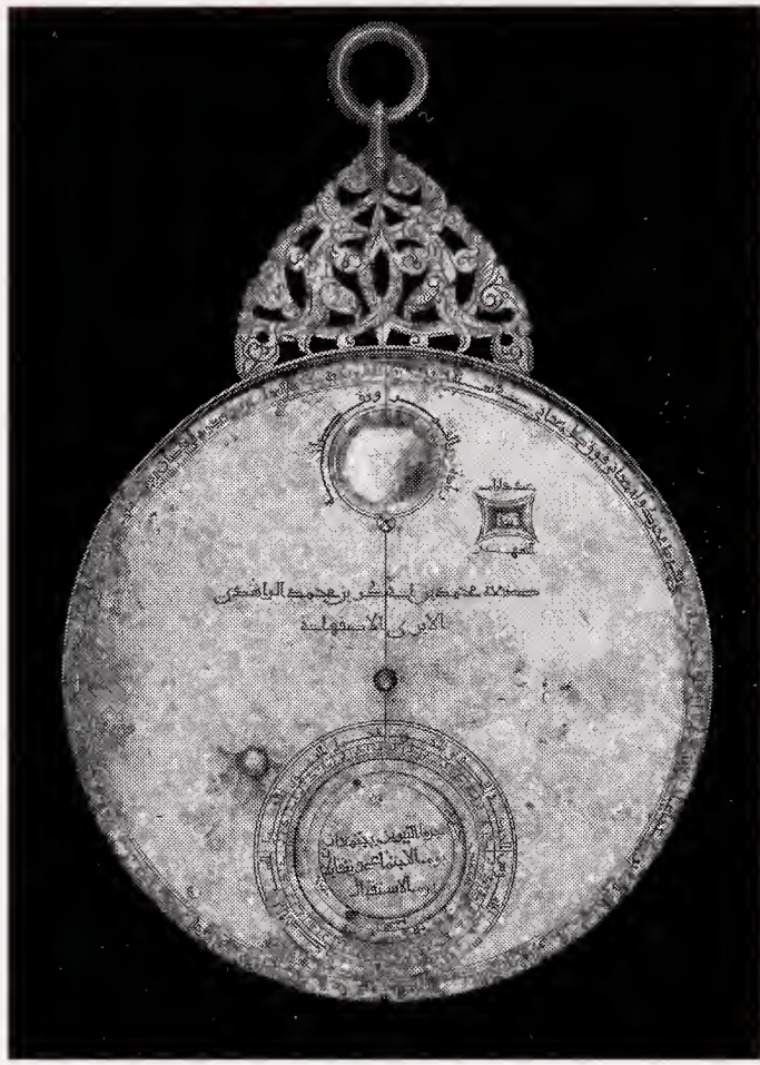
(Above) The Islamic geared astrolabe held in the Museum of the History of Science in Oxford (MHS inv. 48213). It was made in Isfahan, Iran, in 1221/2 AD. This is the back face, with a moon-phase dial (top), date indicator (top right) and concentric dials showing the Sun and Moon in the zodiac (bottom).
