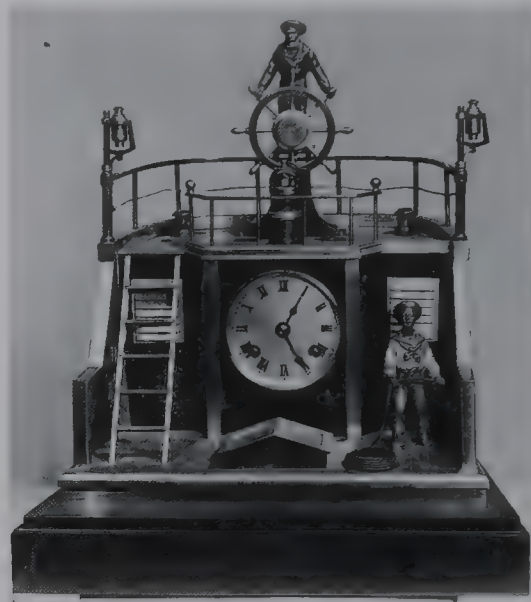
A helmsman clock on which he is rocked by the pendulum to mimic sea motion.
