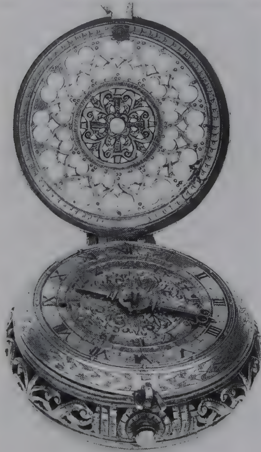
A 16th c clock-watch , i.e. a watch that strikes the hours. It has a stackfeed and verge escapement and is in Basingstoke Museum.
