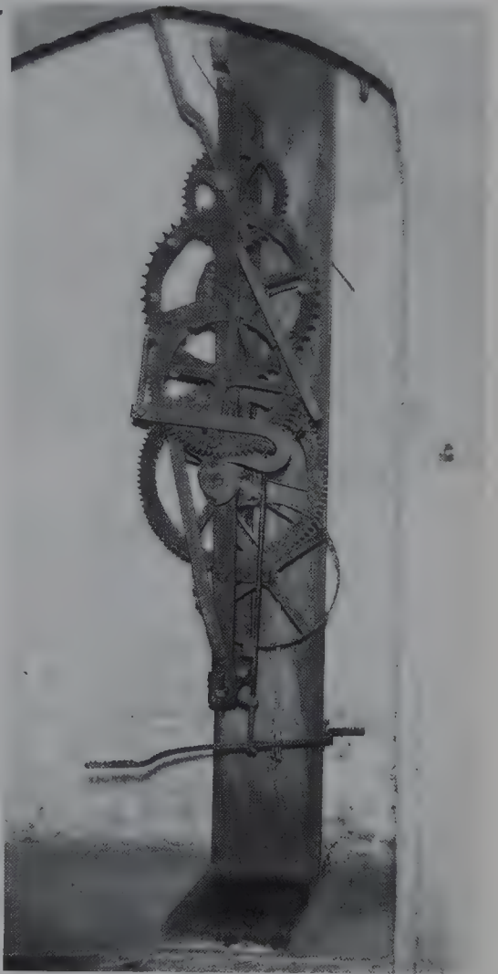
The vertical frame of wood and the underslung foliot of an indigenous English clock in Cothele House, Calstock, Cornwall.
