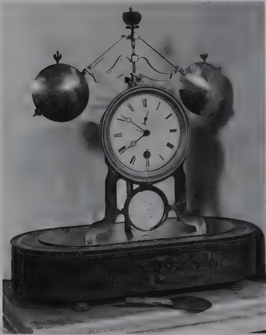
An equipoise pendulum clock that goes for a year at a winding. It has a modified chronometer escapement but is not a good timekeeper.
