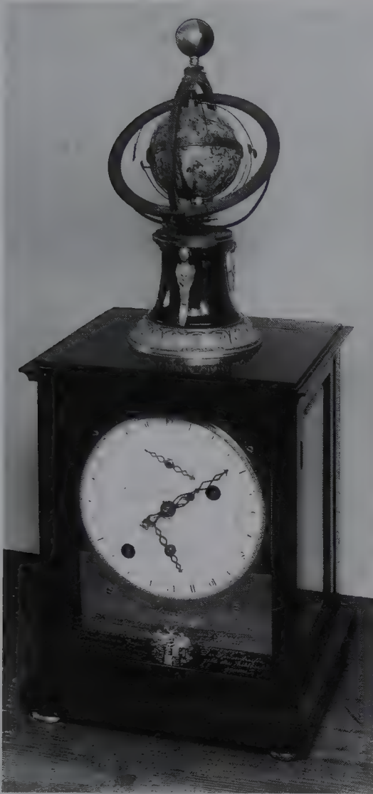
Father Philip Hahn of Echterdingen made this astronomical clock in 1781. On top is a celestial sphere showing motions of the sun, moon and Venus. ( H. Bertele Coll )
