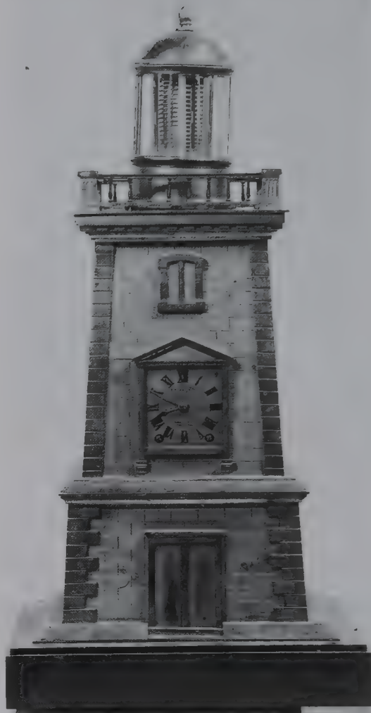
One of many styles of lighthouse clock . It has a torsion pendulum. Note the cylindrical spring in the 'lamphouse'. (Sotheby's)
