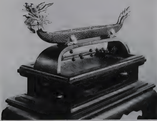
A dragon boat of lacquered wood, a form of Chinese fire clock or more accurately alarm. (Wuppentaler Uhren Museum, Germany)
