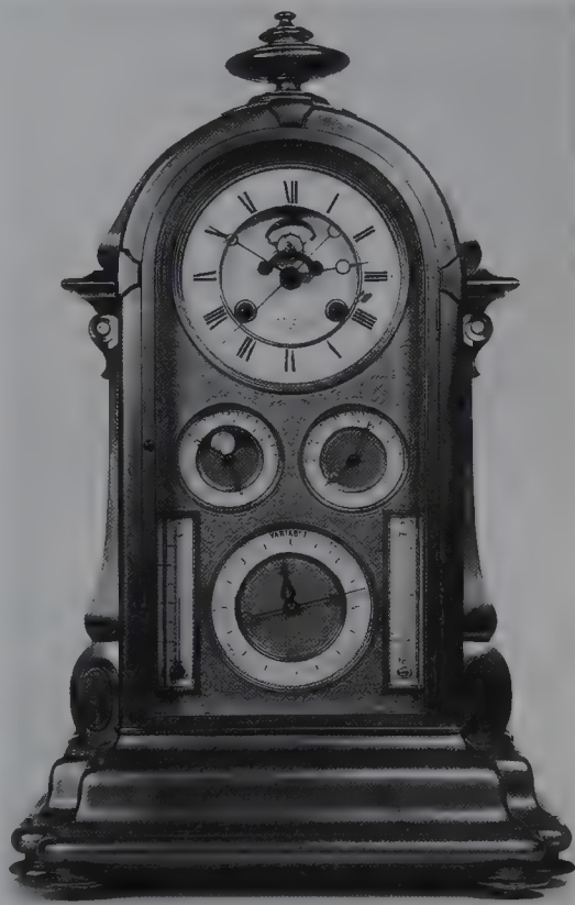
This 19th c mantel clock by Le Roy et Fils, Paris, has a visible escapement, a calendar and moon dial, with thermometers reading Fahrenheit, Centigrade and Reamur. ( Christie's )
