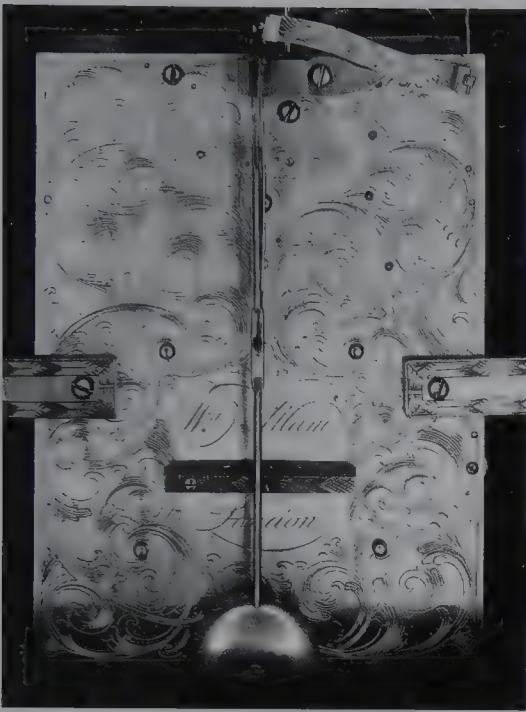
At the top of this movement of c1760 by William Allam, London, the rise-and-fall regulator , which alters the effective length of the pendulum, can be seen. (Sotheby's)
