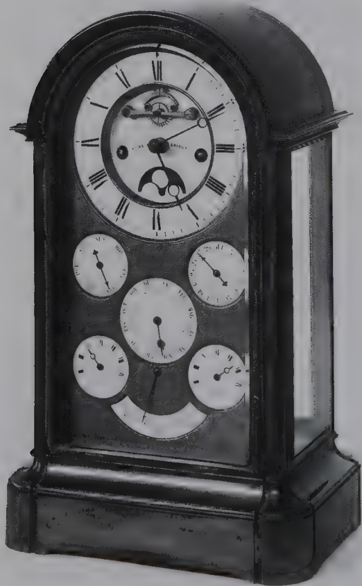
Sunrise and sunset dial (the bottom round ones) on a clock by Boxall, Brighton. The dials above them give day and date. Note the Brocot escapement.
