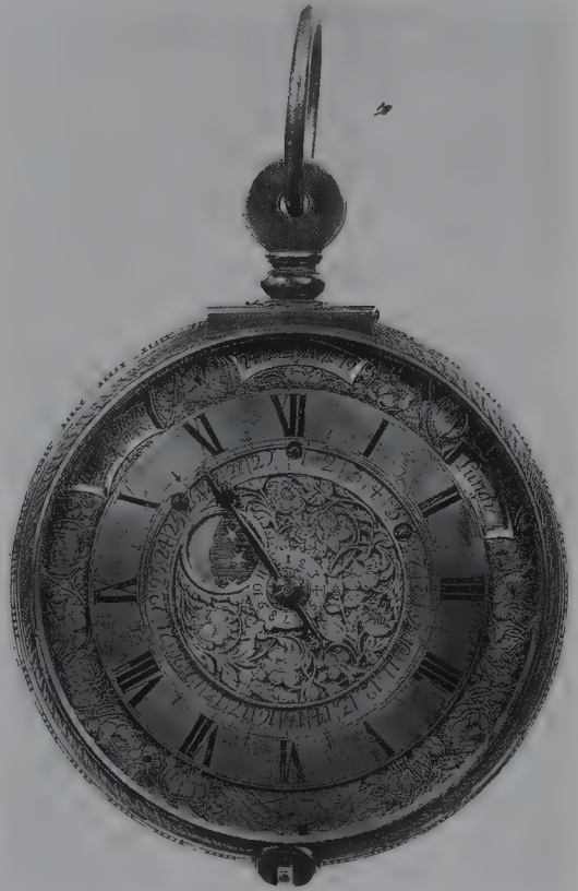
A very early one-hand watch with a pendant that is just a ring. It has moon and day and date indication, and an alarm. ( Christie's )
