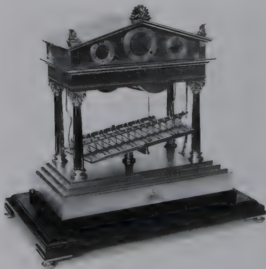
A Congreve clock of the mid-20th c made by E. Dent and Co., Pall Mall, London.
