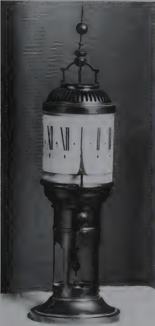
A French night clock of 1860. The hand shows the time on an illuminated pale blue revolving glass bowl.
