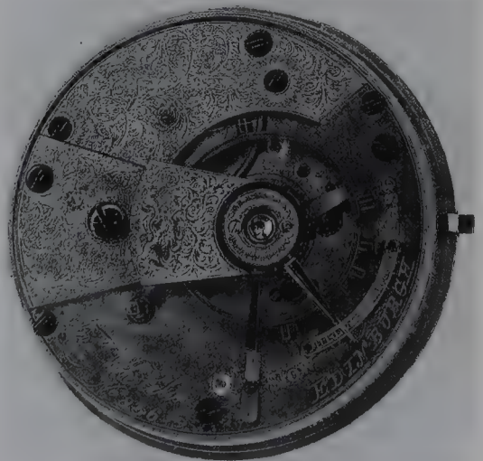
A James Whitelaw, Edinburgh, watch with a diamond end stone to the balance staff.
