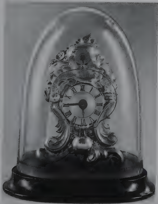
A tiny zappler clock. Note the circular pendulum 'rod' at the front of the clock.
