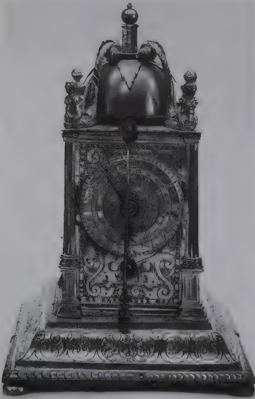
A spring-driven alarm tabernacle clock of 1611 with concentric hour chapters I to XII and 13 to 24, with quarter-hour divisions. ( Sotheby's )
