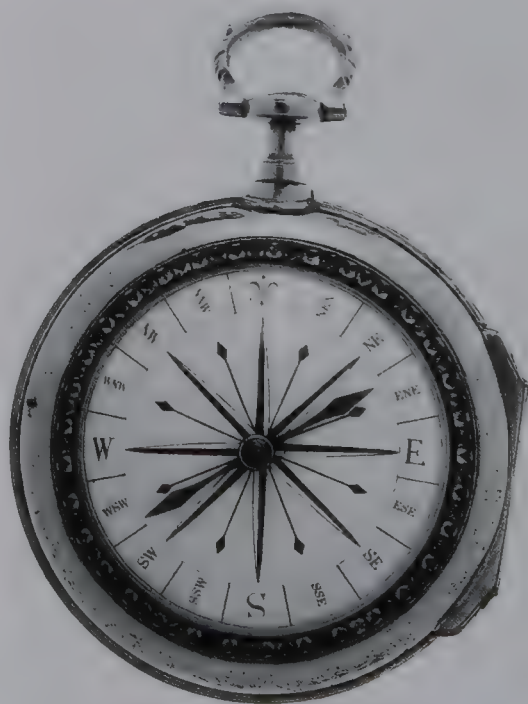
The back of a compass watch . It is not stated how the magnetism affects the timekeeping.
