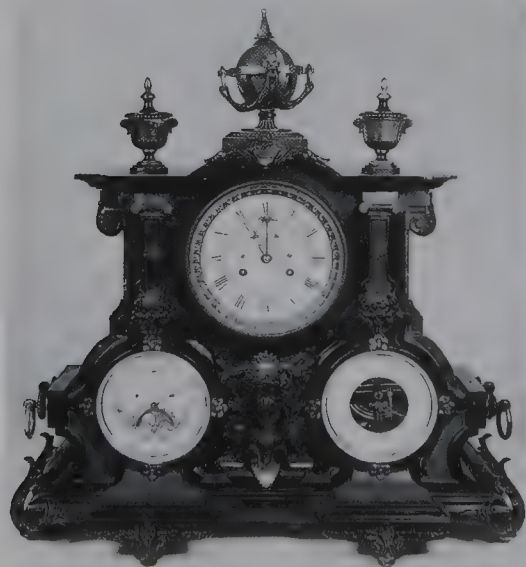
An elaborate French late 19th c marble clock and barometer with a calendar and moon dial. A Brocot escapement can be seen at the top of the dial. The black marble has red marble panels.
