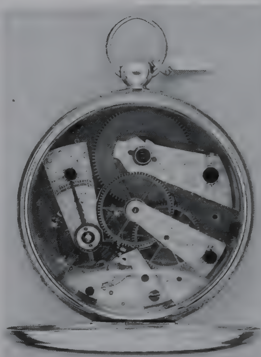
The Lépine calibre movement of an English lever watch hallmarked 1822 and unsigned although the maker may have been J.F. Cole. ( Sotheby's )
