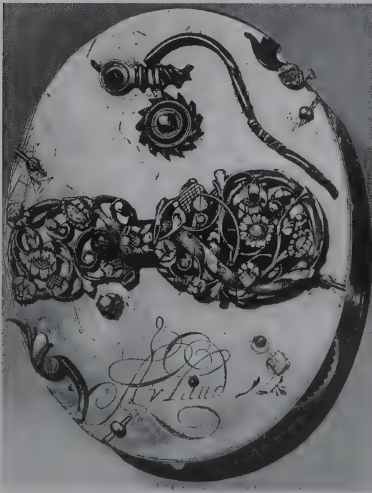
An early form of setting up a mainspring by ratchet wheel and click (at top) of a watch of c1615 by Antoine Arlaud.
