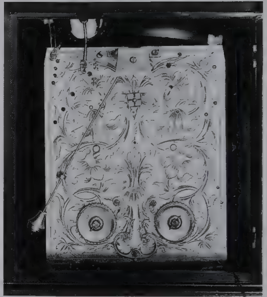
The back plate of a Daniel Quare bracket clock with elaborate acanthus engraving. Note the bob pendulum held by a latch, used when moving the clock. (Sotheby's)
