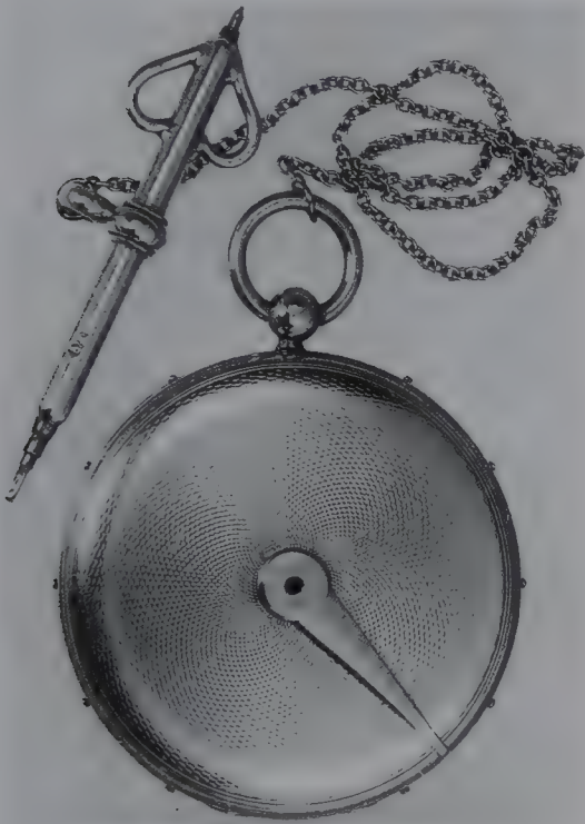
A tact watch for a blind owner devised by Breguet.
