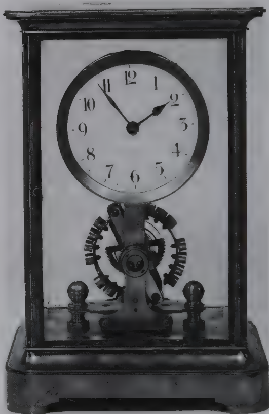
An electric clock of the early 20th c with a large compensation balance. (Phillips)
