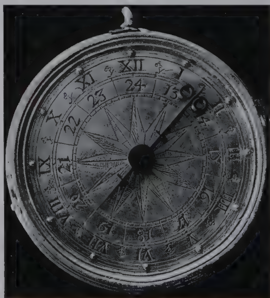
An early double twelve-hour dial in Roman and Arabic numerals with a single hand.
