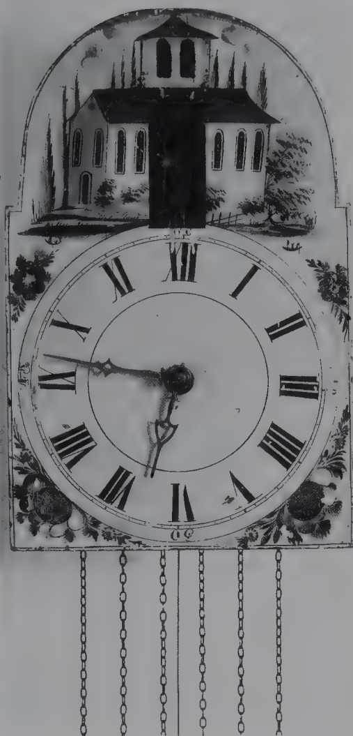
A typical Black Forest wall clock with a painted dial and pull wind (pull-up weights).
