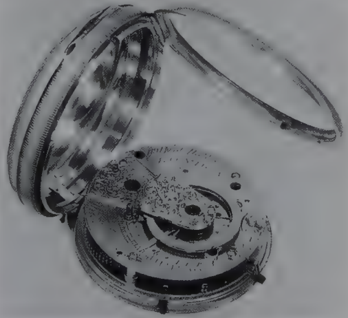
A large balance cock on a full-plate watch movement signed Thos. Earnshaw.
