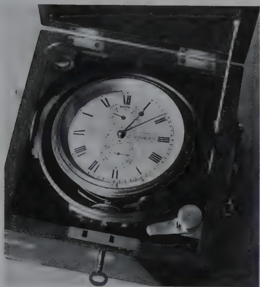
A marine chronometer by Parkinson and Frodsham, London. Note the up-and-down dial. The key is housed at top left and the lever at bottom right locks the gymbals for transport.
