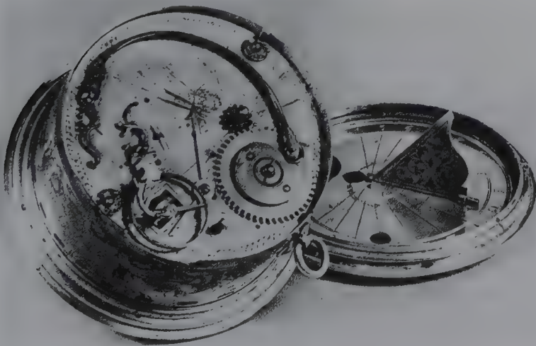
A stackreed with a long curved spring on a late 16th c table clock. Note the one-arm balance wheel and bristle regulator on the arm with arrowed end.
