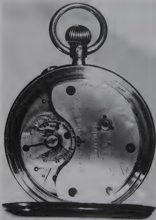
A karrusel of 1900-1 by Golay of Myddleton Street, Clerkenwell, London, which did very well in the Kew trials.
