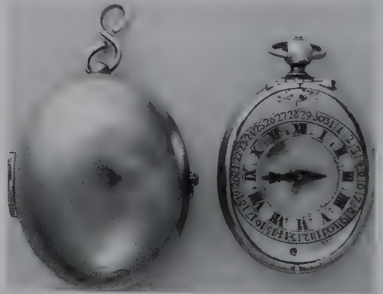
A puritan watch of c1630 with a three-wheel train, gut fusee, and worm and wheel set-up. ( Sotheby's )
