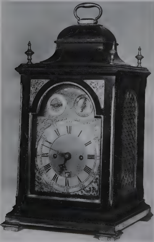
The bell top of a Josiah Emery bracket clock of c1780 with a subsidiary dial for adjusting the rate by the pendulum length at top left and strike/silent dial at top right.
