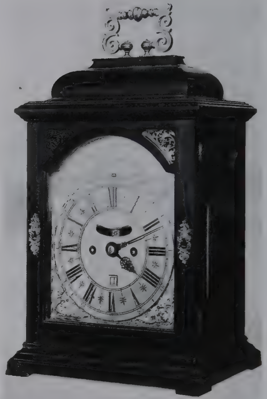
A mock pendulum in the dial of an early 18th c bracket clock by Windmills, London.
