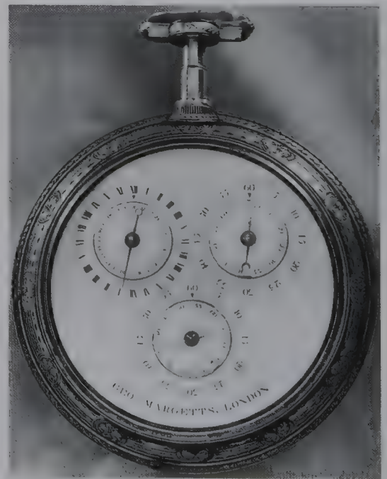
Sidereal time as well as the time of day is shown by this large watch by George Margetts, London, of c1790.
