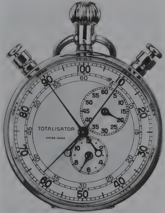
An industrial timer of 1964, the first to give the total time of operations as well as individual times.
