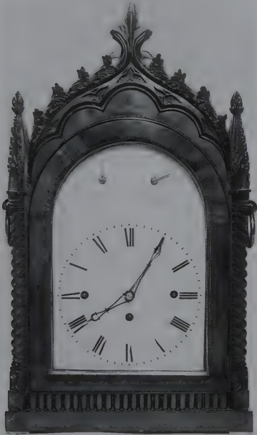
A Gothic clock of c1840 in mahogany with quarter-hour striking on eleven bells. A strike/silent dial is at top left and a tune selection is at top right. ( Sotheby's )
