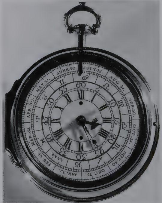
An equation dial on a watch of c1750 by John Ellicott.
