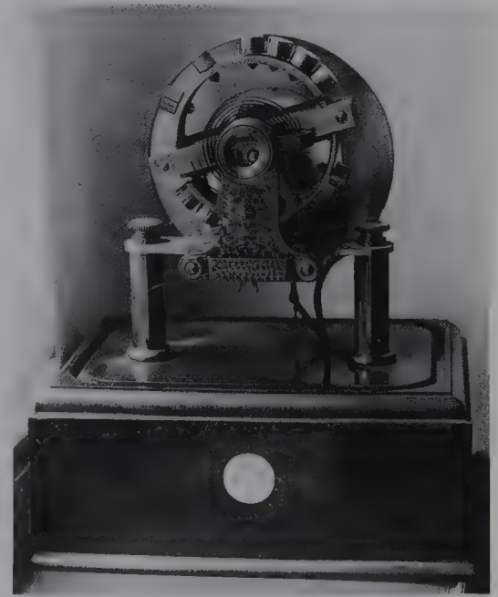
The Eureka clock with a huge balance wheel, that runs for 1,000 days, being powered by a battery in the box under it.
