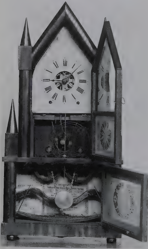
An American waggon-spring clock . The spring is across the bottom of the case.
