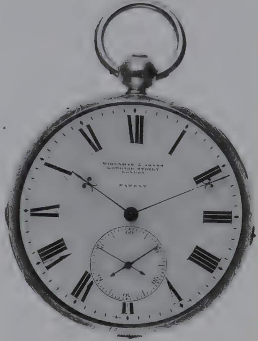
Gothic hands on a large silver gilt split-seconds duplex watch of 1840 by Widenham and Adams, London. ( Christie's )
