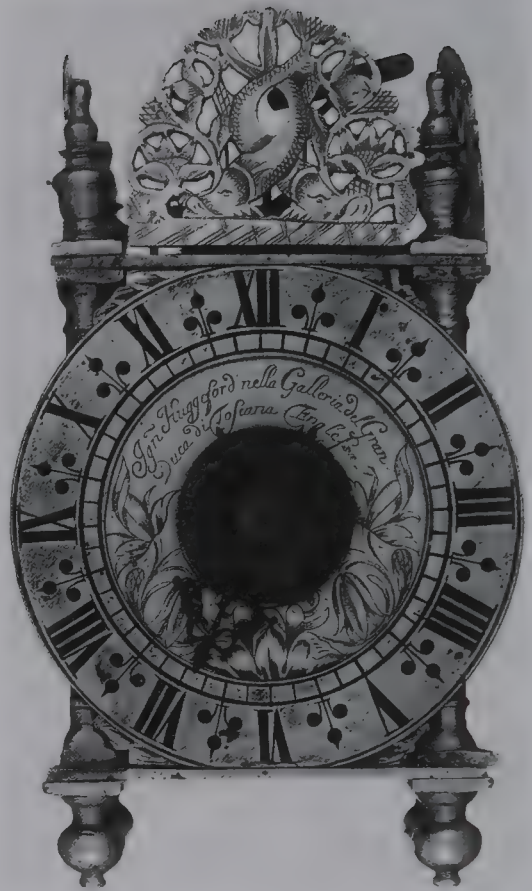
A typical dolphin fret on top of a small lantern clock of c1700 by Ignatius Huggelford. The bell on top has been removed. The dark centre disc sets the alarm. (Sotheby's)
