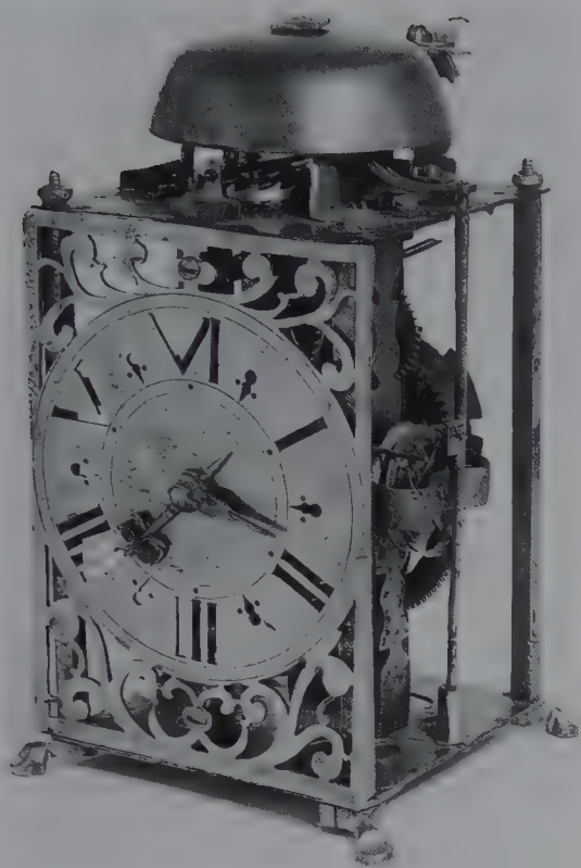
An iron monastic clock with a six-hour dial of the 16th c. The smaller hand is used to set the alarm. ( Bonhams )
