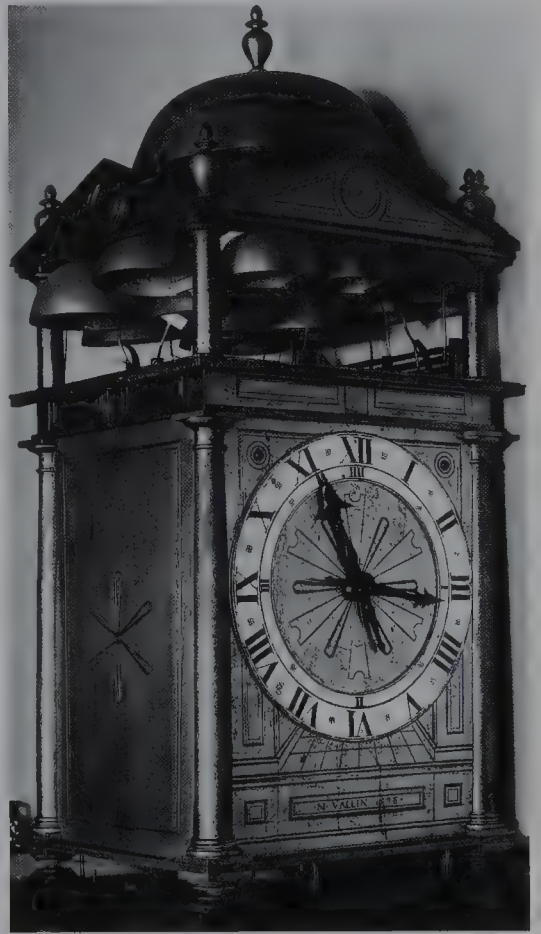
A carillon clock by Nicholas Vallin of 1598, which plays different chimes on thirteen bells. It is in the Ilbert Collection in the British Museum.
