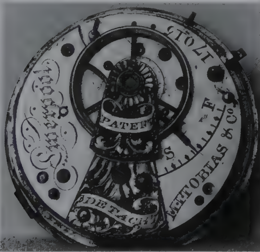
The movement of a typical Liverpool lever escapement watch. It is by M.E. Tobias and Co. ( Dr Vaudrey Mercer Coll. )
