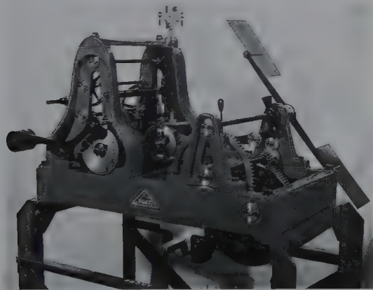
The flat-bed movement of a turret clock by Dent. Note the fly and the leading-off work to the hands at top centre.
