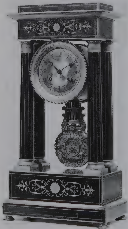
A 19th c French pillar clock with a gridiron pendulum and outside count wheel. (Sotheby's)
