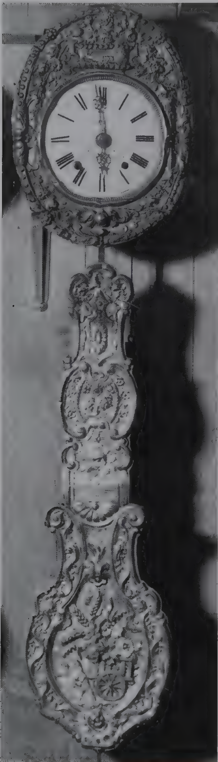
A typical hanging French provincial clock with its ornate exposed repoussé sheet-metal-covered seconds pendulum. ( Hagans Clock Manor Museum, U.S.A. )
