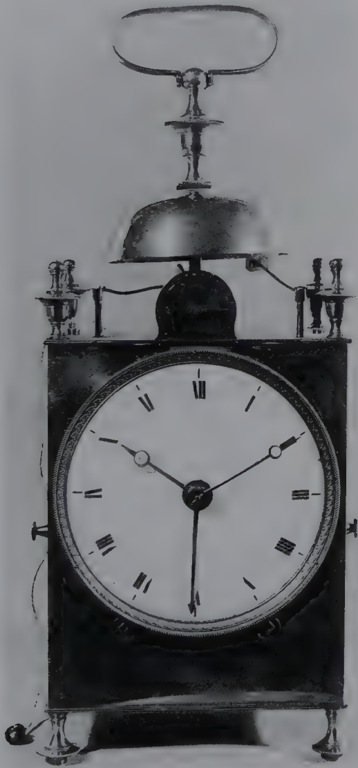
A brass capucine clock of c1820 with an alarm and an hour and half-hour repeater. ( Galerie Genevoise )
