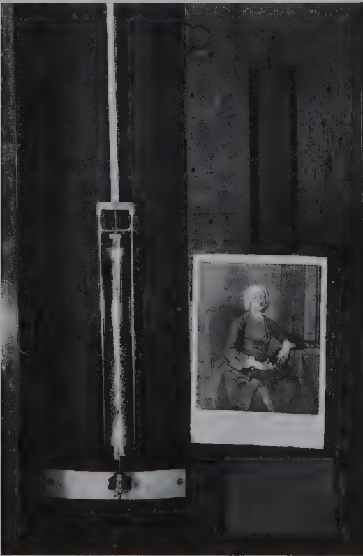
The mercurial pendulum in George Graham's finest regulator, with an engraving of him.
