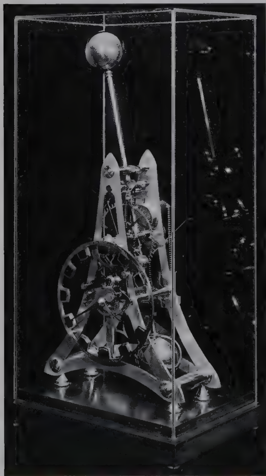
A compound pendulum controlling a 20th c clock by E. Dent and Co., London.
