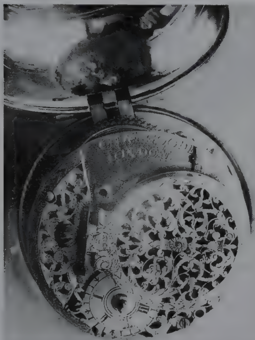
The small dial of this watch by Charles Goode, London, is the regulator of the watch, setting up the mainspring.
