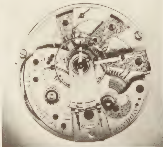
PLATE 127 Gold watch by James Ferguson Cole, hallmarked 1821. Note typical 1820 period English dial a ; superbly finished movement b with Lepine type of calibre, compensated balance and Cole's patented pivoted detent escapement. (British Museum)
