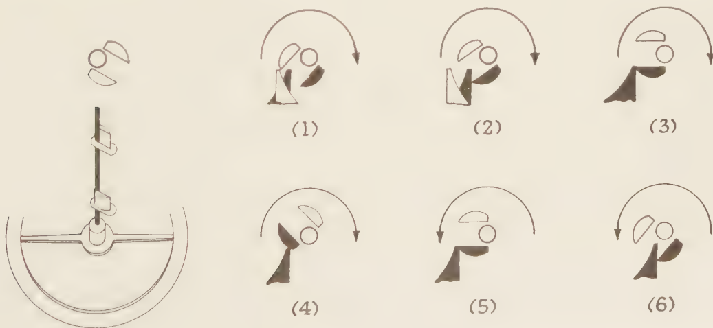
FIGURE 29. The escapement of Harrison's marine timekeeper No. 4. On the left is a perspective view of the verge or balance staff and pallets, looking up from its bottom pivot towards the balance. The six plan views show the sequence of events. White pallet engages with white tooth and black pallet with black tooth. The direction of rotation of the balance staff is shown by arrows. In (1) white tooth has just delivered impulse to white pallet and escaped. In (2) black tooth has engaged with black pallet, but the balance continues in the same direction under its own
