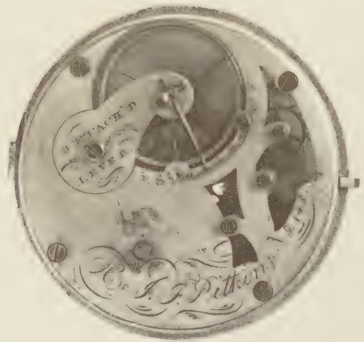
PLATE 150 Movement of lever escapement watch by H. and J. F. Pitkin of Hartford, No. 148. One of the earliest American factory-made watches, circa 1838. (The Smithsonian Institution, Washington, D.C.)
