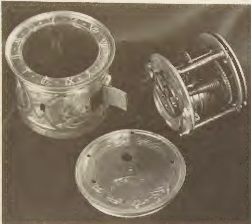
PLATE 7 German watch or small drum clock, circa 1550. a movement, b exterior. (The Time Museum, Rockford, Illinois)
