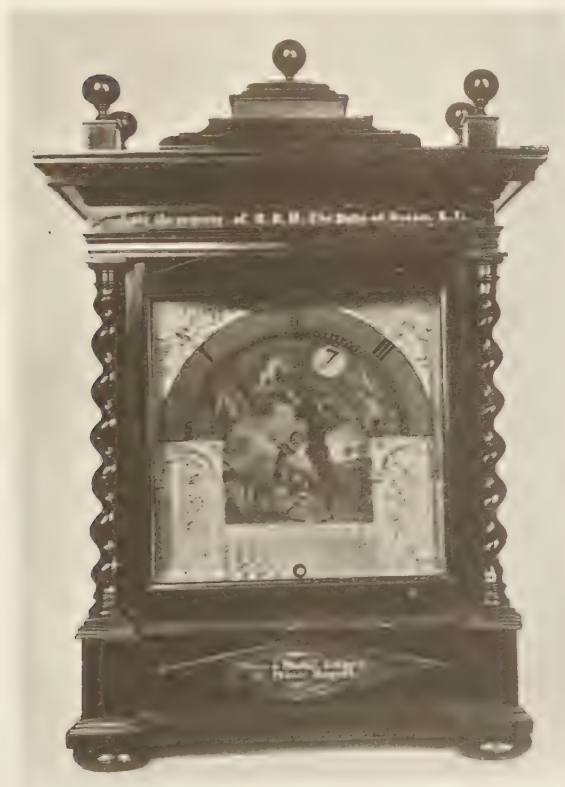
PLATE 55 Night clock by Joseph Knibb, circa 1670. A lamp inside the clock shines through the apertures in the dial plate. The fixed Roman numerals indicate the quarters, past which the arabic numerals move in succession. The time as illustrated is 7.38. (British Museum)
