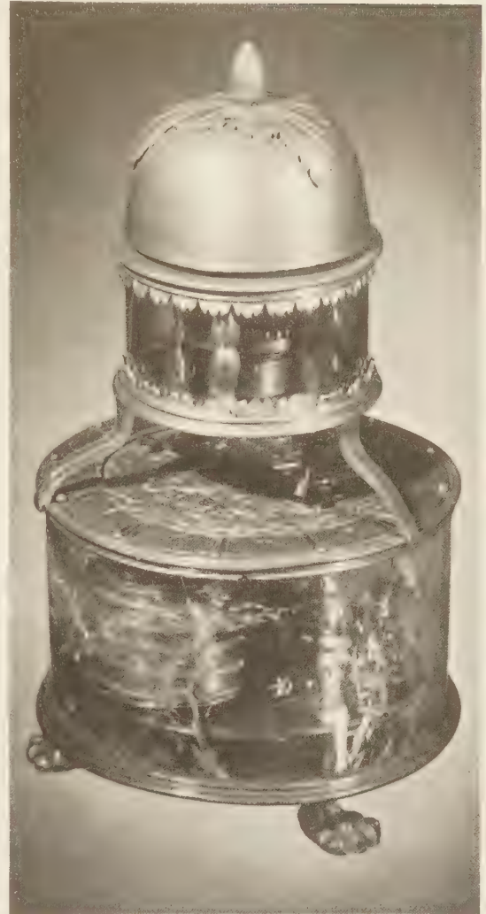
PLATE 12 Early type of spring-driven, drum-shaped table clock with separate detachable alarum mechanism on top of it. German, last quarter sixteenth century. Overall height 6 inches. Steel train. Note rock crystal sides to movement and alarum. Detent for alarum hanging down in path of the clock hand. (British Museum)
