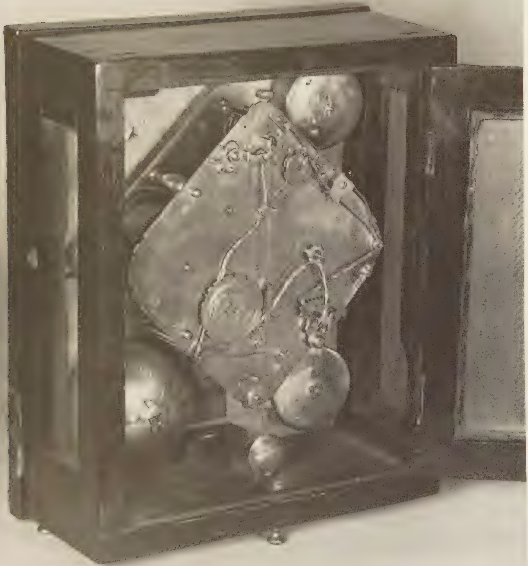
b mounted on a velvet ground. This clock is exceptional in that its striking system is a combination of lock-plate and rack striking, almost certainly prior in date to the invention of full rack striking in England in 1675. a dial, b back plate.
