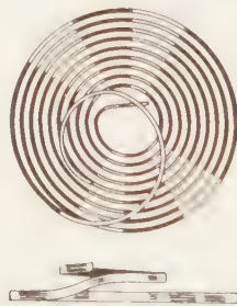
FIGURE 26. Breguet's spiral balance spring with overcoil.
