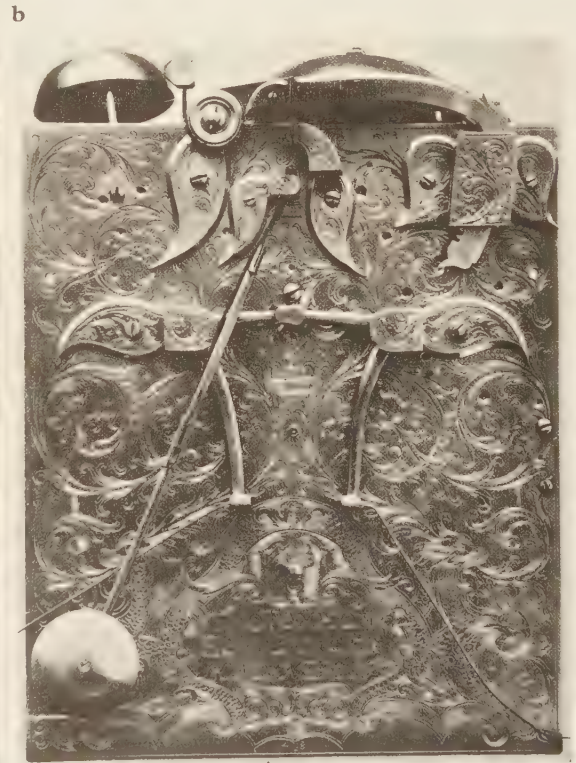
pattern fashionable until twenty-five years previously. Note (compared with plate 47) the spring-suspended pendulum with regulation effected from the subsidiary dial on dial plate; lenticular pendulum bob; absence of count wheel (owing to use of rack striking); operating levers for repeating mechanism. The oil sinks are later.
