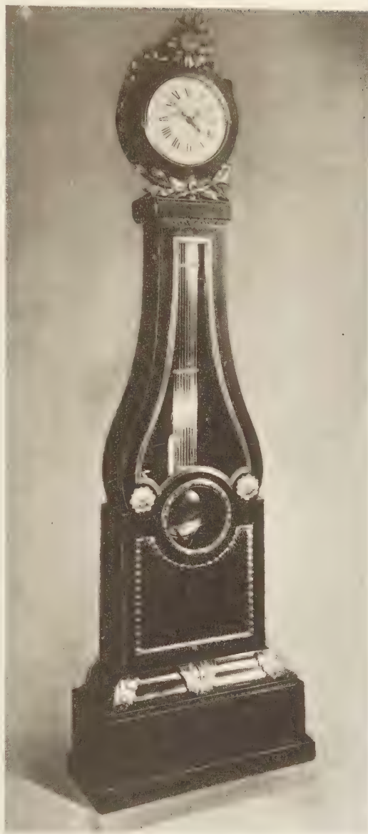
PLATE 170 Louis XVI Regulator by Lepaute, circa 1770. The case by Nicolas Petit. Pin-wheel escapement; gridiron pendulum; equation work. Note the brass-gilt decoration.
