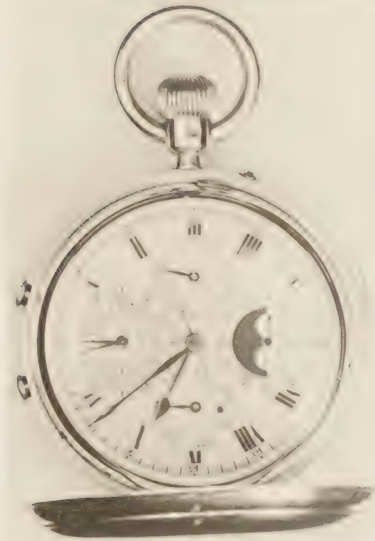
PLATE 149 Gold watch by S. Smith and Son, hallmarked 1899. This watch possesses most of the possible complications including perpetual calendar, minute repeating, and split-seconds chronograph. Hardly anything is visible of the movement, which is not therefore illustrated.
