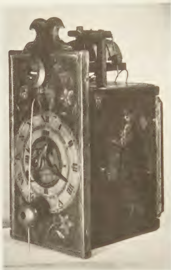
PLATE 198 Black Forest clock, circa 1740. An early example of the fully enclosed movement, two hands, striking train and pendulum. Note the typical arrangement of the pendulum hanging in front of the water-colour painted dial. The aperture above the XII may have contained an alternating sun and moon, now missing. Note also the archaic style of marking the quarters, and the fact that the minute hand is therefore shorter than the hour hand.
