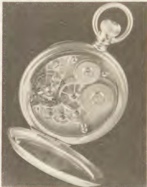
PLATE 153 Watch by the American Waltham Watch Company, circa 1900. The back plate of the movement, in which the wheels are pivoted, is made of rock crystal. Typical of the highest grade of American watch made to special order. a dial, b movement. (The Time Museum, Rockford, Illinois)
