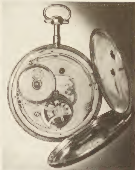
The movement b has the original type of Lepine's own calibre; virgule escapement; hallmarked 1789. (British Museum)
