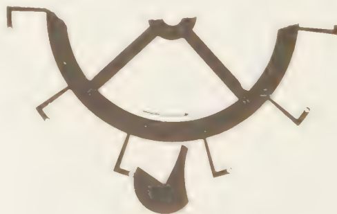
FIGURE 16. Tompion's experimental watch escapement. Pins (shown as white circles on the ends of the black teeth of the escape wheel) alternately rest on the rounded back of the balance staff roller, and impart impulse to its flat (or slightly curved) face. Impulse is in one direction only.
