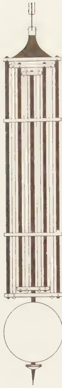
FIGURE 13. Harrison's gridiron pendulum. The five steel rods are black and the four brass rods are white.
