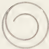
FIGURE 25. Arnold's helical balance spring with end-curves.
