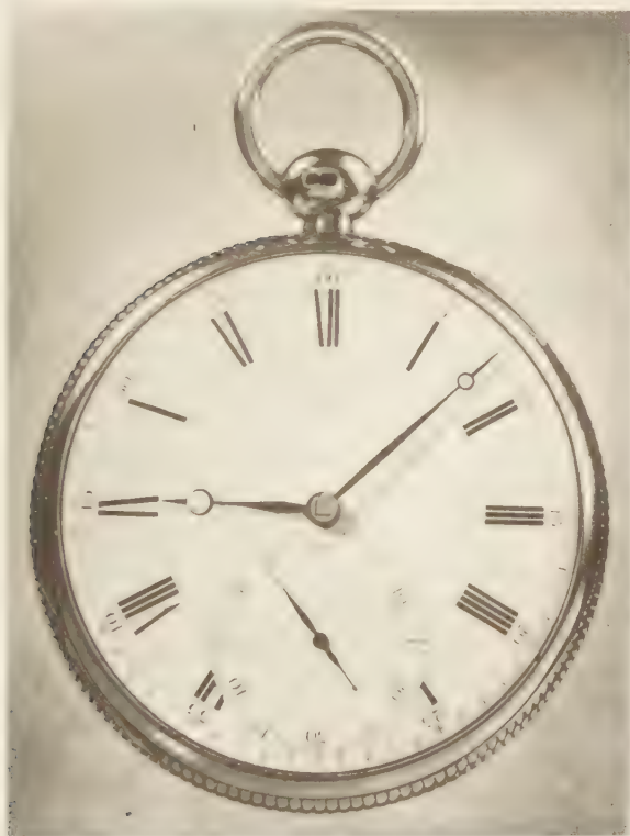
PLATE 127 Gold watch by James Ferguson Cole, hallmarked 1821. Note typical 1820 period English dial a ; superbly finished movement b with Lepine type of calibre, compensated balance and Cole's patented pivoted detent escapement. (British Museum)
