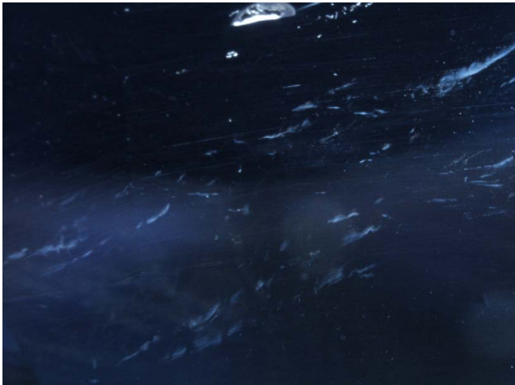
Figure 31: Near surface 'feathering', a feature often associated with heated sapphires, recorded in the he 55.88ct beryllium treated blue sapphire depicted in Figure 29.
