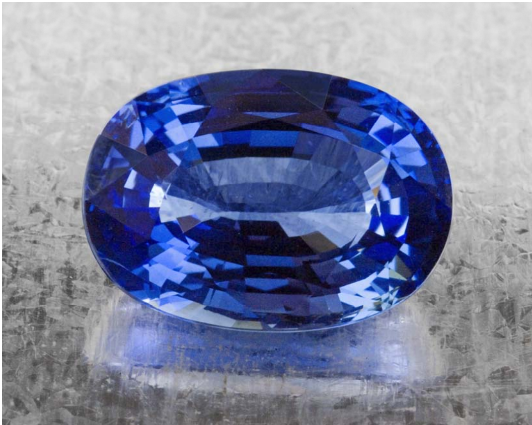
Figure 1: A blue sapphire recently examined in the laboratory weighing 22.52ct was determined to contain 7.50 - 9.50 ppma of beryllium by using LA-ICP-MS. Photo: Suchada Kittayachaiwattana © GIA
