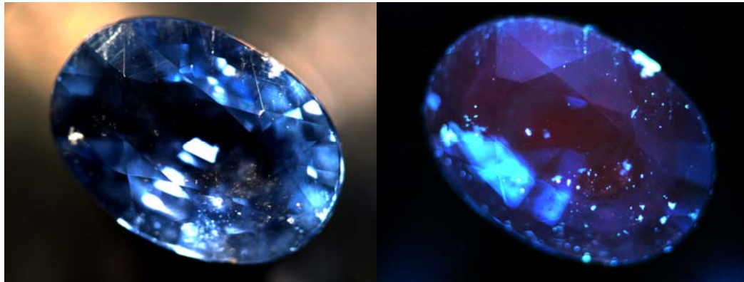
Figure 20: Stone number 5 (Figure 5) in normal light (left) and in the DiamondView™ (right)
