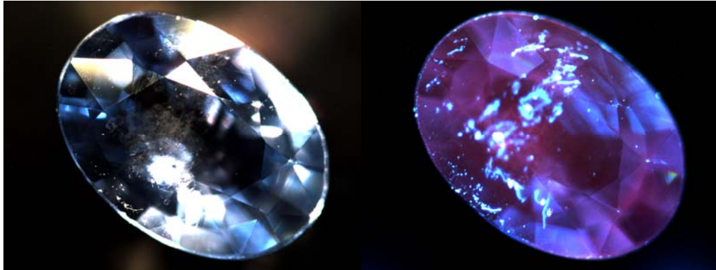
Figure 16: Stone number 1 (Figure 5) in normal light (left) and in the DiamondView™ (right)
