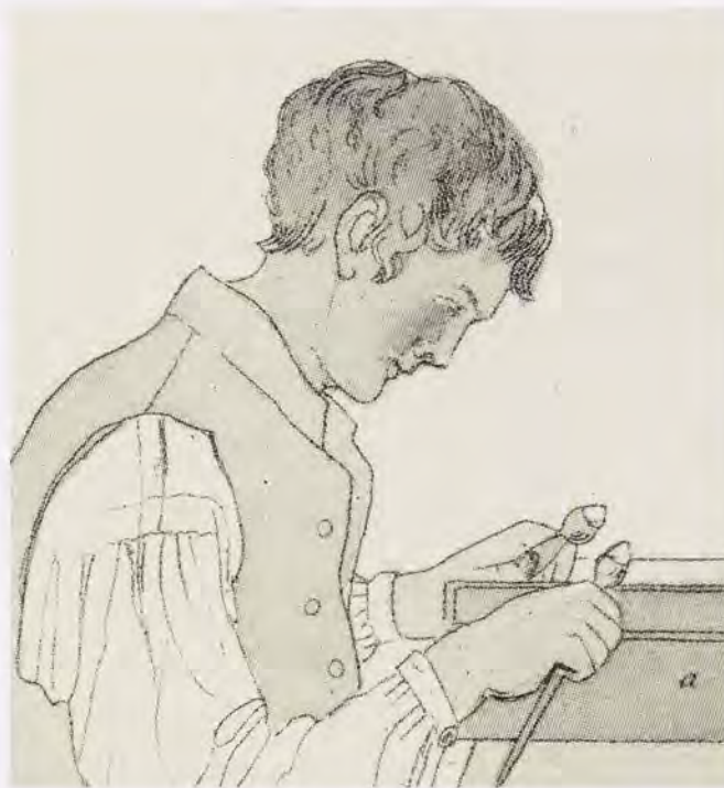
Fig. 2-8: A bruter rubs two diamonds against each other in order to form the shape or outer circumference of the diamond. The heading on this picture in Mawe's book is "Diamond Cutter," consistent with the British term for the act of bruting. Mawe, 1823, plate 1.
