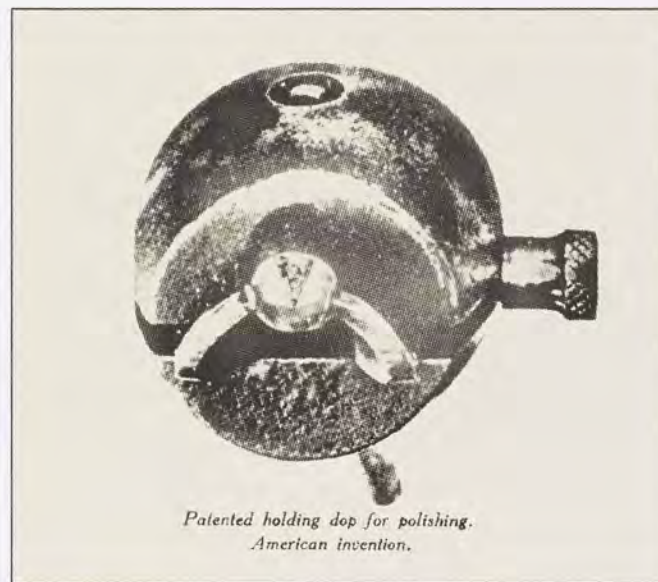
Fig. 3-1: Heat buildup during polishing sometimes softened the old-style lead dop (left), loosening its hold on the diamond. Stern Bros. & Co. developed a mechanical dop (right) in 1897 that held the diamond firmly no matter how much heat was generated during polishing. This allowed for greater polishing accuracy and consistency. Both photos from J. R. Wood & Sons, 1914.
