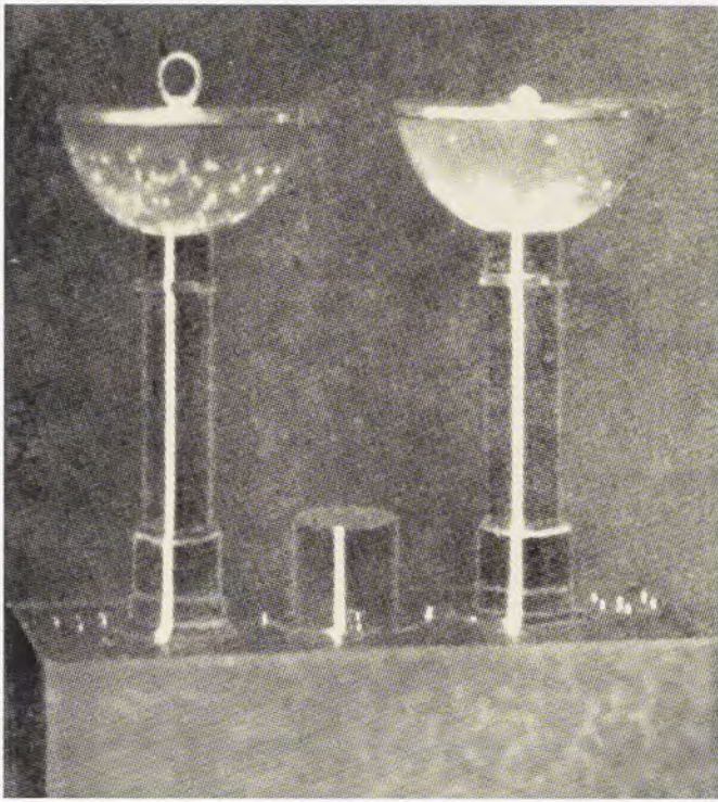
Fig. 5-15: Johnsen's Brilliantoscope. A diamond was placed in each of the two globes and their patterns were compared to determine which was better. Bauer, 1932, Table 14, figure 161.
