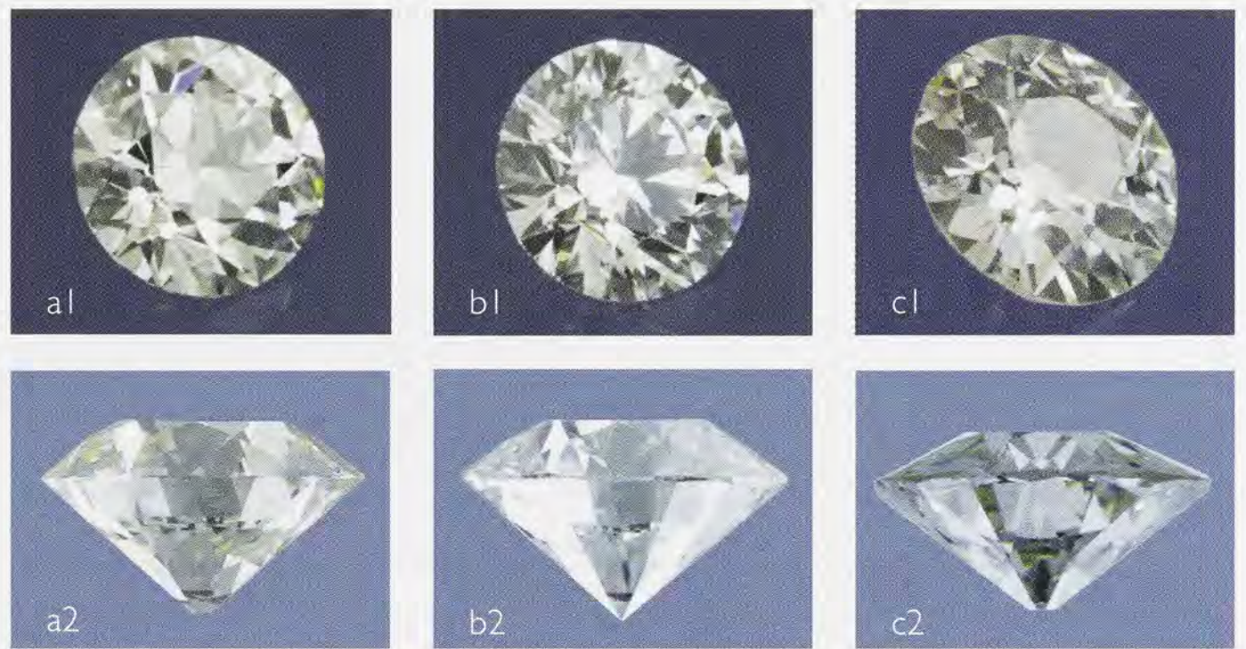
Fig. 5-4: The diamond on the left (a1, a2) was recently cut to the proportions proposed by Marcel Tolkowsky, including his shorter lower halves, large culet facet (by today's standards) and extremely thin girdle. Note that its pattern has a slightly blocky appearance compared to the diamond on the far right. The diamond in the center (b1, b2) is also cut to proportions close to Tolkowsky's, but with modern changes (no culet, a thicker girdle and longer lower girdle facets). The diamond on the far right (c1, c2) has a pavilion angle (40 degrees) and table size (40 percent) in the range of typical American cutting from 1870 through the 1930s. The shallow crown angle (27 degrees) demonstrates that cutters were trying to achieve the look of the period, but were probably cutting from shallow rough crystals to retain weight. Correctly cutting to the proportions of the American Cut for that period (with the slightly steeper crown angle), would have yielded a smaller diameter and less carat weight. Photos by Eric Welch (face-up) and Don Mengason (profile)/GIA.
