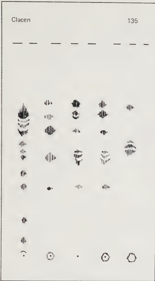
Figure 15.1 Typical results from thin-layer chromatography showing (from left to right): resin, gedanite, copal I, copal II, reduced amber (Rottländer, 1970).
