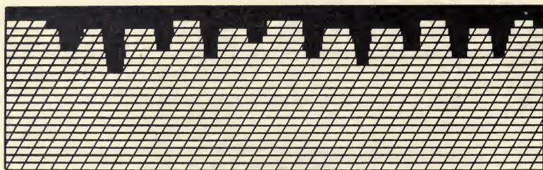
Diagrammatic Section of a Calcite Plate across the line of flow. The flowed material has completely filled up even the deepest scratches.
