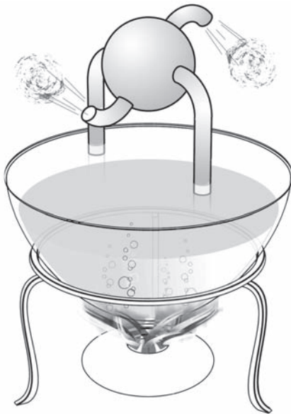
Figure 32: Hero's steam engine.
