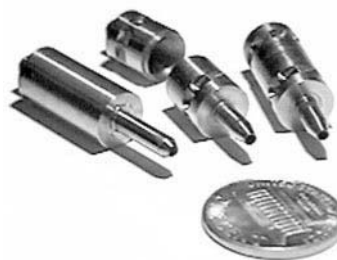
Figure 5 (See Colour Plate 108) Titanium belt driven and air driven rotors used in the arrayable flow-through centrifuge. A penny is shown for scale.
