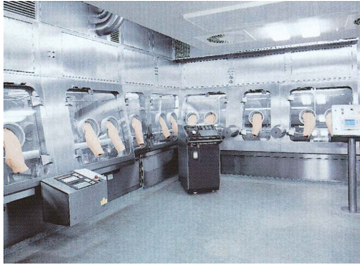
Plate 37 Distillation: Freeze-Drying Isolator, Class 100, for filling, transportation and loading of vials into the freeze-drying plant. Decontamination of the isolator and the equipment therein is accomplished by vaporized hydrogen peroxide (VHP). The VHP 100® generator can be seen in the centre in front of the isolator. (Courtesy of Steris GmbH, Hürth, Germany.)
