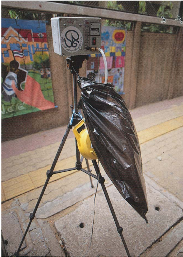
Plate 57 Atmospheric Analysis Air pollution monitor. The initial step of sample acquisition is a far from trivial task in atmospheric measurements. (Reproduced with permission from Eye Ubiquitous.)
