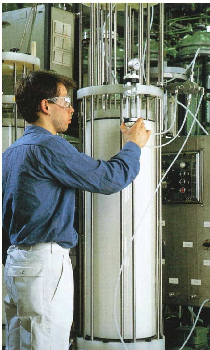
Plate 23 Chromatography: Liquid Large-Scale Liquid Chromatography. Scientist with column Chromatography equipment. Column Chromatography is used to separate the various components from a mixture of chemicals. During this process the mixture is put in the top of the column. The mixture passes through a porous substance, which selectively hinders the movement of each of the components. This means that some components will travel further in a given time than others, allowing each of them to be individually collected. Photograph of equipment used to isolate chemicals produced by microorganisms, including genetically engineered varieties. (With permission from Maximilian Stock Ltd / Science Photo Library).
