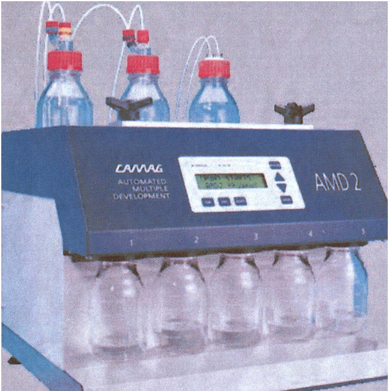
Plate 30 Chromatography: Thin-Layer (Planar) Camag automated multiple development chamber AMD 2.
