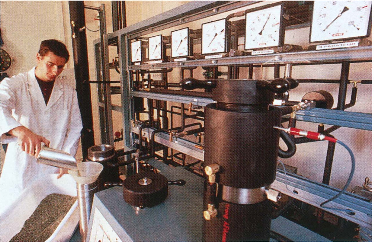
Plate 44 Extraction: Supercritical Fluid Extraction Extraction of taxol. A researcher loading a supercritical fluid extractor with crushed bark. The bark contains the anti-cancer drug taxol, and is from the Pacific Yew ( Taxus brevifolia ). Taxol has been shown to be effective in restricting various types of cancers, particularly of the breast, ovary, skin and colon. Laboratories are looking into ways of synthesising this natural drug, as the tree has become a protected species. Photographed at the institute for the Chemistry of Natural Substances (ICSN), Gif-sur-Yvette, France.
