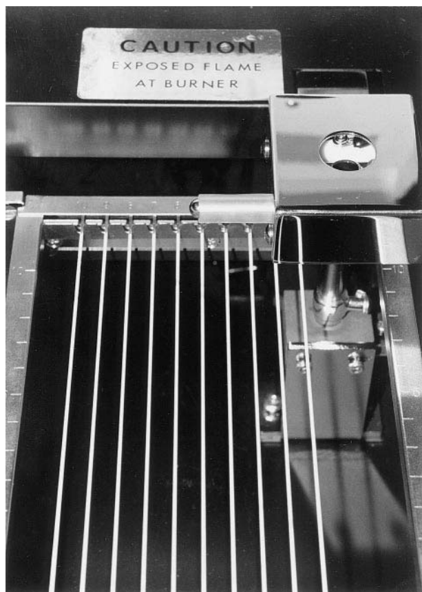
Figure 1 Top view of Mark V Iatroscan with horizontal rack holding 10 Chromarods in position for automatic scanning in the FID. The flame jet on the right is visible below the ion collector. The Chromarods pass between the two FID parts as the frame holding the development rack cycles for scanning. After each scan the frame moves sideways and returns between the Chromarods, bypassing the FID and moving sideways to start the next Chromarod. The right-hand rod is reflected in part of the ion collector.
