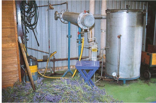
Plate 82 Essential Oils: Distillation Lavender oil is evaporated by steam in the still, condensed, and collected in a Florentine Flask. Jersey. (Reproduced with permission from Eye Ubiquitous.)
