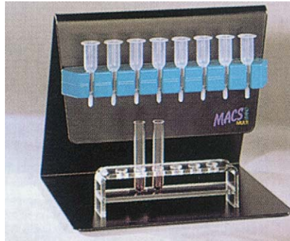
Plate 62 Biologically Active Compounds and Xenobiotics A typical example of laboratory-scale high gradient magnetic separators. OctoMACS Separator (Miltenyi Biotec, Germany) can be used for simultaneous isolation of mRNA. (Courtesy of Miltenyi Biotec, Germany.)
