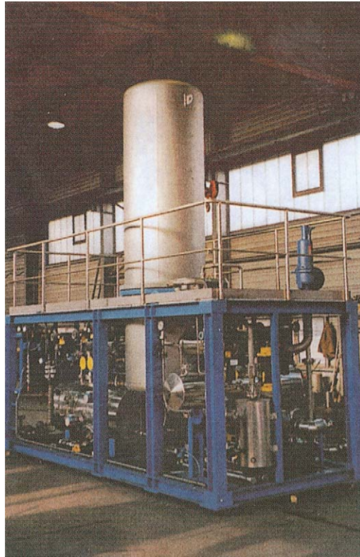
Plate 51 Membrane Separations: Pervaporation Vapour permeation unit for recovering ink solvent.
