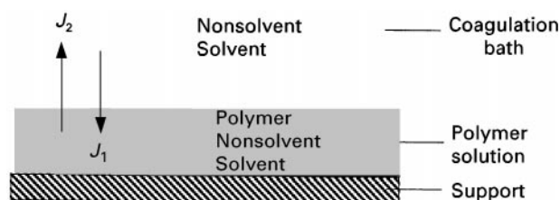
Figure 17 Schematic representation of a film–bath interface. Components: nonsolvent (1), solvent (2) and polymer (3). J_1 is the nonsolvent flux and J_2 the solvent flux.
