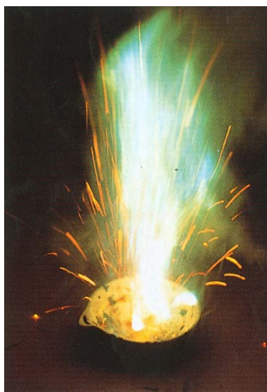
Plate 83 Explosives Ammonium nitrate burning. An explosion of flames leaps out of a dish containing burning ammonium nitrate ( \text{NH}_4\text{NO}_3 ). Ammonium nitrate is used in the manufacture of explosives and fertilisers. It was first used as an explosive by Alfred Nobel, founder of the Nobel Prize, who used it in his dynamite mixtures in 1875. Separations, particularly chromatographic, are important for the characterization of explosives, particularly in forensic contexts. (Reproduced with permission from Science Photo Library.)
