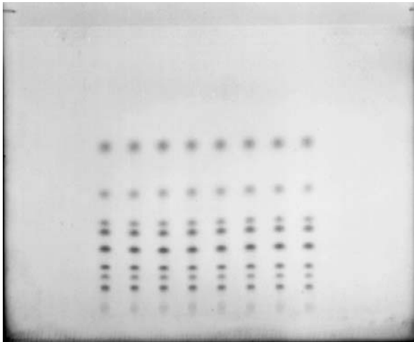
Figure 7 Video scan of separation of corticosteroids on an HPTLC silica gel plate. Detection reagent: blue tetrazolium solution. Spot application with automatic equipment.
