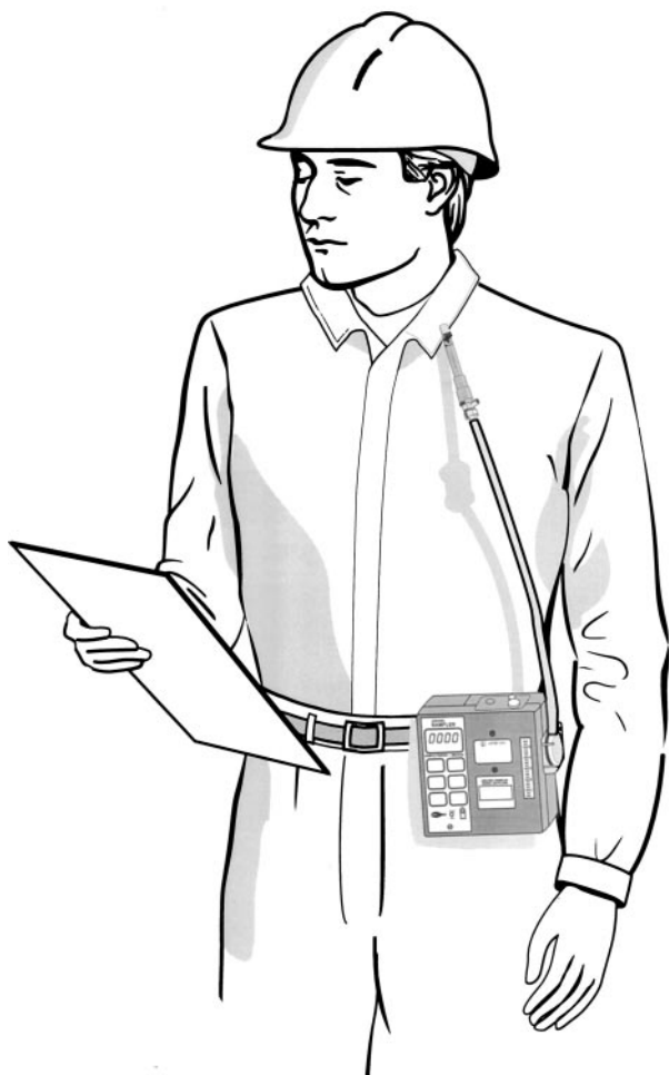
Figure 2 Personal air sampling train attached to a worker.
