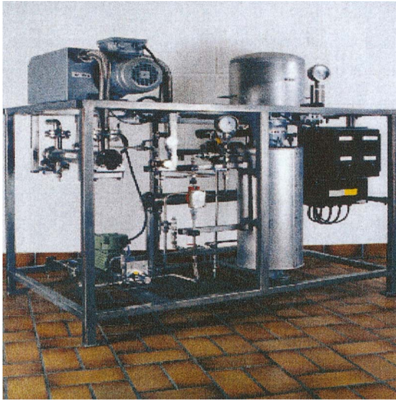
Plate 52 Membrane Separations: Pervaporation Standard unit for batch dehydration of rinse alcohol.
