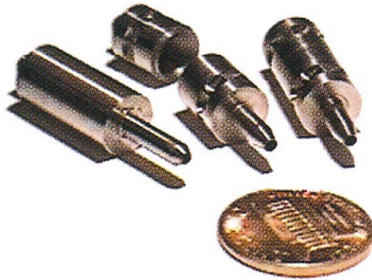
Plate 108 Centrifugation Titanium belt driven and air driven rotors used in the arrayable flow-through centrifuge. A penny is shown for scale.
