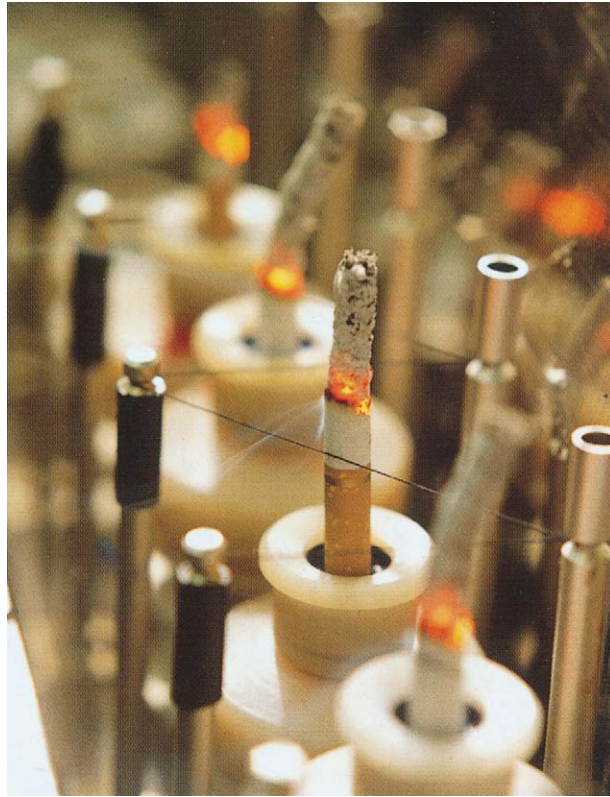
Plate 122 Tobacco Volatiles Cigarette testing. Cigarettes being tested for the nicotine and tar content of their smoke during either medical research or as part of quality control in the tobacco industry. The cigarettes are being held vertically and having air sucked through them into the tubes in which their butts (brown) have been placed. The air will be analysed for its tar and nicotine content. Nicotine acts as a stimulant on the central nervous system and is the chemical that causes cigarette addiction. The tar is one of the numerous toxic by-products released by the burning of the cigarette. (With permission from Science Photo Library.)
