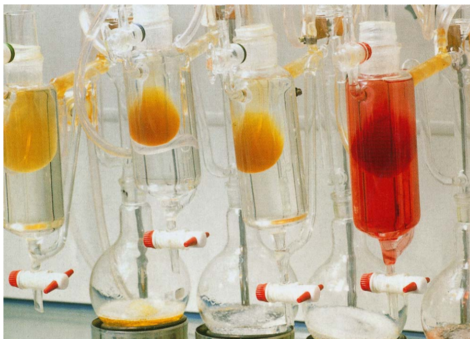
Plate 48 Membrane Separations: Diffusion Dialysis Chemical dialysis. Glassware used for purifying solutions by separating them from colloid chemicals using dialysis. During dialysis an impure solution is placed in a semi-permeable membrane (spheres) which is immersed in a pure solvent. Some of the chemicals within the membrane may pass out into the solvent by diffusion. The chemicals that remain trapped within the membrane are called colloids . Colloids usually consist of large molecules & tiny particles, although their exact composition depends upon the nature of the membrane. (Reproduced with permission from Science Photo Library.)
