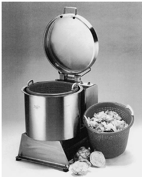
Figure 8 Small industrial-scale centrifuge for dewatering fresh-cut produce. The machine is operated in batch mode, but use of insertable plastic bowl minimizes down time between loads. Reproduced with permission from Freshline Machines, Sydney, Australia.
