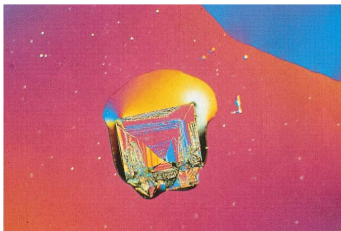
Plate 67 Chiral Separations: Crystallization Crystallization remains an important method for the resolution and purification of enantiomers, as first used by Pasteur for D and I tartaric acid. (Reproduced with permission from Science Photo Library.)
