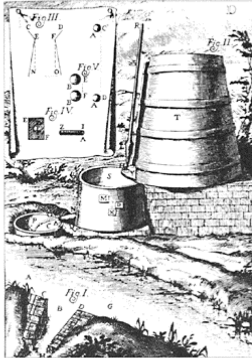
Poleni's apparatus to study the efflux of water from conical mouthpieces that modeled the entrance mouth of a flood relief channel. From G. Poleni, De castellis (1718).
