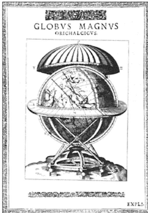
Tycho Brahe's brass celestial globe was about five feet in diameter. From Brahe's Astronomiae instauratae mechanica (1598).
