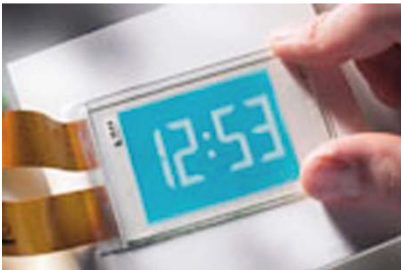
Electrowetting and Droplets, Figure 2 Electrowetting-based cyan display with 160 pixels/inch (courtesy of LiquaVista)
