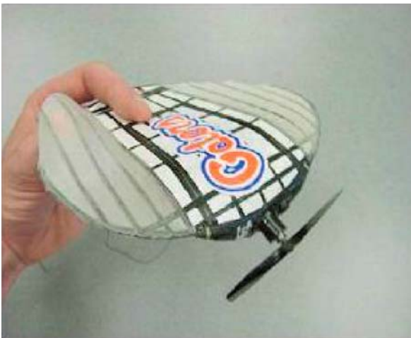
Micro Aerial Vehicles, Figure 3 MAV prototype built and flown by University of Florida research group [5]
