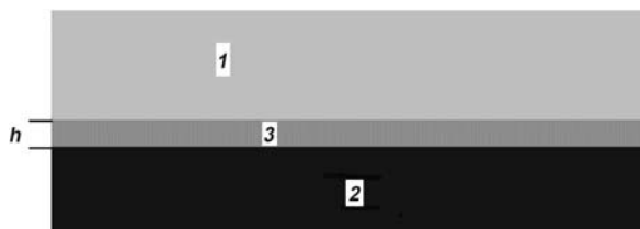
Disjoining Pressure, Figure 2 Interaction between two thick plates 1 and 2, possibly made of different materials, with a thin layer, 3, in between
