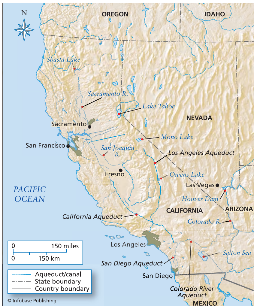
Map of California showing the locations of the aqueducts bringing water from the mountains of the Sierra Nevada and from Mono Lake to water-thirsty Los Angeles
