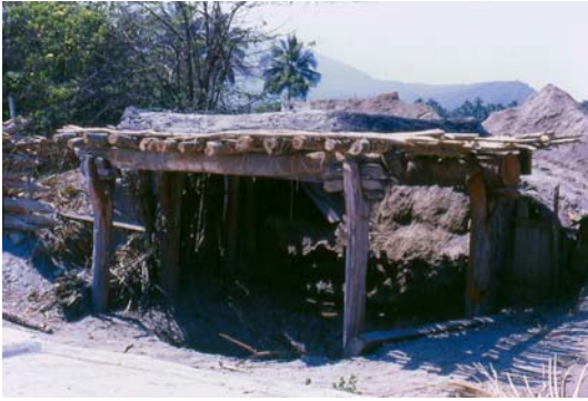
Salt Production in Mesoamerica. Fig. 4 Filtering device known as tapeixtle , used on the coast of Michoacán for leaching estuary water to produce brine (© Eduardo Williams).
