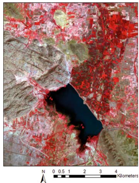
Water Management and Reservoirs in India and Sri Lanka. Fig. 8 ASTER satellite image of the Daroji reservoir first built in the sixteenth century, south of Vijayanagara. Notice the strong growth of agricultural crops indicated by the reflection of near-infrared wavelengths (shown here in red) downstream from the embankment. Vegetation growth is also occurring on the edges of the reservoir as receding water exposes moisture retaining sediments (data originally obtained from NASA).
