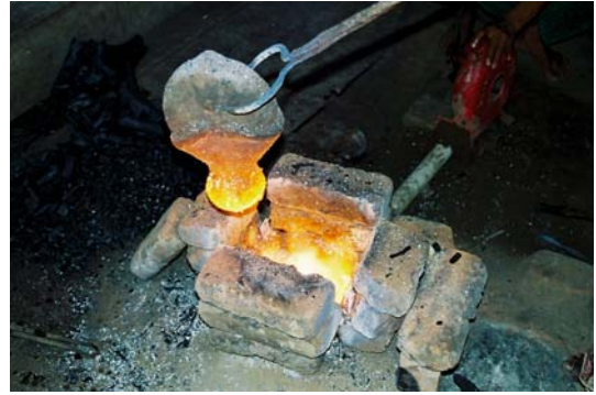
Mirrors: Metal Mirrors from India. Fig. 4 Heated inverted crucible-cum-mould being removed from hearth with the lower part containing the metal to be cast. When the jug-shaped crucible-cum-mould is tipped over the molten metal flows into a narrow hollow space for the blank created by two flat disc moulds.
