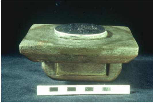
Mirrors: Metal Mirrors from India. Fig. 2 Cast oval mirror blank of silvery delta bronze mounted on wooden polishing board.
