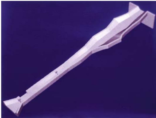
Water Management in Peru. Fig. 9 FLOW-3D computer model of the excavated hydraulic control section upstream of the chute and Hoya Hondada aqueduct from measured field data. Note the presence of the side overflow weir. Photo by C. R. Ortloff.
