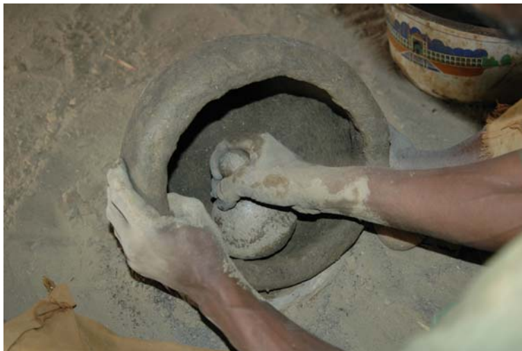
Ceramics in Africa. Fig. 2 Shaping a vessel with the pounding technique, on a concave wooden anvil with a clay tamper (photo by Olivier Gosselain).
