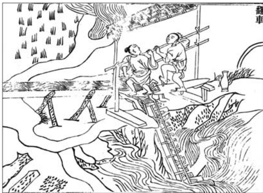
Agriculture in China. Fig. 7 Chain pump operated by two men. These light, portable pumps could be made quite easily by local carpenters and they would be moved from field to field as each needed irrigating or draining. Wang Zhen, Nongshu 19/7a–b.
