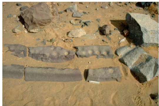
Mining in Ancient Egypt and Nubia. Fig. 19 Remains of a circular heavy mineral concentrator from Daghbag gold mine, Eastern Desert, Egypt, introduced during Ptolemaic times into Egyptian gold ore processing, but originally designed in the Laurion district, Attica, Greece.
