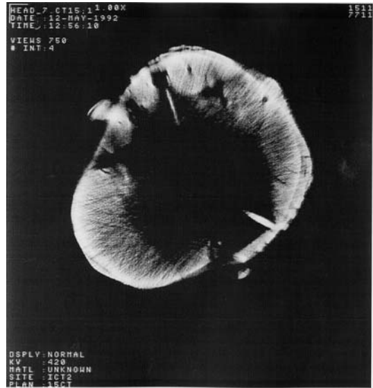
Metallurgy: Early Metallurgy in Mesopotamia. Fig. 23 Horizontal computed tomography cross section through the Head of a Ruler showing core supports (Photo: The Metropolitan Museum of Art, New York).
