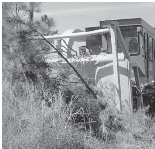
biofuel A biomass fuel machine known as “Jaws” harvests forest waste materials to be processed and used as fuel.
