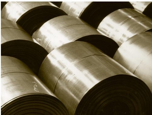
cold-rolling Tons of coiled cold-rolled steel stored in preparation for processing into tin-plated steel.
