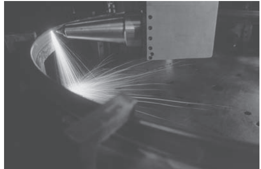
laser Laser beam employed in the process of manufacturing a jet engine part.
