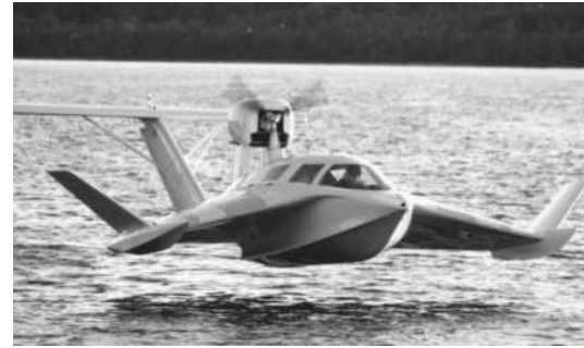
Fig. 2. Wing-in-ground-effect craft used over water as a commuter vehicle. (FlareCRAFT Corp.)
