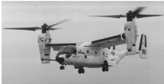
Fig. 2. Bell-Boeing V-22 Osprey tilt-rotor aircraft. (Bell Helicopter Textron)
