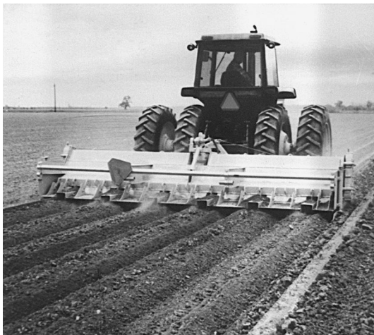
Multipurpose machine used for precision tillage, planting, bed shaping, and fertilizing in one pass, and for later bed shaping, cultivating, and fertilizing. (Johnson Farm Machinery Co.)
