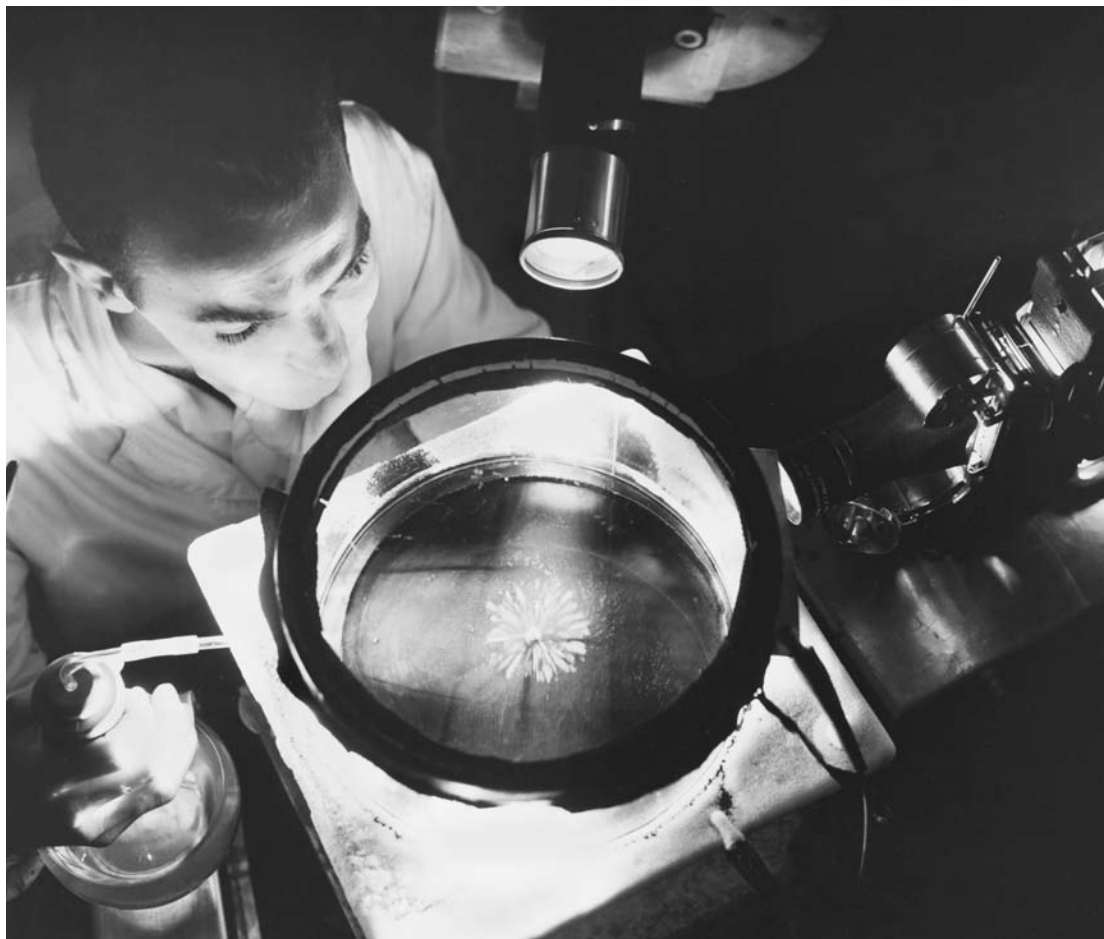
Scottish physicist Charles Thomson Rees Wilson invents the cloud chamber, which is used to study charged particles. In this photograph, physicists use the cloud chamber to study alpha particles. (Bill Bowles/NASA)
