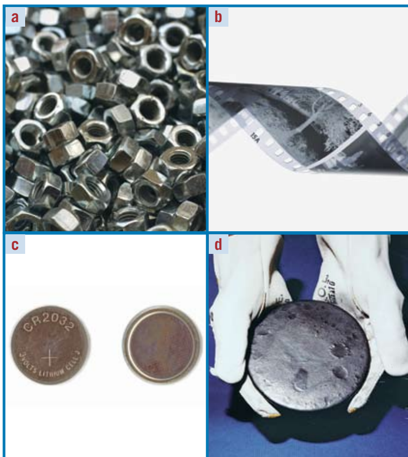
Figure 6.2 Metals are used in a variety of applications: (a) zinc nuts; (b) photographic film; (c) a lithium battery; (d) a piece of uranium called a billet.
