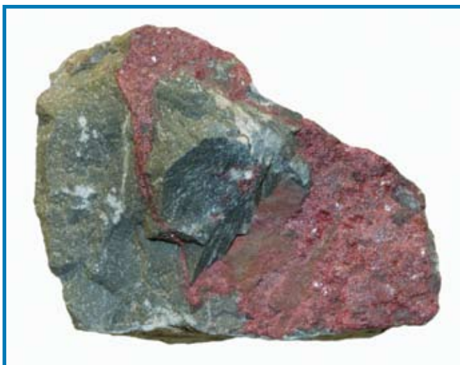
Figure 4.6 This is a sample of the ore cinnabar (vermillion). Cinnabar contains high concentrations of mercury sulfide and is the chief ore from which mercury is extracted.
