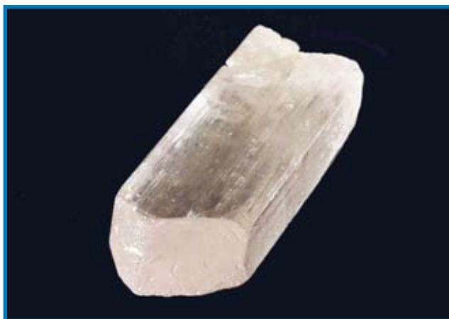
Figure 2.3 Lithium chloride can be extracted from the mineral spodumene ( \text{LiAlSi}_2\text{O}_6 ). Lithium can then be isolated from lithium chloride.
