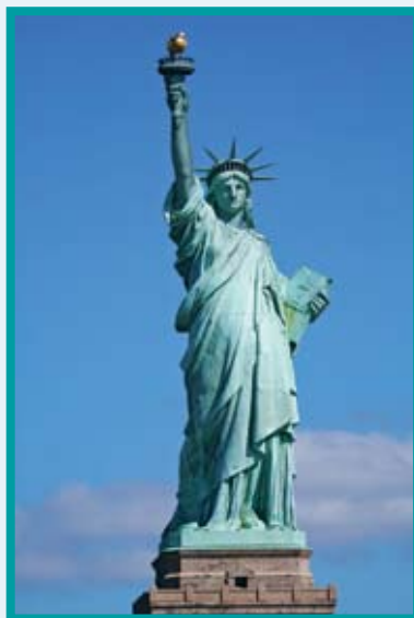
Figure 4.5 The Statue of Liberty has a copper skin that has oxidized to a greenish color.
