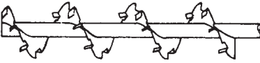
(c) Cut and folded screw flight. Continual lifting and tumbling of the material by the folded flights improves aeration and promotes mixing
