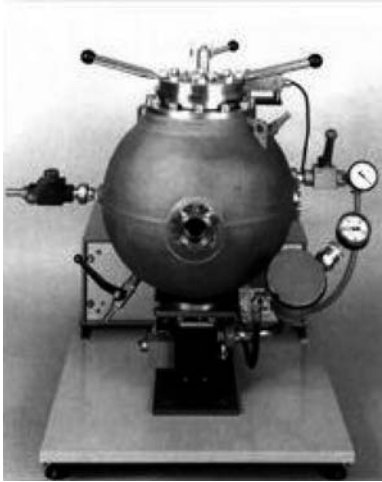
Figure 4-66 Kuhner 20-liter sphere (from Kuhner with permission).
