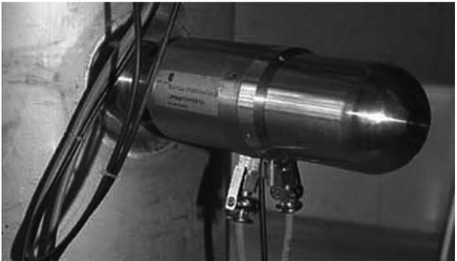
Figure 2-16 Fiber optic measuring instrument: “Labasys® Control Ex” for inline monitoring of dust concentration, velocity and flow rate. (From MSE Meili, Zurich, www.msemeili.ch , with permission.)
