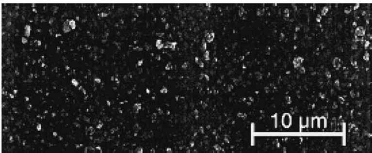
Figure 2-12 Abrasion-generated debris particles (From Repehagen and Werther, "Catalyst Attrition in Cyclones," Powder Technology , 113:55–69, 2000.)
