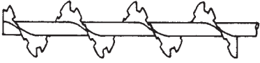
(b) Cut screw flighting. Used for conveying, cooling and moderately mixing materials, simultaneously
