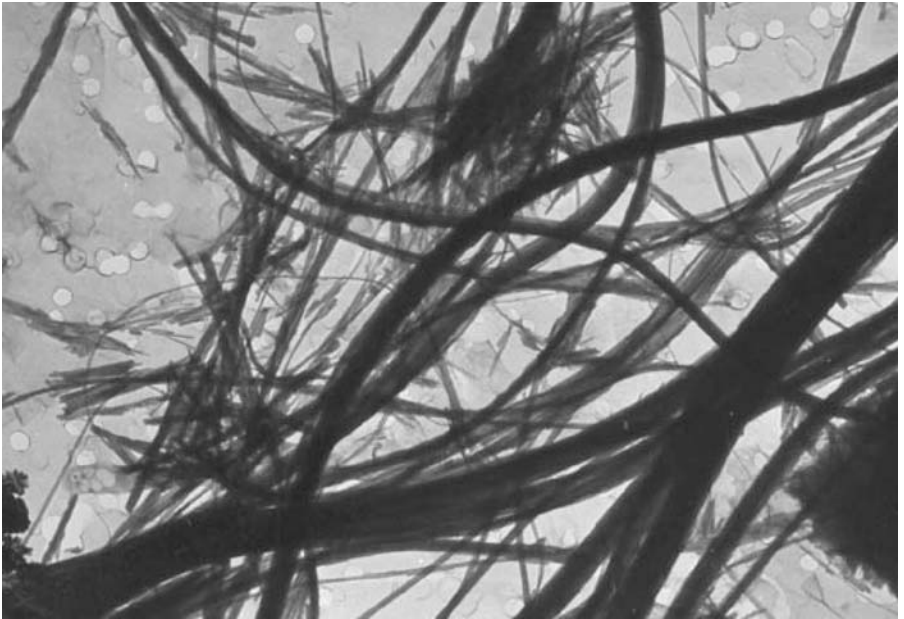
Figure 2-5 Friable asbestos fibers (from Fuller.com).
