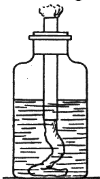
Fig. 10.—A Simple Alcohol Burner for the Laboratory.
