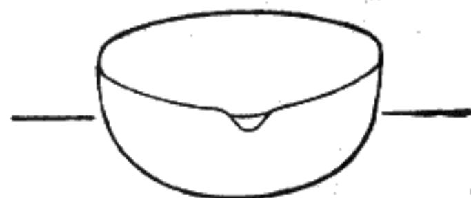
Fig. 17.—An Evaporating Dish Which is Generally Used for Boiling Purposes.
