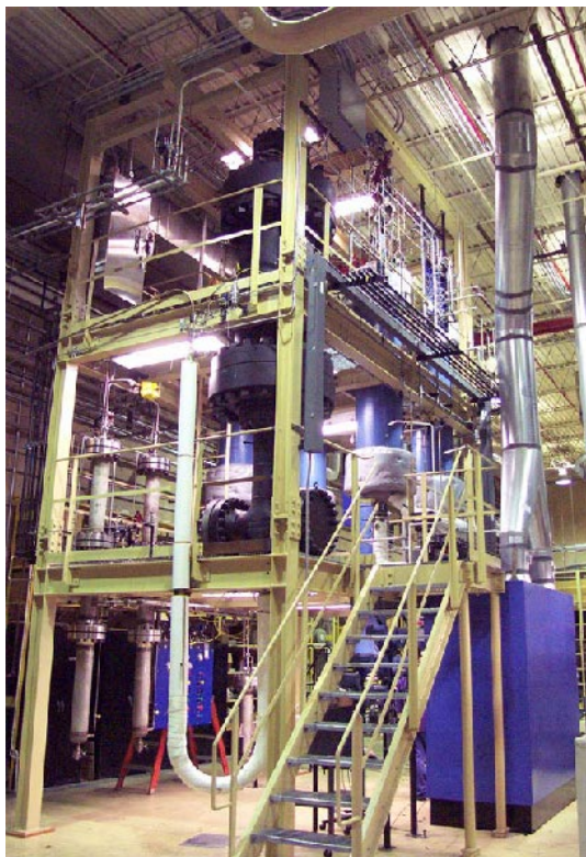
Figure 2. The setup at CNI for large scale production of SWNTs. Picture provide by CNI.
