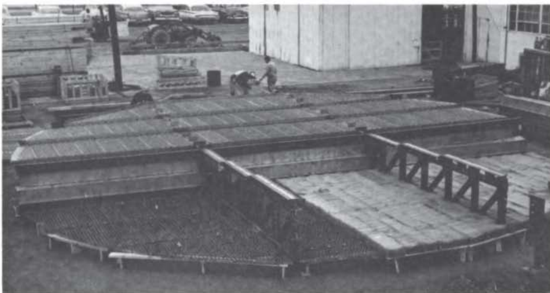
Figure 12-12 Assembly of a 12-m-diameter cascade tray containing ballast, or valve caps. The bottom portion of the plate, grid and matting, is a mist eliminator to remove entrainment from the vapors rising from below. ( Fritz W. Glitsch & Sons, Inc., Dallas, Texas. )
