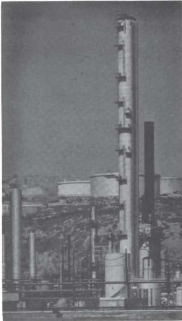
Figure 14-3 A xylene splitter column at the Richmond, California, refinery of Standard Oil Company of California. This column takes m - and p -xylenes as distillate and o -xylene as bottoms. Notice the large size compared with other columns. (Chevron Research Company, Richmond, California.)
