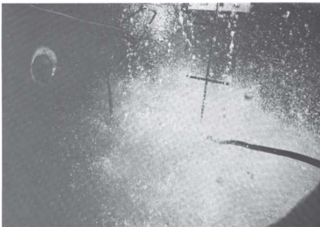
Figure 12-8 A view of typical vapor-liquid contacting on a sieve tray. ( Fractionation Research, Inc., South Pasadena, California. )
