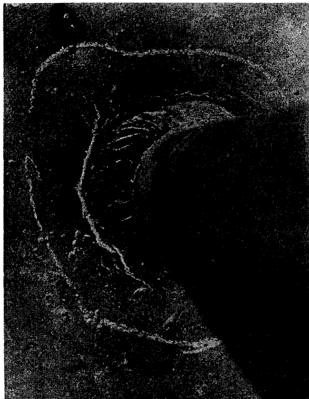
Fig. 16-56. Magnetic-particle indications revealing stress-corrosion cracks adjacent to weld joining 2-in. drain nozzle to bottom head of absorber. (Garwood, 16-42. Courtesy Phillips Petroleum Co. and NGAA.)
