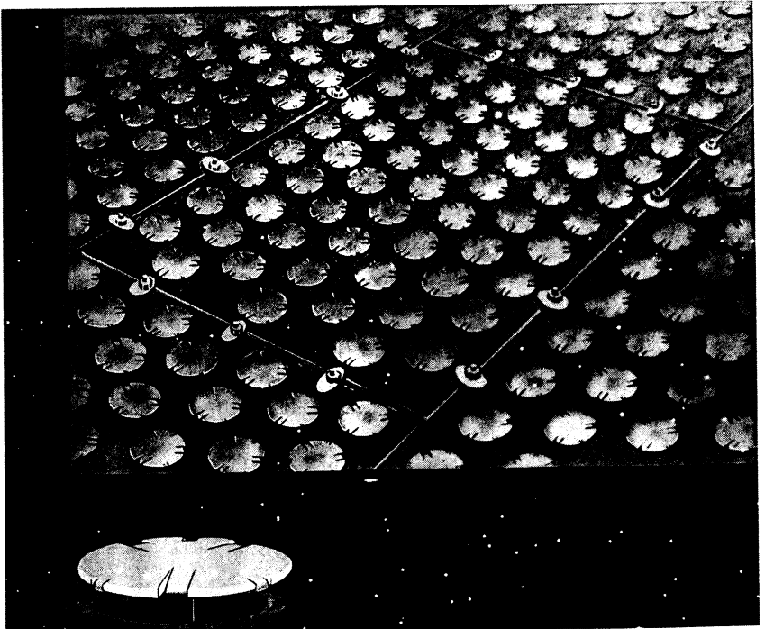
Figure 1-3 Portion of a Glitsch V-1 ballast tray. (By courtesy of Glitsch, Inc.)
