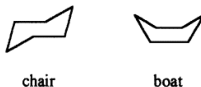
Figure 3.13. Chair and boat conformations of cyclohexane
