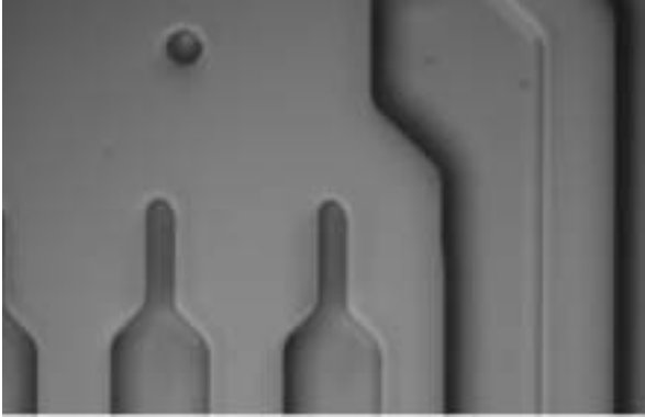
Fig. 7. Microscopic views of etched structures, before sputtering.
