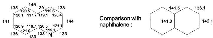
Fig. 6.11 Bond parameters of quinoline (bond lengths in pm, bond angles in degrees)
