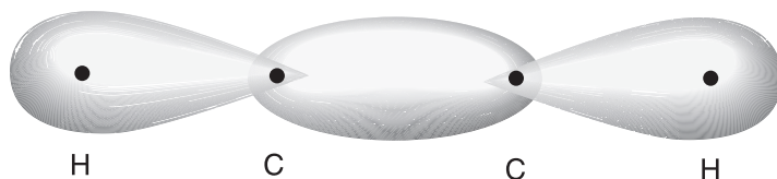
Fig. 1.6. The \sigma electrons of acetylene.
