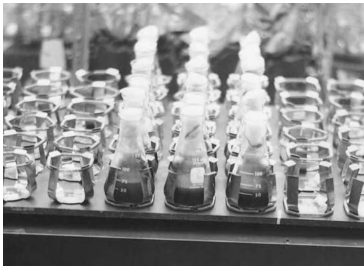
Figure 8.1 Example of a flask algal toxicity test conducted on an oscillator shaker.
