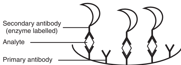
Figure 12.6 Representation of sandwich ELISA microplate well after its second washing. Note that the amount of enzyme on the plate is proportional to the amount of analyte present.
