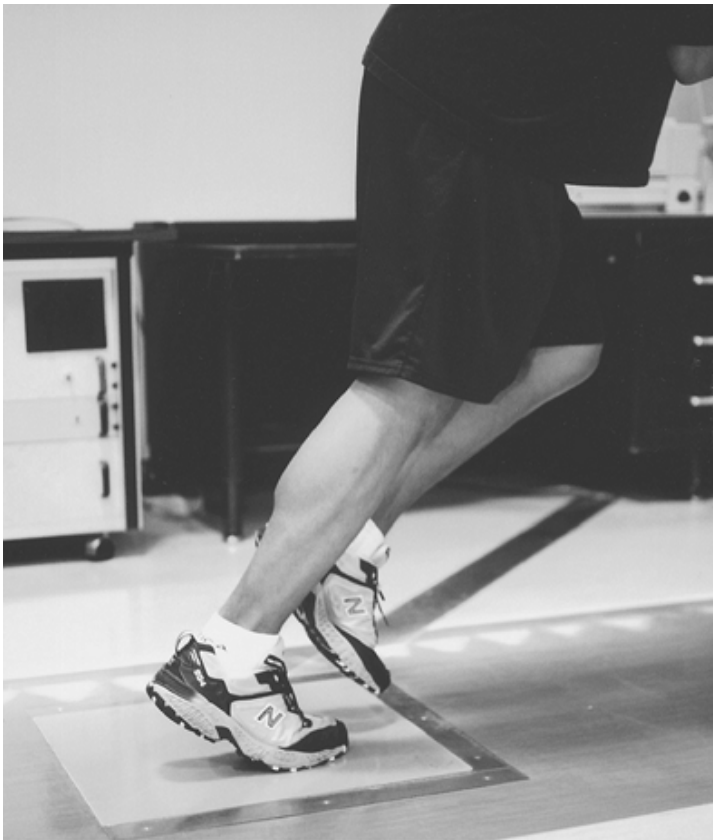
FIGURE 10-5 A typical laboratory force platform setup.
