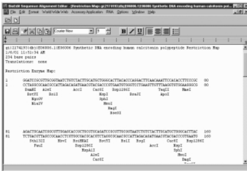
Figure 9.7. Restriction map generated with BioEdit. Synthetic DNA encoding human calcitonin is subjected to restriction with all REBASE restriction endonucleases to generate restriction map.
