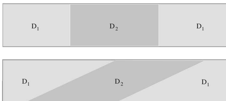
Figure 1.17. Two kinds of mean phase boundaries of a two dye, D_1 and D_2 , sandwich system. The phase boundaries are sorted according to their distance from the front and back.
